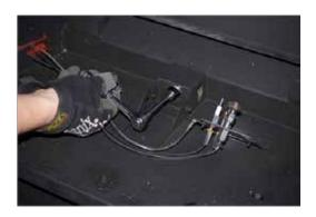
9) Remove pilot retainer clip with pliers and pull off the pilot cap to expose the pilot orifice.
