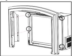
4. Install the safety screen into the inner Vignette frame with spacer by slightly tilting the safety screen frame and placing it up into the Vignette frame. Let the safety screen slightly drop down into position within the Vignette frame.
