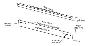
Similar to the front hearth trim, cut the top of the bottom piece of the spacer brackets to the appropriate height.
