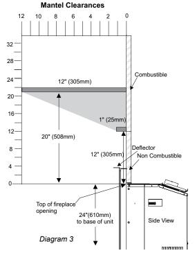
Note: A 3-1/2" mantel deflector to reduce mantel height to 36" from bottom of unit @ 1"depth.
