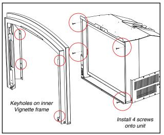
3. Install the inner Vignette frame by hanging the frame off the 4 screws via the keyhole openings on the frame. When in position, tighten the 4 screws.
