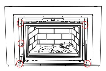
3. Separate the Outer Faceplate from the Backing Plate by removing 7 screws.
