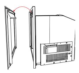
2. Remove 4 screws from the back of the Vignette faceplate in locations shown below—to remove the safety screen assembly.
