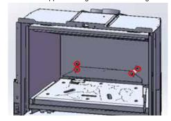
A top bracket must be installed prior to installing the log set.
