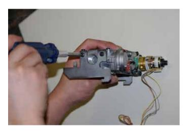
**11)** There is a provision in the Valve body casting that is designed to be used as a gripping point for assembly with other components. This is the portion of the valve that can be placed in a machine vice.
