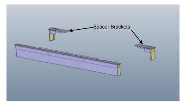
4) Attach the top and bottom part of the spacer brackets and then attach these spacer brackets to the assembled hearth trim with 3 screws.
