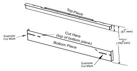
3. Reattach the top piece of the hearth trim to the cut bottom piece by fitting in place.
