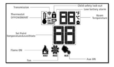
Figure 2: Transmitter LCD Display
