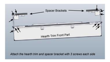
5) Secure the hearth trim with a clip on its side to keep it steady as shown in the diagram below.
