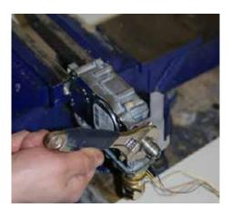
**13)** Remove the 2 screws that secure the left side valve mounting bracket from the gas valve.
