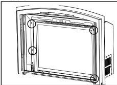
4. Install the safety screen into the inner Vignette frame by slightly tilting the safety screen frame and placing it up into the Vignette frame. Let the safety screen slightly drop down into position within the Vignette frame.
