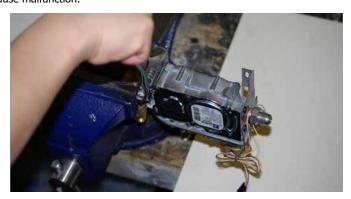
10) Remove the 2 screws that hold the Right Side Valve Mounting Bracket onto the Valve.
