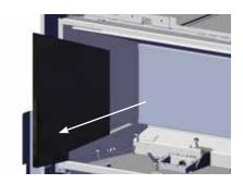
2) Lift the Burner slightly while pulling forward to clear the mixing tube.
