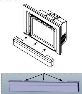
Align hearth trim to base of the unit and secure it with 3 screws
