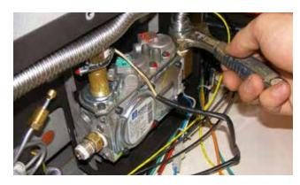
**7**) Remove both Screws that secure the Gas Valve Mounting brackets, both sides.
