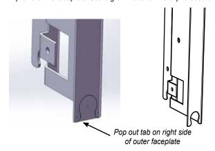
Install the vignette faceplate by hooking the flange over the hanger as shown below.
