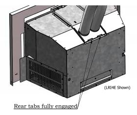
Properly installed Flue Connector Plate
