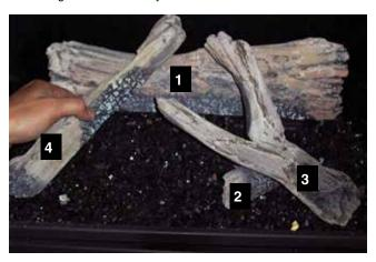
Line up pin locator and pin, Logs 1,4
