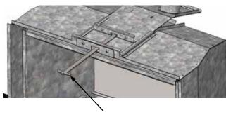
Flue Connector Slide Tool
