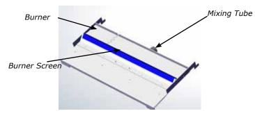
3) Remove the 2 screws as shown. Lift the burner with both hands.
