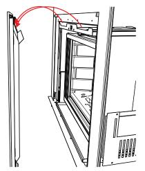
2. Remove the outer faceplate by removing the 5 screws as shown.
