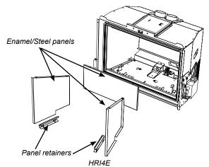
\*Insulation panels not shown in this diagram
