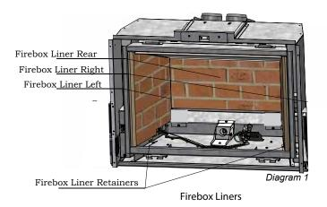
If installed, remove black metal left and right side inner panels by sliding them forward - see below. Discard panels after removal.
