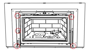
Attach the backing plate to the outer faceplate from the front with 7 screws (3 along the top and 2 on each side).
