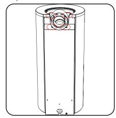
3. Line up the flue collar with the screw holes in the unit and replace the 4 screws removed in Step 2. Reinstall the centre cast piece.
