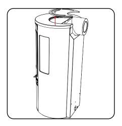
2. Remove 4 screws securing flue collar and turn flue collar 180°.
