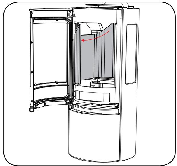
11. Reinstall top heat baffle and secure both enamel panel and baffle with screws loosened in Step 3.
