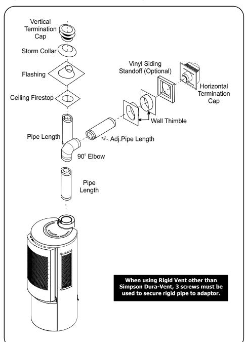
The FPI AstroCap™ and FPI Riser Vent terminal are certified for installations using FPI venting systems as well as Simpson Dura-Vent® Direct Vent, American Metal Products Ameri Vent Direct Vent, Security Secure Vent®, Selkirk Direct-Temp, Olympia Ventis, and ICC Excel. AstroCap™ is a proprietary trademark of FPI Fireplace Products International Ltd. Dura-Vent® and Direct Vent Pro are registered and/or proprietary trademarks of Simpson Dura-Vent Co. Inc.
