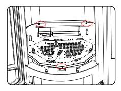
Loosen both screws on pilot hood cover. Pivot cover to the left to reveal pilot hood.
