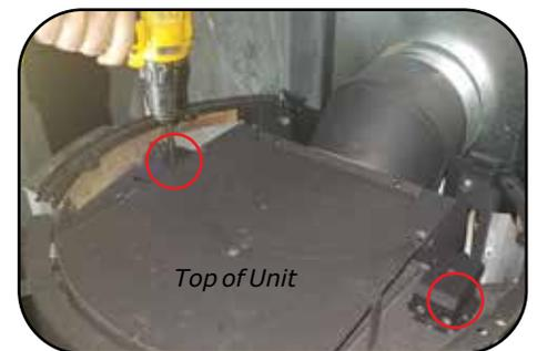
4. Remove 2 screws to release each bulb housing.
