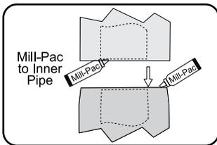
**NOTE: For best results and optimum performance with each approved venting system, it is highly recommended to apply "Mill-Pac" sealant (supplied) to every inner pipe connection. Failure to do so may result in drafting or performance issues not covered under warranty.**
