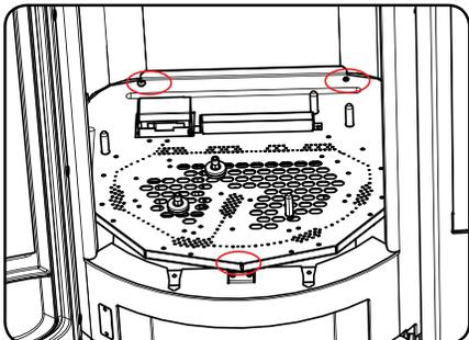
6. Loosen both screws on pilot hood cover. Pivot cover to the left to reveal pilot hood.
