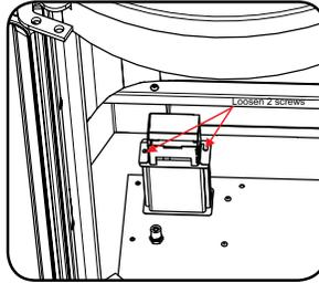
7. Lift off pilot cap to expose pilot orifice.
