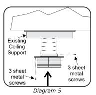
7. The connection between the appliance and the Retro Connector may be completed with sections of black direct vent pipe, together with an adjustable length.
