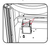
Lift off pilot cap to expose pilot orifice.
