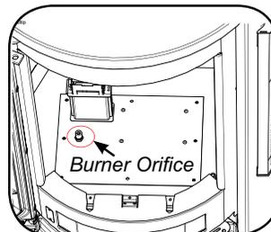
10. Reinstall new burner orifice LP stamped #54 and tighten.
