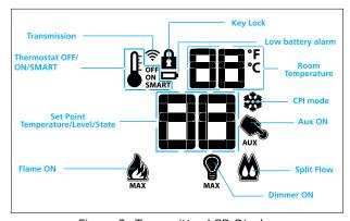
Figure 2: Transmitter LCD Display
