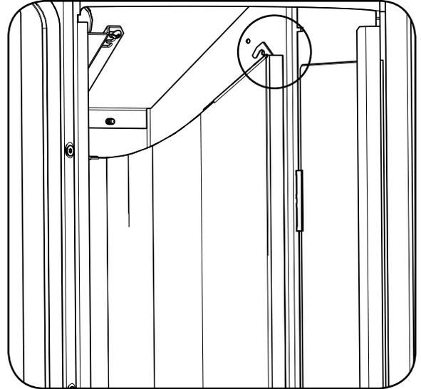
9. Lift panel up off the screw and rotate to remove from the unit.
