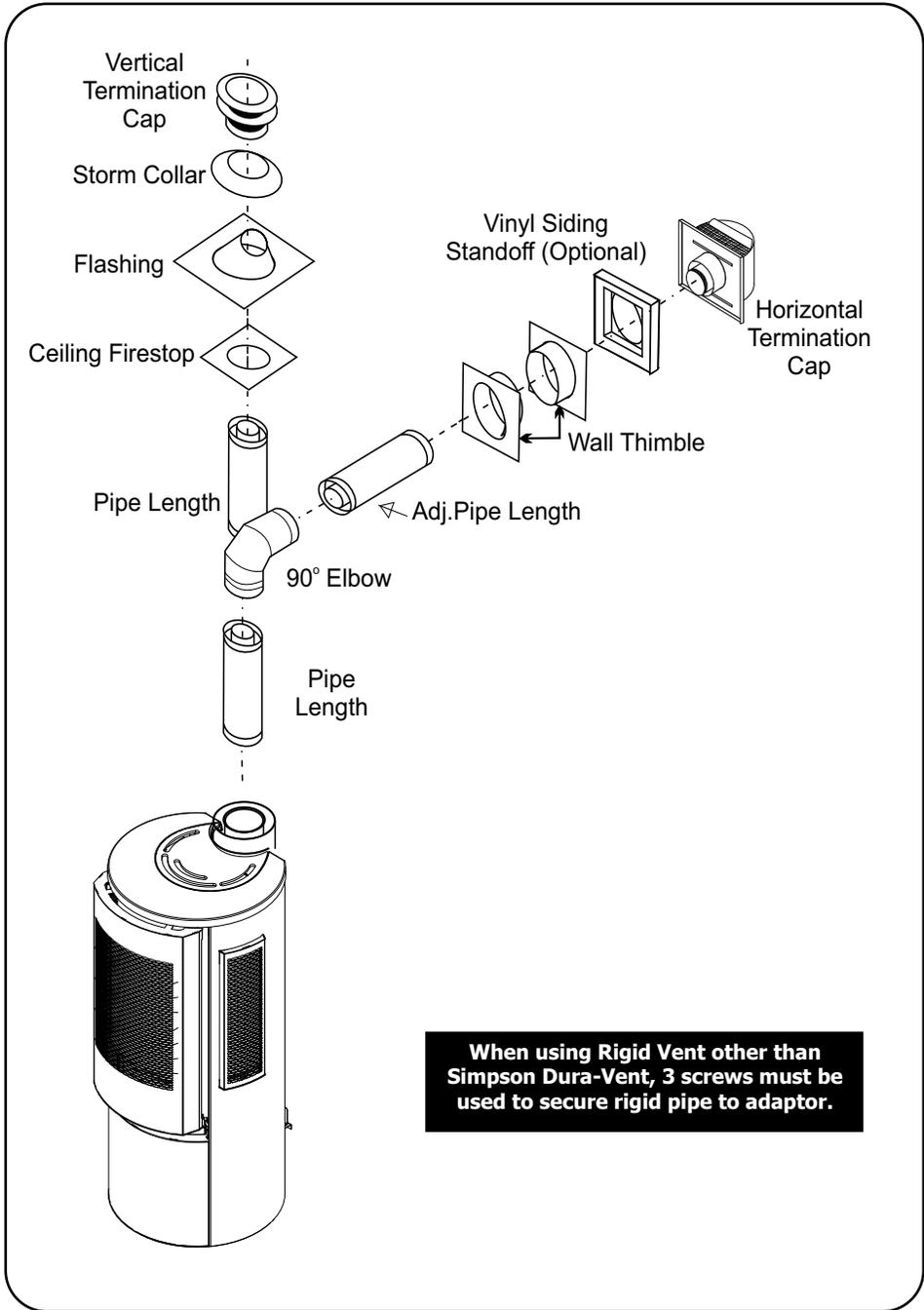
**When using Rigid Vent other than Simpson Dura-Vent, 3 screws must be used to secure rigid pipe to adaptor.**
