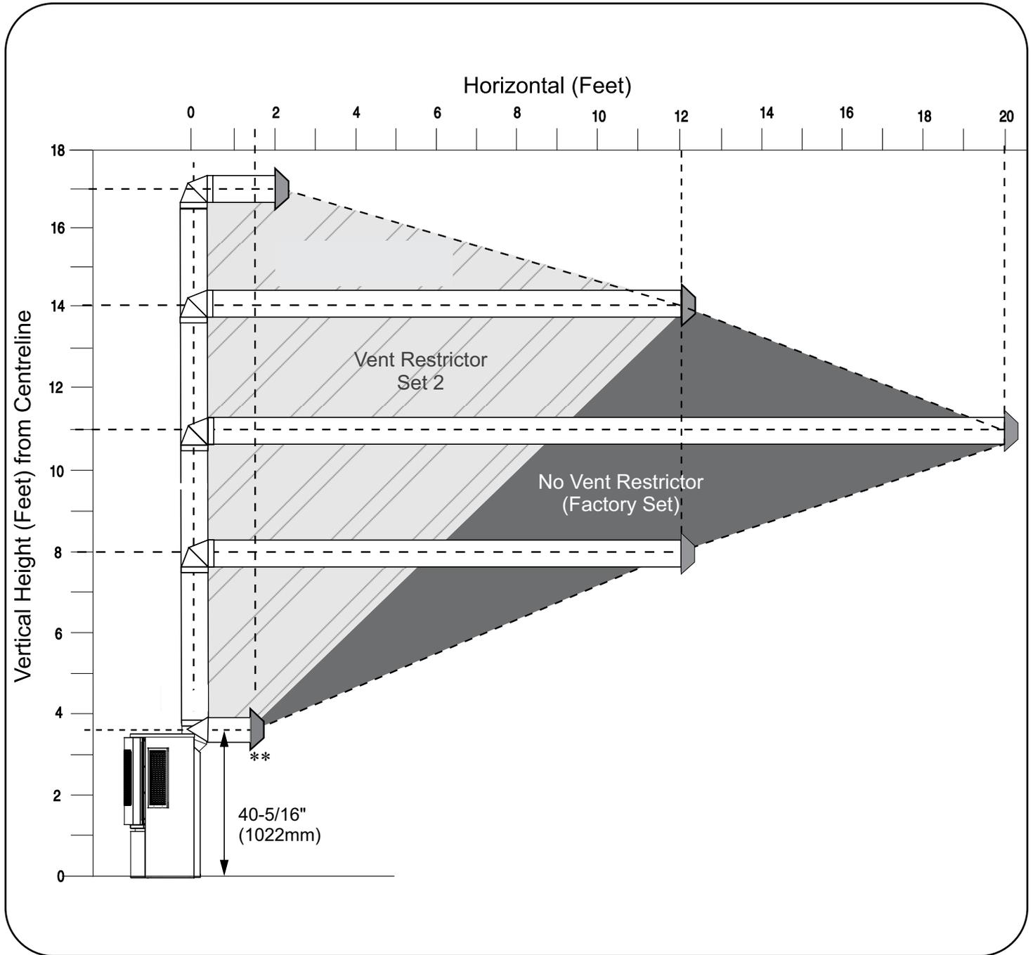
\*\*Note: If termination is rear vented at a minimum to centerline height of 40-5/16" (1022 mm) and horizontal length greater than 12" (305 mm) to a maximum of 18" (457 mm), only a rear vent riser or snorkel may be used. See manual for details.
