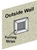
3. Attach the 4" dia. flex liner to the vent terminal ensuring that the flex overlaps the collar of the vent terminal by a minimum of 1-3/8"(35mm). Use Mill-Pac to seal and secure with 3 of the #8 x 1/2" screws (stainless steel).
