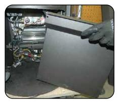
3. Profile of lower access panel showing hook locations. Reverse steps 1 + 2 to reinstall.
