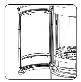
Side glass panels can be replaced in the same manner as the front glass - but there are only 2 brackets securing each piece of side glass as shown below.
