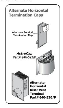
The FPI AstroCap $^{\text{TM}}$  is certified for installations using FPI venting systems as well as Simpson Dura-Vent $\circledR$  and Direct Vent Pro.
