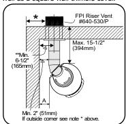
When installed in a corner as shown at 2" minimum clearance from wall to pipe using the 946-544 vent kit.
