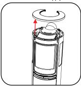
3. Remove 1 screw from the cover of each light assembly housing in locations shown below.
