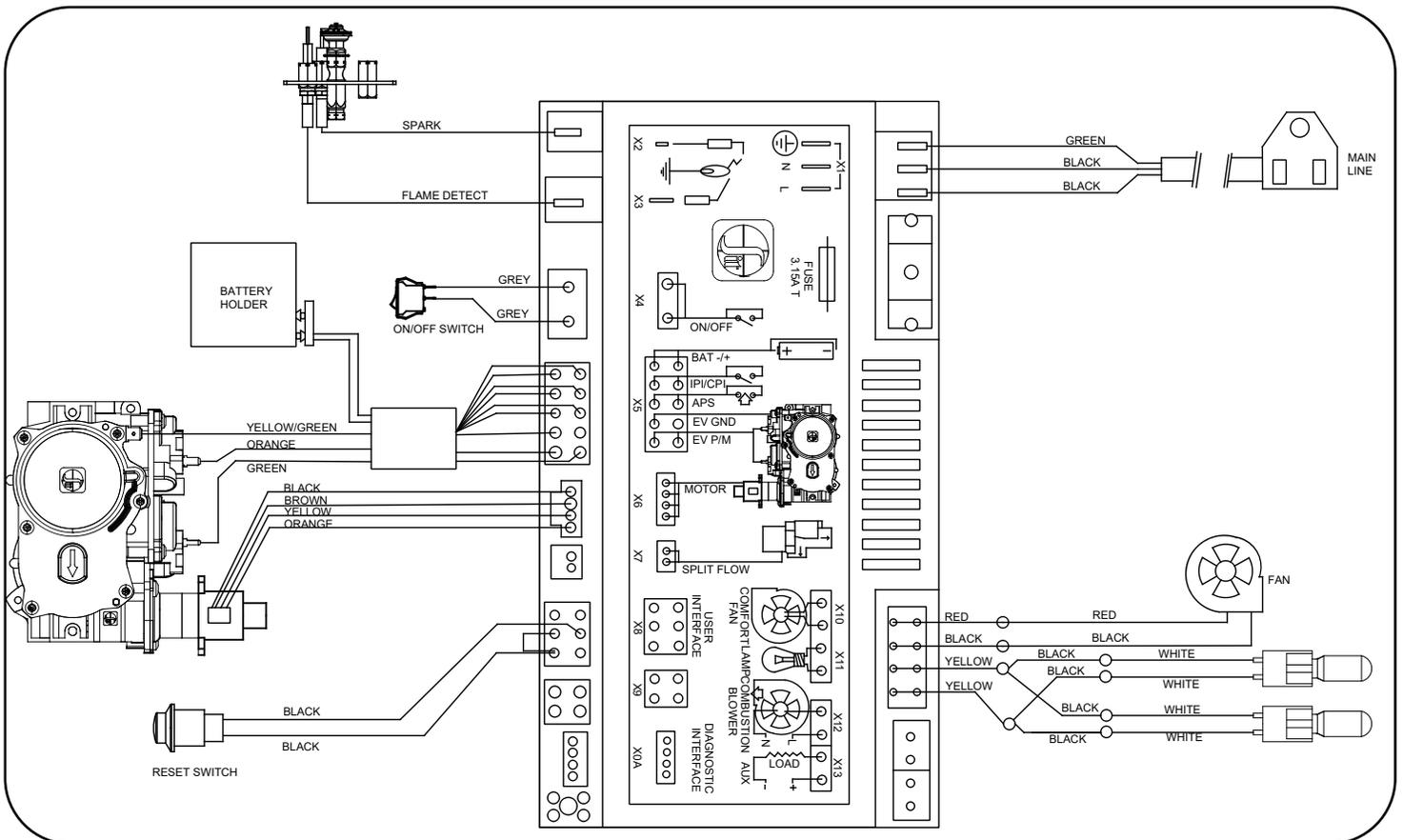
Wiring Diagram With Thermostat
