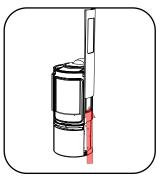
5. Bend out 4 tabs 90° until straight to release glass.
