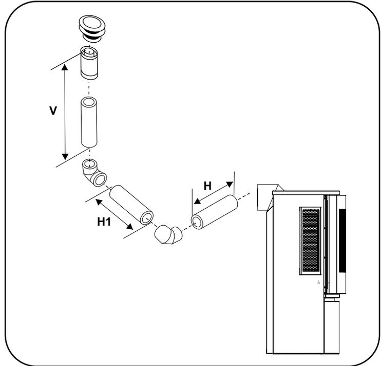
**Co-Linear 3" - 3" Flex Pipe Venting (Masonry Chimney Applications Only)**
