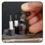
Unscrew the pilot orifice with the supplied Allen key and replace with the LP pilot orifice in the kit --replace pilot cap.
