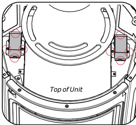
4. Lift housing off unit to replace bulb.
