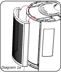
4. Secure the front screen with one bolt installed from the bottom up through the screen bracket and into a nutsert in the screen.
