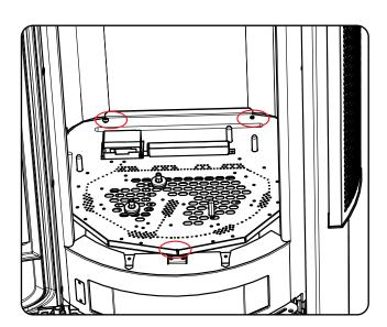
3. Lift burner straight up to remove.
