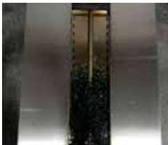
1. Start pouring Crystals/Firebeads on one end of the burner.
