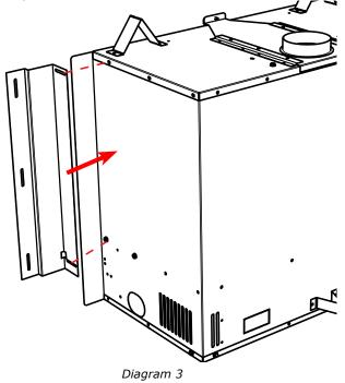
**Note:** Side brackets can be adjusted between 13 mm to 38 mm. This adjustment must be done before unit is moved into framed opening.
