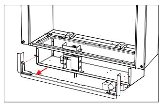
**11**. Remove pilot retainer clip with pliers and pull off the pilot cap to expose the pilot orifice.
