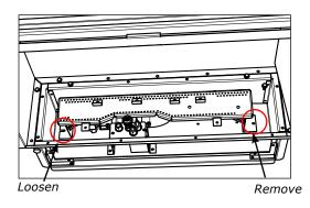
10. Remove 2 screws in location shown below to remove front bracket.
