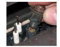
12. Remove burner orifice with a 1/2" wrench and discard. Use another wrench to hold on to the elbow below the orifice.
