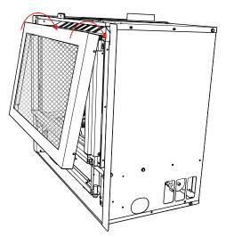
Feed the wire from the digital box on the floor of the unit up through the back of the faceplate and plug into the switch in the location shown.
