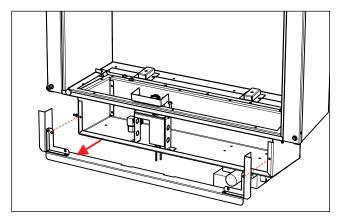
11. Remove 8 screws to remove valve tray - lift up and out to remove.
