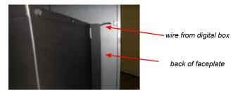
7. Place power cord through opening located on the side of the faceplate and secure with supplied grommet.
