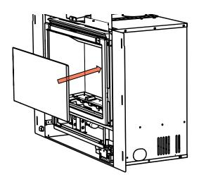
4. Before installing the side panels, loosen the screws for the tabs enough so that you can slide the tabs on to the screws easily but that the tabs are secure. For the location of the side tab screws see Diagram 2.
