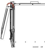
2. Install 2 Faceplate brackets to the top of the unit with 3 screws each.
