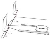
3. Lift Faceplate over brackets on top of unit--hook faceplate over brackets and lower gently.
