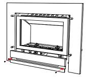
6. Feed the wire from the digital box on the floor of the unit up through the back of the faceplate and plug into the switch in the location shown.
