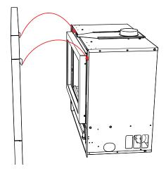
4. When the faceplate is in position, secure with 2 screws in locations shown below and apply the Regency logo to the lower left hand corner.
