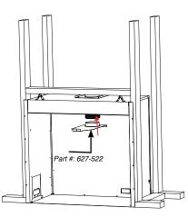
6. Slide the unit into place while guiding the unit flue assembly back into position on top of the unit and secure.
