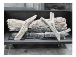
7. Place Log 7 on the left hand side of the burner, Log 7 will sit in a notch on Log 6 and the bottom of Log 7 will rest on a tab located on the burner.
