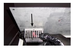
17) The fan control module (supplied with the fan kit) secures to the floor of the unit with a Velcro pad in the position shown in the drawing. Plug the fan control module into the outlet in the unit.
