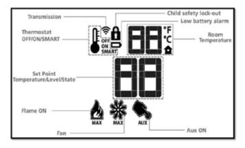
Figure 2: Transmitter LCD Display
