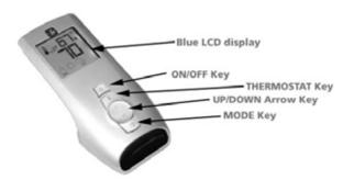
Figure 1: Proflame Transmitter
