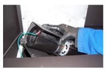
14) Secure the fan to the floor of the unit with 2 screws.
