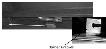
5) With burner removed - lift out burner tray.
