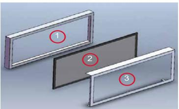
Remove screws from inner side of the inner door frame and discard screws and the brackets. (Brackets not shown). Remove the screen mesh from inner door frame.
