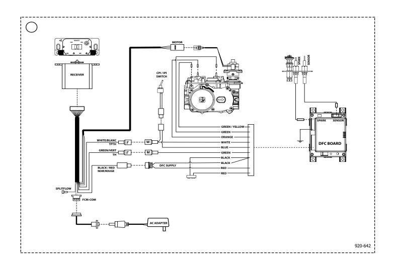
**Note: Either** 4 AA batteries or AC adaptor must be installed to operate the burner switch/Receiver.
