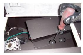
**15)** Attach the ground wire from the fan and the power cord to the ground lug in the unit. The ground lug is located just in front of the receptacle box on the left side on the floor of the unit.
