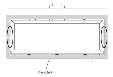
**4)** Remove the door frame overlay by swinging out 45° from the bottom and lift up and out.
