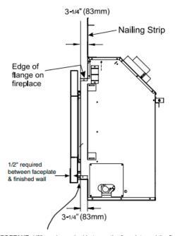
IMPORTANT: 1/2" gap is required between the faceplate and the finished wall when using 4 piece Faceplate (Part # 258-954, 258-957) or Verona Glass Surround (Part # 256-951, 256-957)
