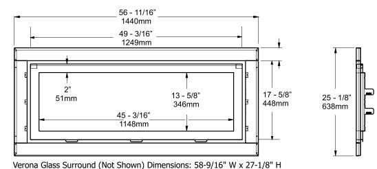
Note: Gas connection is from the right hand side of the appliance & electrical connection on left hand side of the appliance. A metal receptacle box is supplied/installed with the appliance to make all 120 volt electrical connections.
