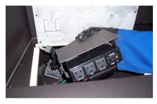
18) Plug in the fan power cord to the Fan Control Module into the outlet marked "Fan". Plug the FCM-COM wire from the remote control wiring harness into the location on the Fan Control Module marked "COM". Turn the switch on the Fan Control Module to the ON position. ON is to the left. The "O" is the off position
