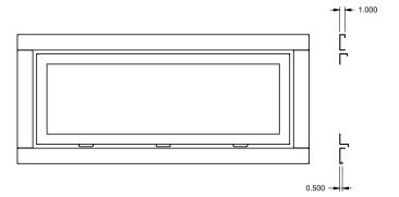
2. Install the faceplate to the unit by hooking the left and right side mounting brackets into the mounting slots at the side of the firebox as shown below. It is recommended that you use the first mounting slot (the one closest to the door frame overlay) out of the 5 so that the faceplate and door frame overlay are flush with one another. See diagram below.
