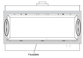
Remove the door frame overlay by swinging out 45° from the bottom and lift up and out.
