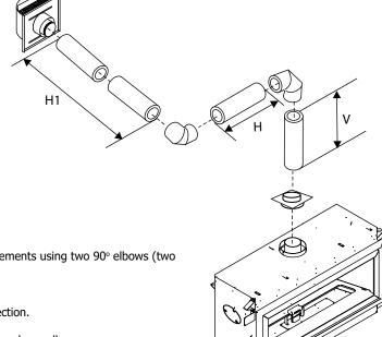
The diagrams below show examples of horizontal termination arrangements using two  $90^{\circ}$  elbows (two  $45^{\circ}$  elbows equal one  $90^{\circ}$  elbow).
