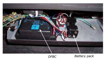
6) Disconnect the CN4 and CN3 wires from the DFBC.
