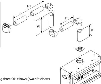
The diagrams below show examples of horizontal termination arrangements using three 90° elbows (two 45° elbows equal one 90° elbow).
