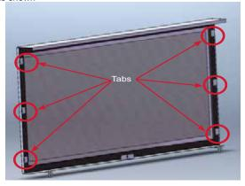
**4.** Hook the outer door frame (3) and mesh screen (2) assembly over the inner door frame.
