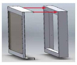
Bend the center tab up and secure with a screw to attach the outer frame/mesh assembly to the inner door frame
