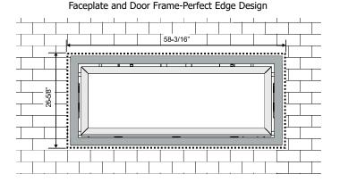
For material such as brick, stone, etc that extends 3-1/8" or less, the minimum opening dimensions noted below must be adhered to when finishing around the unit. This is to ensure the removal of the faceplate and for the safe operation of this appliance.
