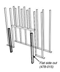
5. Secure horizontal steel header with 2 screws per diagram
