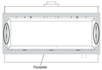
**4)** Remove the door frame overlay by swinging out 45° from the bottom and lift up and out.
