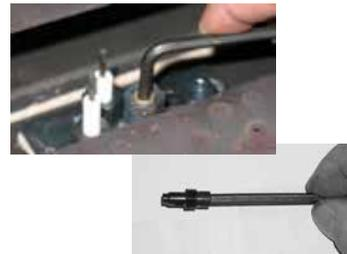
15. Reinstall pilot cap and pilot retainer clip.
