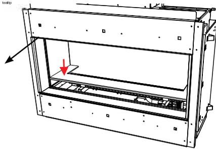
2. Manoeuvre in back panel to the back wall of the unit.
