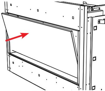
3. Install panel bracket into the slot in the panel.
