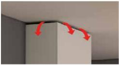
The ventilation opening may be fully open at the top of the enclosure. This type of ventilation opening would be used when the top of the enclosure is not visible from above and where the ceiling within the room is higher than normal. When creating this type of ventilation opening, measures should be into place to avoid having objects of any type falling or be thrown into the ventilation opening. Mesh screen or other preventative measures should be put into place.
