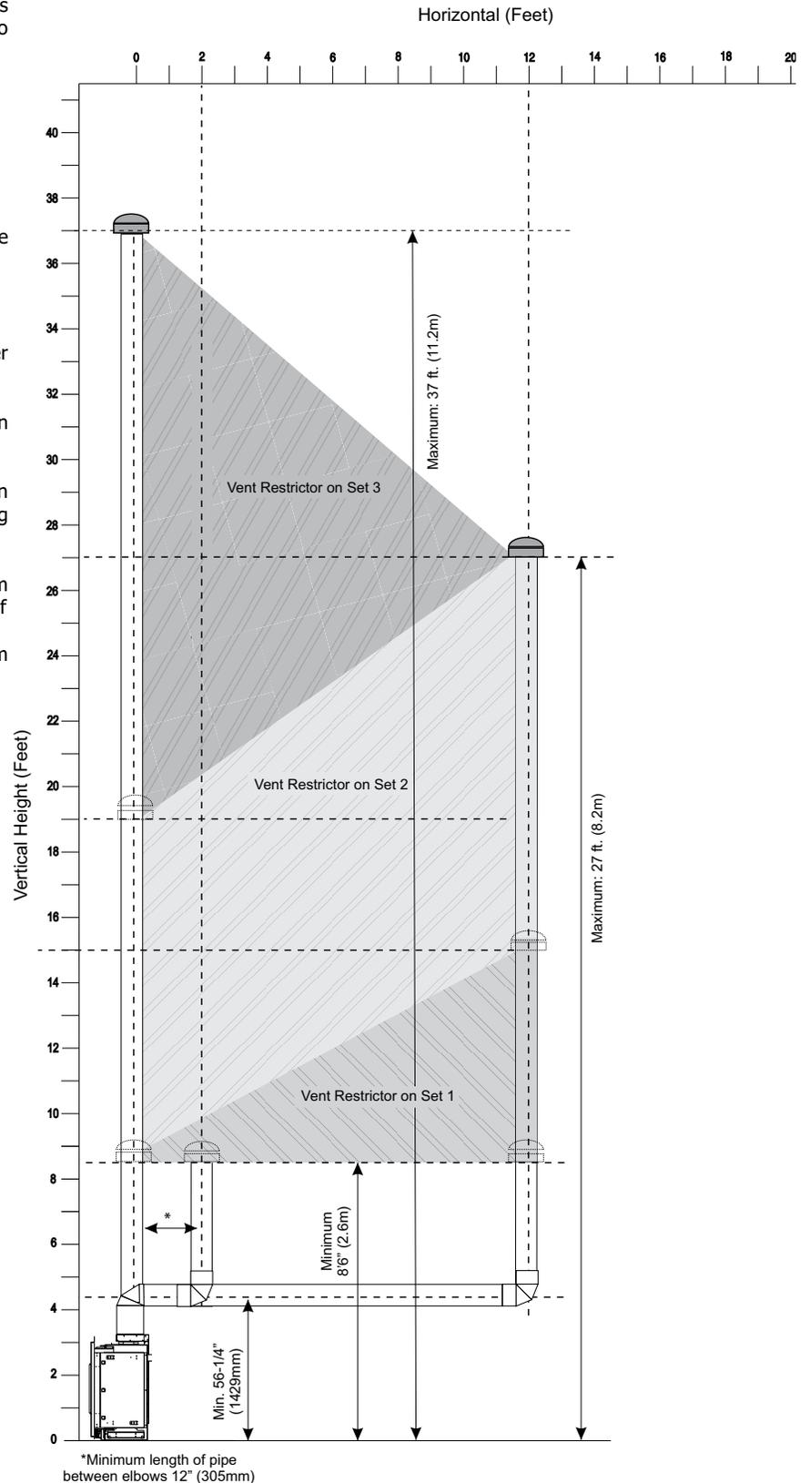
**Vertical terminations - Rigid Pipe 4" x 6-5/8" (Non Power Vent)**
