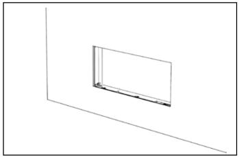
Prior to installing outer liner panels and barrier glass remove finishing trim plates from right and left sides.
