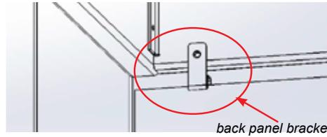
8. Carefully manoeuvre the back glass panel (4) to the back wall of the firebox. Centre the glass panel at the back of the firebox positioning underneath the loosely installed bracket— once in position, slide the bracket in position on the opposite side and tighten both brackets in place with one screw each.
