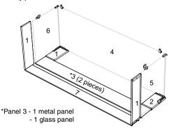
3. Install back corner panels (1, 2) - seat smallest panel in back left corner, repeat on other side.
