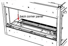
4. Install bottom corner 'securing bracket' as shown. Repeat step for other side.
