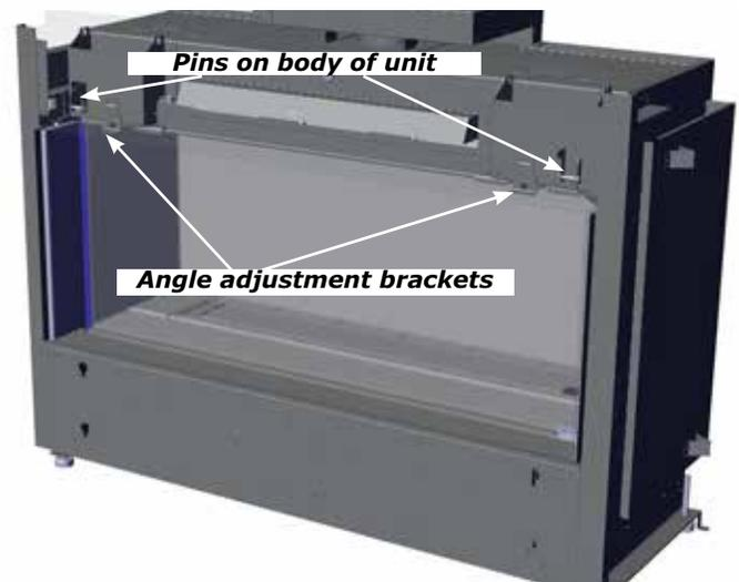
**Note:** If the outer safety glass panel does not sit at 90° and angles too far inward or outward, remove the glass panel and adjust the screw of the panel angle bracket. Turn the panel angle bracket screw in 1/4 increments—reinstall panel to check.
