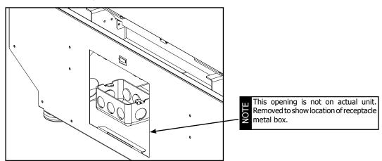
2. Bring the wiring from inside the wall to the receptacle box.
