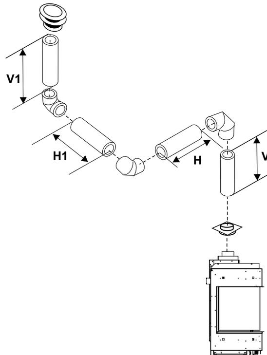
**DuraVent Vertical Termination - 4" X 6-5/8" Venting (Rigid Vent Systems) (Non Power Vent)**
