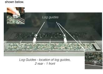
5. Clip on the log guides - position the rear guides by centering over the second and fourth vertical lines at the back of the burner. The front log guide clips on to the front edge of the burner on the right side as
