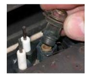
14. Unscrew the pilot orifice with the allen key; then replace with the LPG pilot orifice and the pilot cap, provided in the kit.
