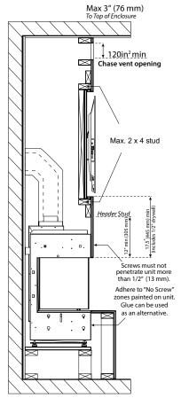
Flush wall TV recess using 1/2" (13 mm) drywall
