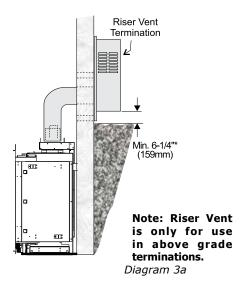
\*Diagrams 3 & 4: As specified in CSA B149.1 Installation Code. Local codes or regulations may require different clearances.
