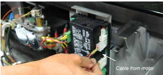
6. If unable to access this Cable - undo 2 screws securing the IFC Board and slide out of unit to access cable.
