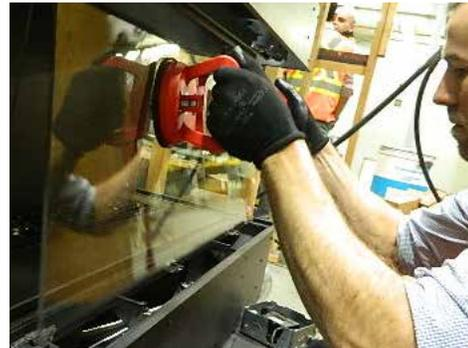
Handle front panel with supplied vacuum clamps
