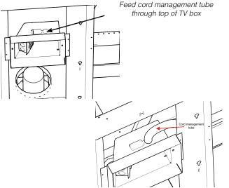
8. Secure the cord management tube to the inside of the framing with the supplied ties.
