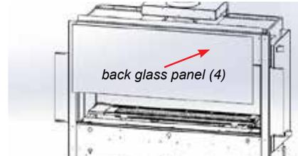
9. With the back panel installed, slide in one of the side glass panels (6). Push the panel all the way to the back of the firebox ensuring that the glass is sitting on the bottom corner bracket installed in step 4. Attach top rear bracket as shown. Note: There is a left and right bracket. The left bracket is shown below.
