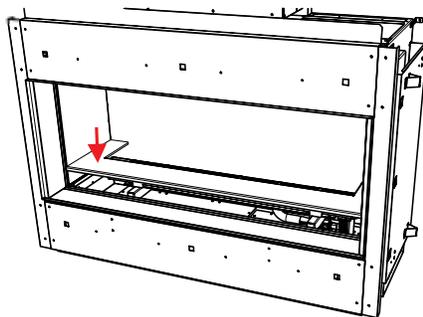
3. Install back enamel panel - manoeuvre panel into unit and position panel at back wall of firebox.
