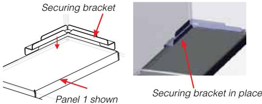
5. Install metal panel (3) into of front firebox panel.
