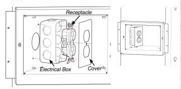
Run the BX cable from the back of the electrical box and route through the framing using the supplied ties (use larger holes in framing to accommodate cable ties).
