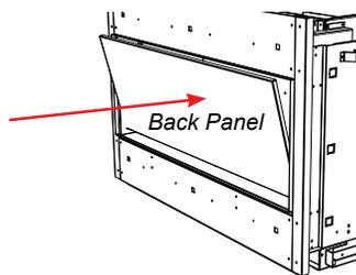
4. With back panel in position — install side panel. Place panel bracket into slot located at top of panel. Place panel and bracket in unit against the side wall. Slide keyhole bracket (installed in panel) over screw in unit to secure side panel.
