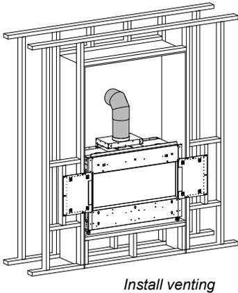
8. Finish the wall with desired finishing material and install rear enclosure venting (see manual for finishing/venting requirements).
