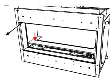
2. Manoeuvre in back panel to the back wall of the unit.
