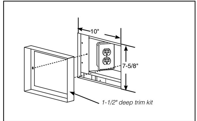
12. Secure TV box to framing with 2 screws per side. See below.
