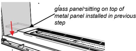
7. Install one of the back panel brackets loosely with one screw (leave the bracket loose to allow room to install the back panel behind it).
