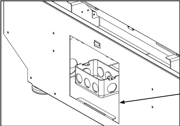
**NOTE** This opening is not on actual unit. Removed to show location of receptacle metal box.
