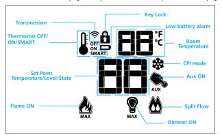
Figure 1: Transmitter LCD Display
