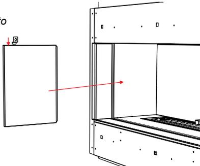
5. When side panel is in position, secure in place with one screw. The side panel, once installed will hold the back panel in position.
