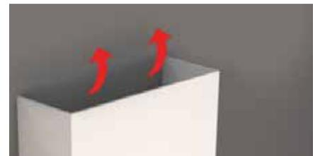
The ventilation opening may be placed on top ensuring it meets the 120 square inch opening. This type of ventilation opening would be used when the top of the enclosure is visible from above and where the ceiling within the room is higher than normal.
