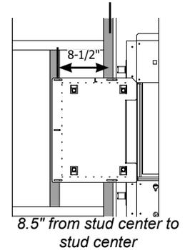
3. Attach left and right base panels using 2 screws on each side. Remove drywall finishing trim from right and left side of window opening using supplied right-angle screwdriver. Screws only need to be loosened to remove both finishing trims. Once removed, re-tighten screws and discard finishing trim.
