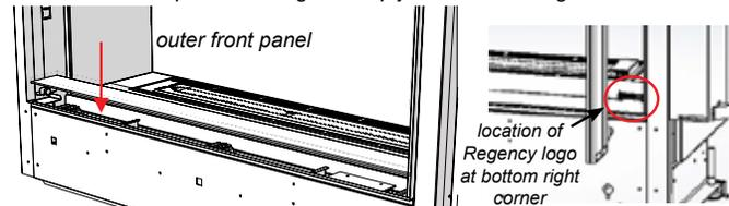
14. Install outer side panels (8, 9) —these panels are held in position with magnets. Clean all fingerprint marks on outer side and bottom panels prior to next step.
