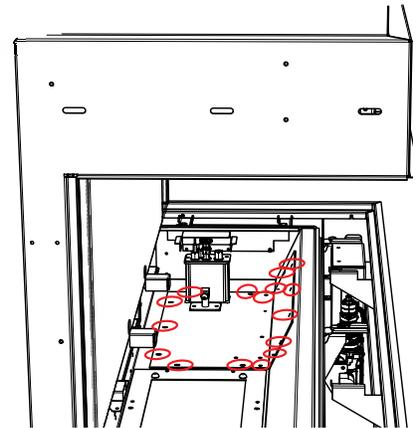
8. Lift valve tray out partially and disconnect flexible gas connection on the valve inlet side, remove valve tray- replace with new valve tray.
