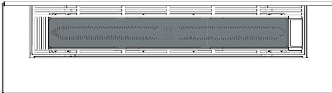
2. Install the 3.5 lb box of black charcoal glass and 1 lb of Andiron embers around the burner. Make sure the burner surround is only 50% covered.
