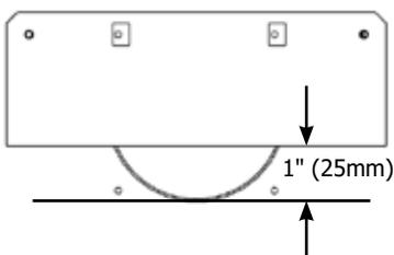
**Venting Arrangement for Vertical Terminations**
