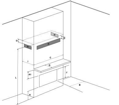
Full framing with low ventilation opening in front or 2 sides
