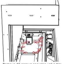
Remove 16 screws securing valve tray
