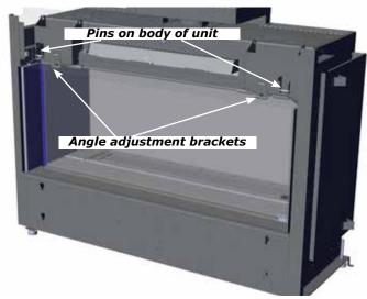
**Note:** If the outer safety glass panel does not sit at 90° and angles too far inward or outward, remove the glass panel and adjust the screw of the panel angle bracket. Turn the panel angle bracket screw in 1/4 increments—reinstall panel to check.
