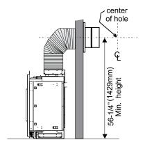
NOTE: A minimum of 1' (305mm) vertical off the top of the unit is required before any horizontal runs can start.
