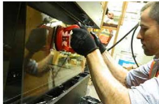
Handle front panel with supplied vacuum clamps
