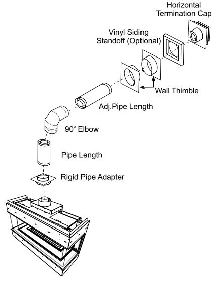
When using Rigid Vent other than Simpson Dura-Vent, 3 screws must be used to secure rigid pipe to adaptor.
