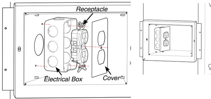
5. Run the BX cable from the back of the electrical box and route through the framing using the supplied ties (use larger holes in framing to accommodate cable ties).
