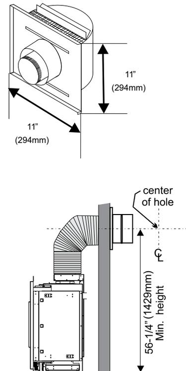
**NOTE:** A minimum of 1' (305mm) vertical off the top of the unit is required before any horizontal runs can start.
