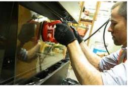
Handle front panel with supplied vacuum clamps
