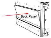
4. With back panel in position — install side panel. Place panel bracket into slot located at top of panel. Place panel and bracket in unit against the side wall. Slide keyhole bracket (installed in panel) over screw in unit to secure side panel.
