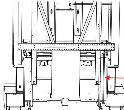
7. Feed the required cords (for TV, PVR, etc.) into the cord management tube, with cords installed, feed the end of the tube + cords through the top of the electrical box.
