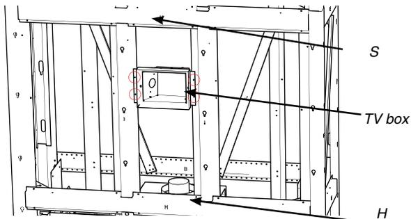
2. Install the electrical box into the TV box with 2 screws—see below.
