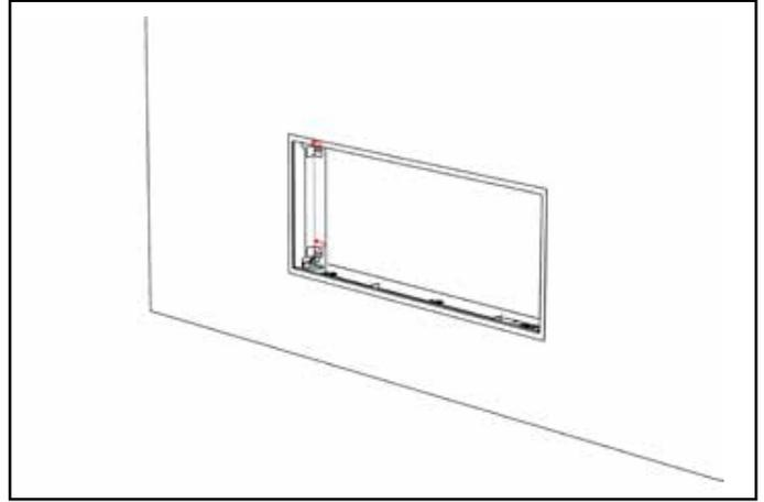
2. Prior to installing outer liner panels and barrier glass remove finishing trim plates from right and left sides.
