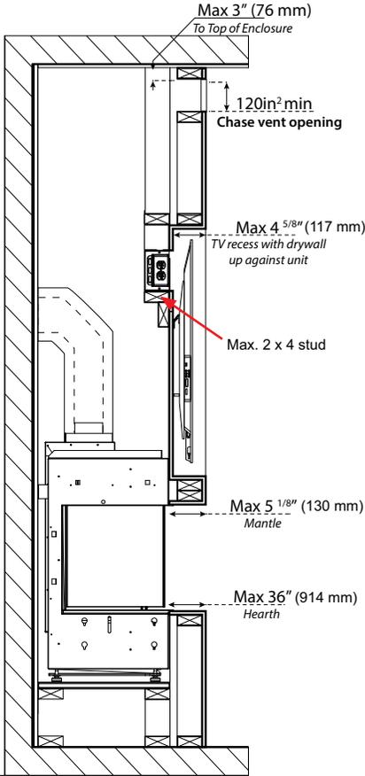
4 5/8" (117 mm) maximum TV recess using 1/2" (13 mm) drywall
