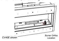
13. Remove pilot retainer clip with pliers and pull off the pilot cap to expose the pilot orifice.
