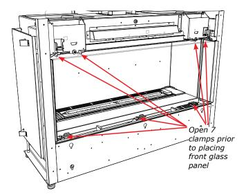
4. Lift up the front panel using the supplied vacuum clamps and position into the lower front channel-ensure the front panel is accurately centered-with the front panel in position—secure in place by closing the 3 lower clamps and 4 upper clamps.
