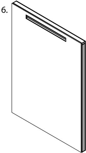
6. Cut hole in finishing material around inside of chase vent. Finish edges around opening
