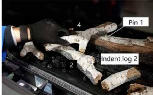
13. Place Log 5—identify the pin locator and match with the right side pin on Log 1. Rest the Log 5 on the indent in Log 3 as shown below.
