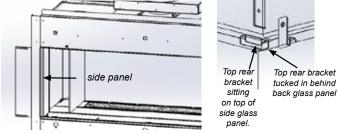
10. Install side panel bracket as shown and secure with one screw.
