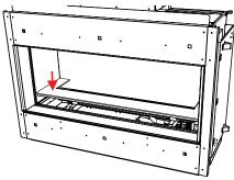
3. Install back enamel panel - manoeuvre panel into unit and position panel at back wall of firebox.
