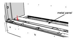
6. Install glass panel (3) on top of the metal panel.
