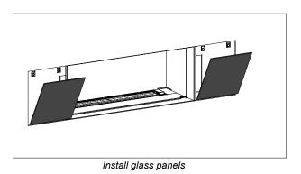
12. Glass panels should overlap with outer side liner panel as shown below.
