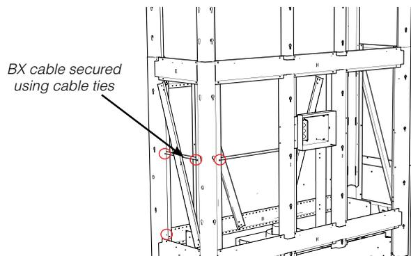
6. Run the BX cable down the back of the unit and to the electrical box located on the front lower left hand side of the appliance and tie in 120 volt power.
