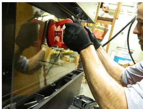
Handle front panel with supplied vacuum clamps
