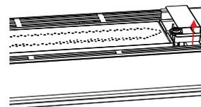
11. Loosen 4 screws in locations shown below (2 at front and 2 at rear)—slide burner to the left away from the orifice and lift out.
