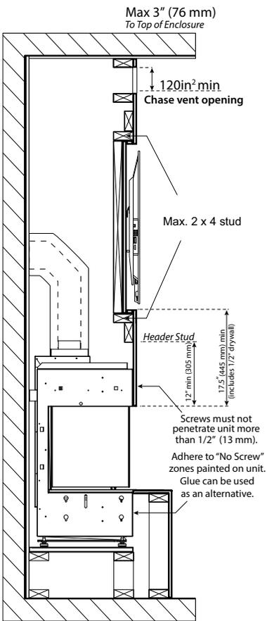
Flush wall TV recess using 1/2" (13 mm) drywall
