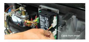
If unable to access this Cable - undo 2 screws securing the IFC Board and slide out of unit to access cable.
