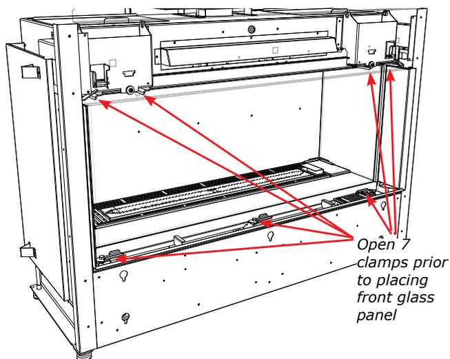
Press glass vacuum clamps in open position firmly onto surface of glass. Bring handles together to close.
