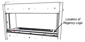
3. Install side panel - the side panel is secured in place by existing magnets in the unit.
