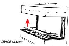
Loosen 4 screws in locations shown below (2 at front and 2 at rear)—slide burner to the left away from the orifice and lift out.
