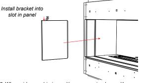
When side panel is in position, secure in place with one screw. The side panel ,once installed will hold the back panel in position.
