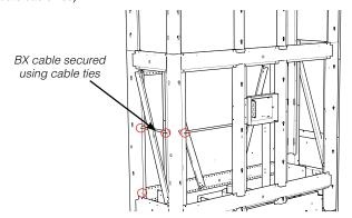
6. Run the BX cable down the back of the unit and to the electrical box located on the front lower left hand side of the appliance and tie in 120 volt power.
