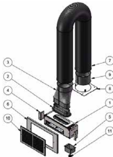
Diagram 1: Guide for possible air duct runs and locations. Keep duct length and number of bends to a minimum. Maximum duct length is 9.0m. The Fan Kit 946-591 does not contain any flueing a separate Flex Kit is required 946-596. This Flex Kit contains one length of 4.5 metres of flex flueing. If 9.0 metres of flex ducting is required you will need to purchase an additional Flex Kit.
