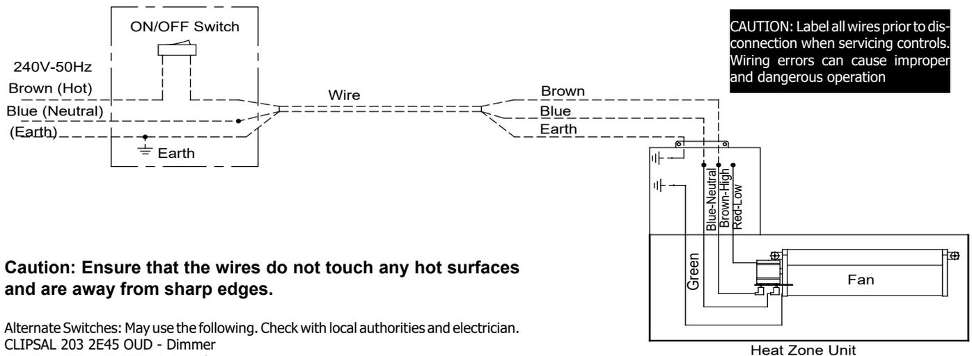
**Caution: Ensure that the wires do not touch any hot surfaces and are away from sharp edges.**
