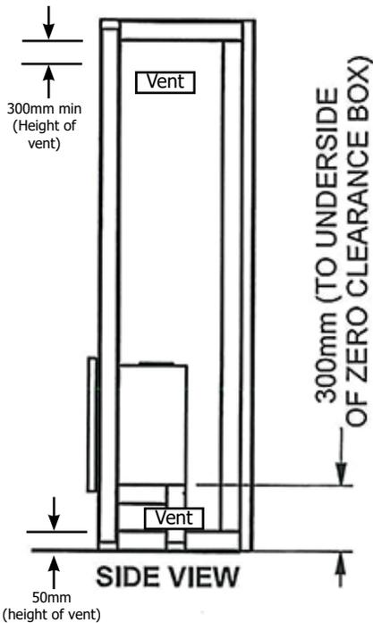
**MUST USE NON-COMBUSTIBLE MATERIALS 315MM ABOVE THE UNITS OUTER SHELL (REDUCED CLEARANCE BOX), 200MM FROM THE SIDES OF THE OUTER SHELL AND ALL BELOW THE HEATER.**
