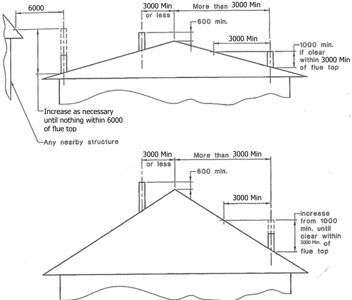
THE FLUE PIPE SHALL EXTEND NOT LESS THAN 4.6 M ABOVE THE TOP OF THE FLOOR PROTECTOR / HEARTH.
