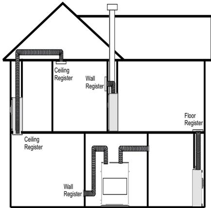
Diagram 1: Guide for possible air duct runs and locations. Keep duct length and number of bends to a minimum. **Maximum duct length is 9.0m.** The Fan Kit 946-591 does not contain any flueing a separate Flex Kit is required 946-596. This Flex Kit contains one length of 4.5 metres of flex flueing. If 9.0 metres of flex ducting is required you will need to purchase an additional Flex Kit.
