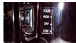
To manually operate the fan system, push the switch on the left to "Man" and switch on the right to either "high" or "Low". This will bypass the sensing device and allow full control of the fan. Switching from "Auto" to "Manual" or "High" to "Low" may be done at any time.
