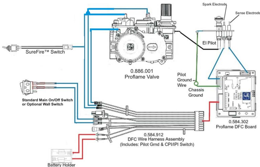
**Note:** 4 AA batteries must be installed to operate the burner switch. Do not use a 9 volt battery.
