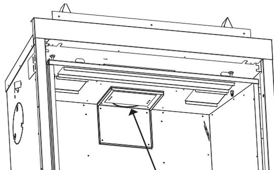
Diagram 2 Vent restrictor installed on top exhaust assembly
