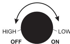
Turn rheostat all the way counter clockwise until you hear a click (**OFF** position). Then turn clockwise slightly, just past click - to **ON** (**HIGH**) position.
