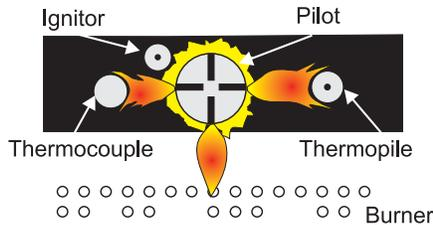
Incorrect flame pattern will have small, probably yellow flames, not coming into proper contact with the rear burner or thermopile or thermocouple.
