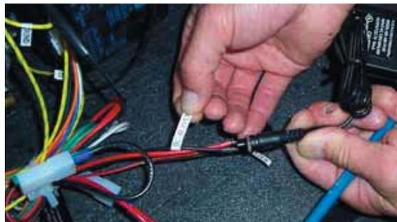
3) Plug AC adaptor into 120V wall outlet (or into 120V receptacle if installed inside the gas fireplace firebox).
