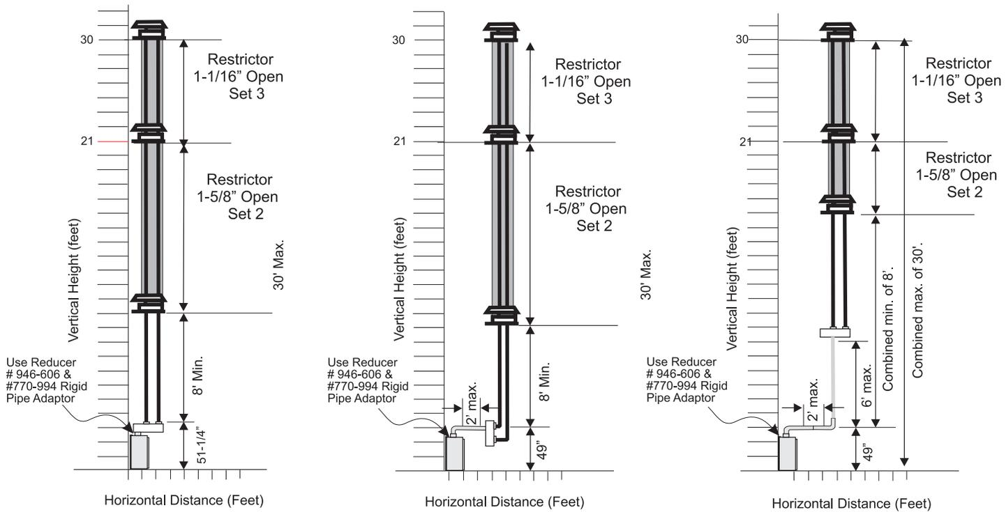
The shaded area in the Diagrams show the allowable vertical terminations.
