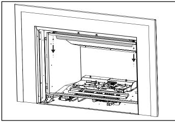
3. Loosen screws and remove brick retainer brackets.
