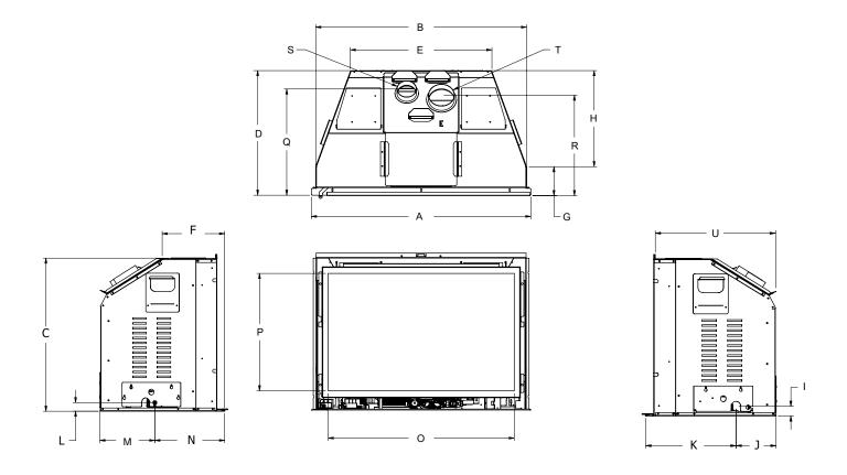
Note: Gas Located on right side of appliance and electrical located on the left hand side of appliance.
