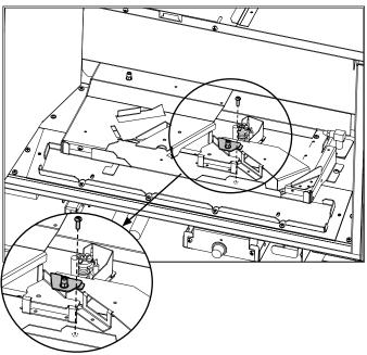
8. Re-install the burner and pilot shield.
