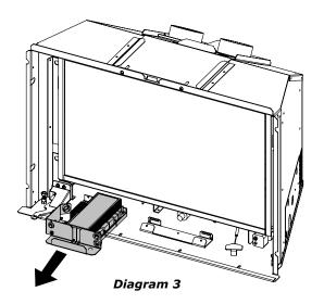
3. Unplug the main power harness (X1) at the PF11 IFC Control Board and disconnect the ground wire from the ground stud. Unplug fan & lights (X10) at the PF11 IFC Control Board to allow for better access to the IFC.
