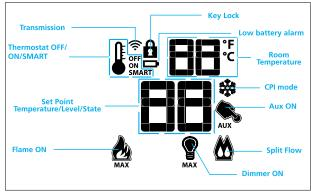
Figure 2: Transmitter LCD Display
