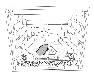
10. Place Log 5 on the pin under the right burner.
