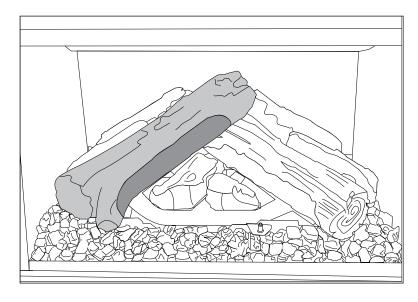
19. Place Log 8 on the pin on the front log mount. The other end will rest on the ember media.
