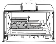
Pull off the pilot cap to expose the pilot orifice.
