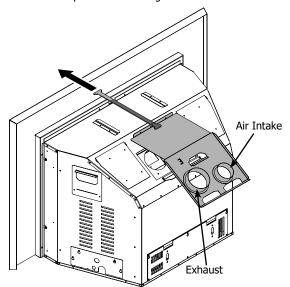
Ensure the draft hood is properly secured and screws tight to create proper seal.
