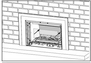
The brick panel sets must be installed with the arrow on the back of the panel pointing up to align the grout lines.
