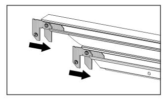
2. Tighten the top screws (x4).
