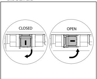
3. Alternatively, rotate the knob to turn it into a handle for more leverage. Clockwise closes the valve, counter-clockwise opens it.
