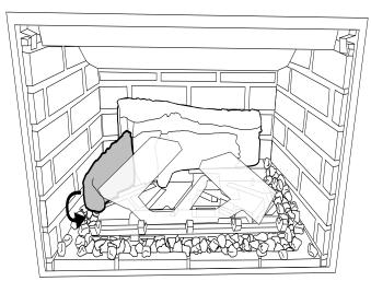
8. Place Log 3 on the pin and rotate it until it touches the tab shown below. Ensure that Log 3 is resting directly on the tray with no embers underneath.
