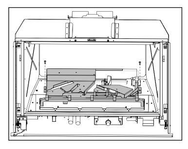
4. Remove the light tray by removing the 12 screws and disconnecting the light tray cable underneath.
