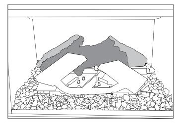
13. Place Log 2 behind the left portion of the burner, resting its right side in the notched area on Log 1. Rotate the front of Log 2 onto the metal flange and ensure it is resting directly on the tray, with no embers underneath.
