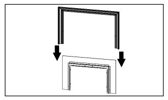
Insert and tighten the rear screws (x5). Traditional surround installed.
