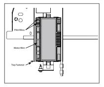
Disconnect the cable coming from the pressure regulator motor at the IFC board (marked X6 on the IFC).
