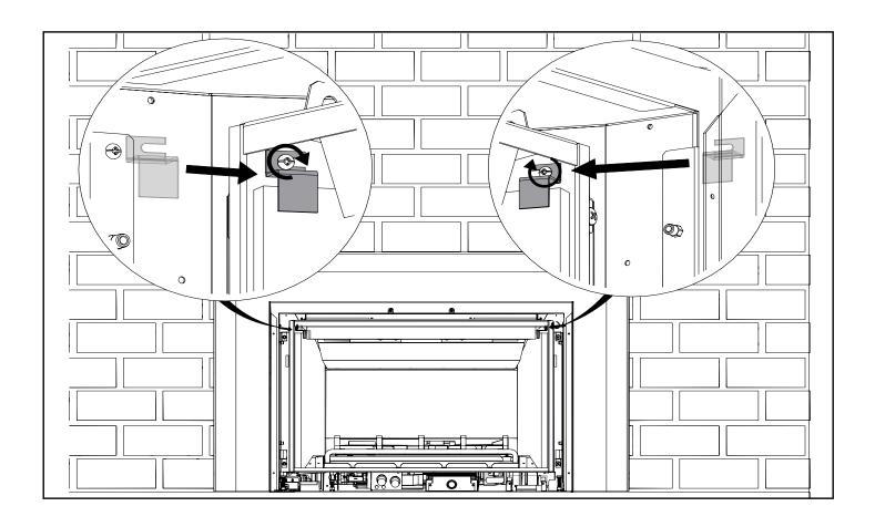
8. Install the front panel(s)\* by placing between the front of the firebox and the media tray.
