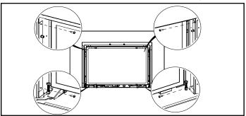
3. Fasten four screws on both sides to attach the backing plate.
