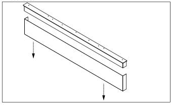
2a. If using a grinder (recommended): Trim the lower section to height refering to the installation table for the amount to remove.
