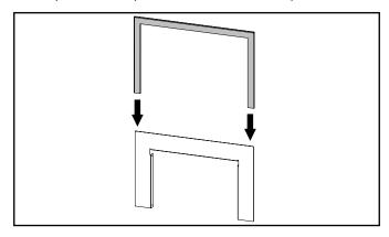
2. If using a Gi33 3-Sided Flush Faceplate (391-912), place the magnet on face A. One magnet per bracket.
