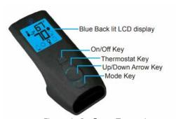
Figure 1: Proflame Transmitter
