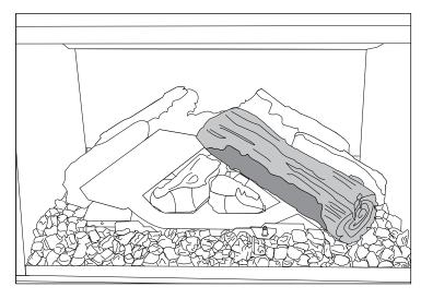
18. Place Log 7 on the left of the burner. The log rests on the burner.
