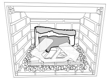
7. Place Log 2 behind the left portion of the burner, resting its right side in the notched area on Log 1. Rotate the front of Log 2 onto the metal flange and ensure it is resting directly on the tray, with no embers underneath.
