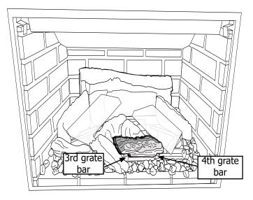
14. Place Log 9 on the right end of the burner. The log rests on the burner, not on the fifth grate bar.
