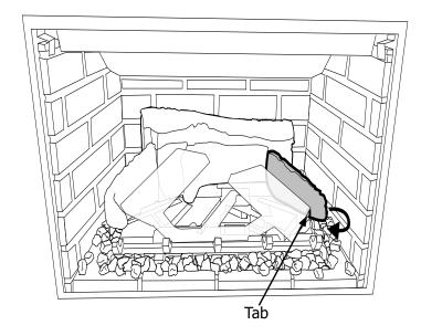
9. Place Log 4 on the two pins under the left burner.
