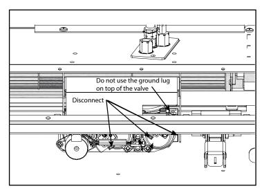
Remove tray fastener by removing 1 phillips head screw as shown below, slide out IFC tray and disconnect the pilot wires marked X2 & X3 on IFC and motor wire marked X6 on IFC.
