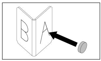
3. Ensure the faceplate and faceplate surround are pressed against each other. Insert the brackets on both sides, at the bottom.
