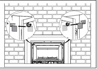
4. Insert the rear panel and hold in place while installing the left and right panels.
