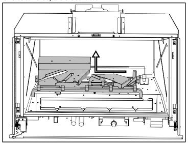
2. Remove the burner tray (2 screws).
