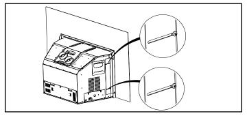
8. Pull the backing plate as far forward as possible against the faceplate, then retighten the screws on both sides.
