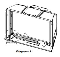
1b. Remove the left side cover (loosen the top two screws and lift up and out).
