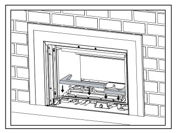
9. Reinstall the blocker and secure using the previously removed screws.
