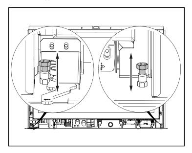
5. From below: The bolts can be flipped around and installed from the bottom of the insert for extended length. Once it is in position, adjust the bolts to ensure the appliance is level and won't rock.
