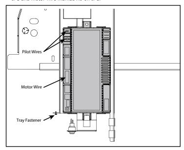
Warning: Ensure wires are tucked back into place and not touching the firebox base after servicing.
