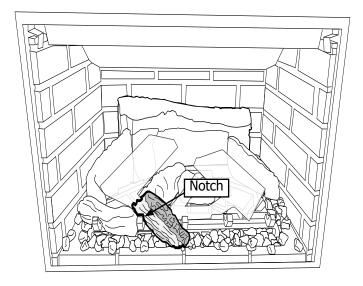
13. Place Log 8 between the third and fourth grate bar. The charred section at the top of the log faces the inside of the firebox.
