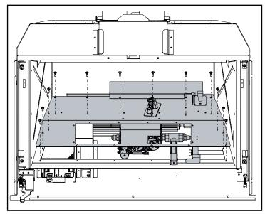
9. Remove the 2 screws from each side of the valve and disconnect pilot gas line to remove valve.
