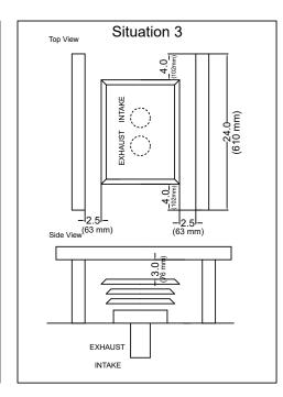
Note: Restrictor must be set to 3-1/2" (89 mm) open for NG or 4-1/4" (108 mm) open fo LP.
