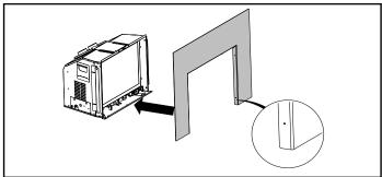
6. Fasten the four screws on both sides to attach the faceplate.
