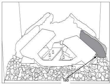
15. Place Log 4 on the two pins under the left burner.
