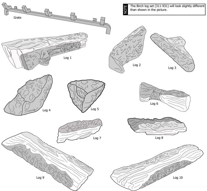
2. Install the log grate with the two screws provided.
