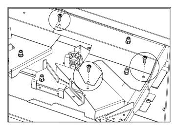
3. Remove 3 screws attaching the pilot shield to the burner tray.
