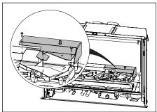
6. Remove the burner tray (2 screws).
