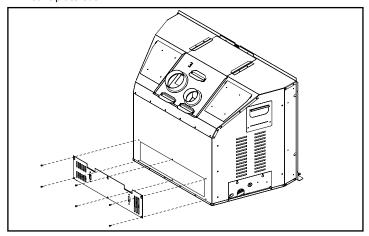
Remove the electrical access panel from the left side of the insert by removing five screws.
