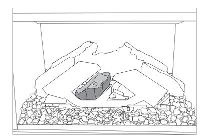
16. Place Log 5 on the pin under the right burner.
