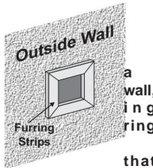
**Note:** If installing termination on siding covered a vinyl siding or furring strips must be used to ensure the termination is recessed into the siding. For vinyl siding standoff installation refer to the Dura-Vent Termination instructions.
