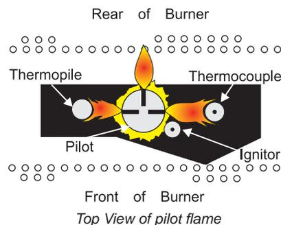
Incorrect flame pattern will have small, probably yellow flames, not coming into proper contact with the rear of the burner or thermopile.
