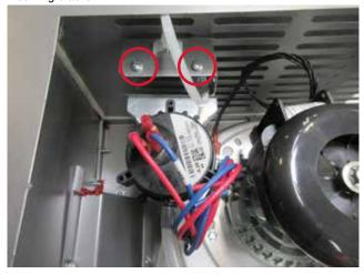
2. Turn the mounting bracket 90 degrees, line up the holes and screw the bracket back onto the mount.
