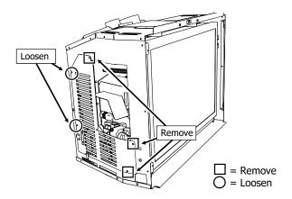
2. Remove 5 screws and loosen 2 screws along the bottom to remove fan access panel.
