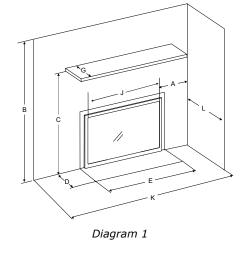
NOTE: 36" (914 mm) wide x 12" (305mm) deep non combustible hearth is required in front of the appliance, unless the unit is raised 3-1/2" (89 mm) off the floor surface.
