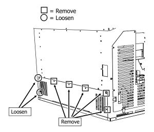
3. Remove ground wire of main harness (X1) from the ground stud.
