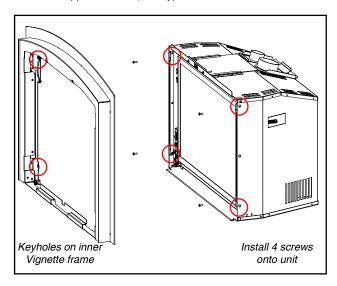
Install the inner Vignette frame by hanging the frame off the 4 screws via the keyhole openings on the frame. When in position, tighten the 4 screws.
