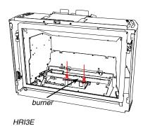
8. From inside the firebox, remove pilot retainer clip with pliers and pull off the pilot cap to expose the pilot orifice.
