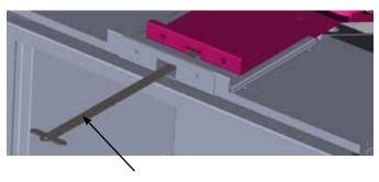
Flue Connector Slide Tool
