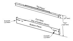
Reattach the top piece of the hearth trim to the cut bottom piece by fitting in place and secure with supplied clips, one on each side.
