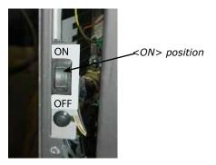
Press and release the black SYNC button (below the ON/OFF switch). The Receiver will "beep" three (3) times to indicate that it is ready to synchronize with a Transmitter.
