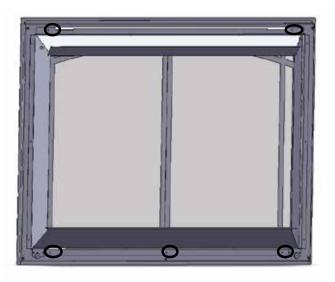
7. Install the Vignette frame with Inlay onto the 2 hooks provided on the unit.
