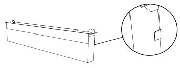
3. Ensuring back faceplate is in place - line up the hearth trim with base of the unit and secure it with 2 screws as shown below.
