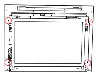
Install mantel deflector onto the back side of the back faceplate with 2 screws as shown below.
