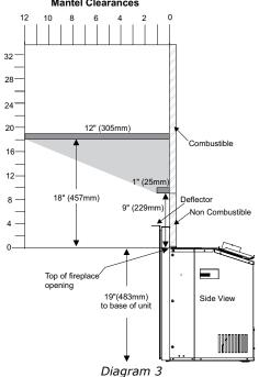
Note: A 3-1/2" mantel deflector to reduce mantel height to 28" from bottom of unit @ 1"depth.
