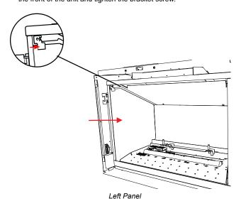
4. Loosen bracket screw in firebox in location shown below, slide right panel into position until it contacts the back panel. Slide the panel bracket on from the back of the unit and tighten the bracket screw.
