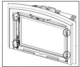
4. Install the safety screen into the inner Vignette frame by slightly tilting the safety screen frame and placing it up into the Vignette frame. Let the safety screen slightly drop down into position within the Vignette frame. The bottom of the screen will be held in position by magnets.
