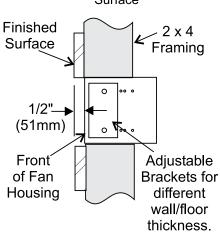
Diagram 2: Side View - Secure fan housing to minimum 2 x 4 framing.
