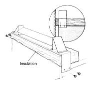
IMPORTANT: Insulation extends forward to seal against the back of the fireplace masonry or non-combustible face.
