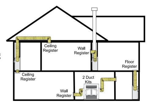
Diagram 1: Guide for possible air duct runs and locations. Keep duct length and number of bends to a minimum. Maximum duct length is 20 ft. (6.1m) per kit.
