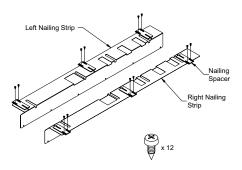
2) Mount Nailing Strips left, right and top to the positions indicated below.
