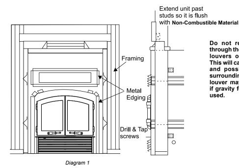
Do not restrict air flow through the top and bottom louvers of the fireplace. This will cause overheating and possible ignition of surrounding materials. Top louver maybe closed only if gravity feed kit option is used.
