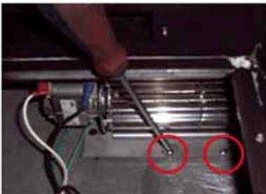
3. Attach the green ground wire to the ground lug – located in the lower left back corner of the unit.
