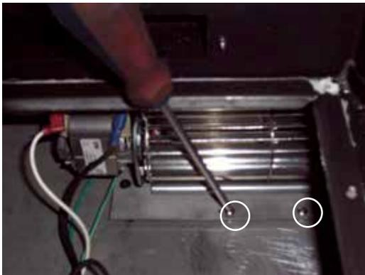
11. Connect the Black wire to the fan motor spade and the other end of the black wire spade to the thermdisc.
