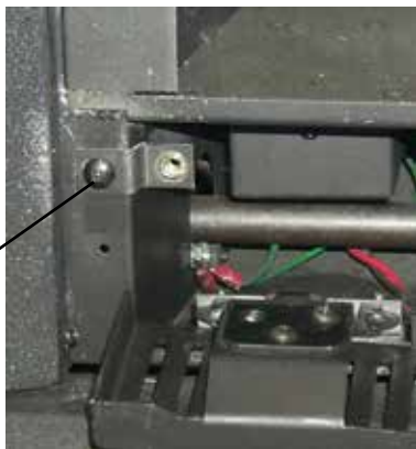
Secure bracket with screw.
