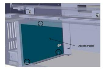
17. Install the fan control module (FCM) into the bracket on the side access panel. Plug in the power cord to the outlet in the unit.
