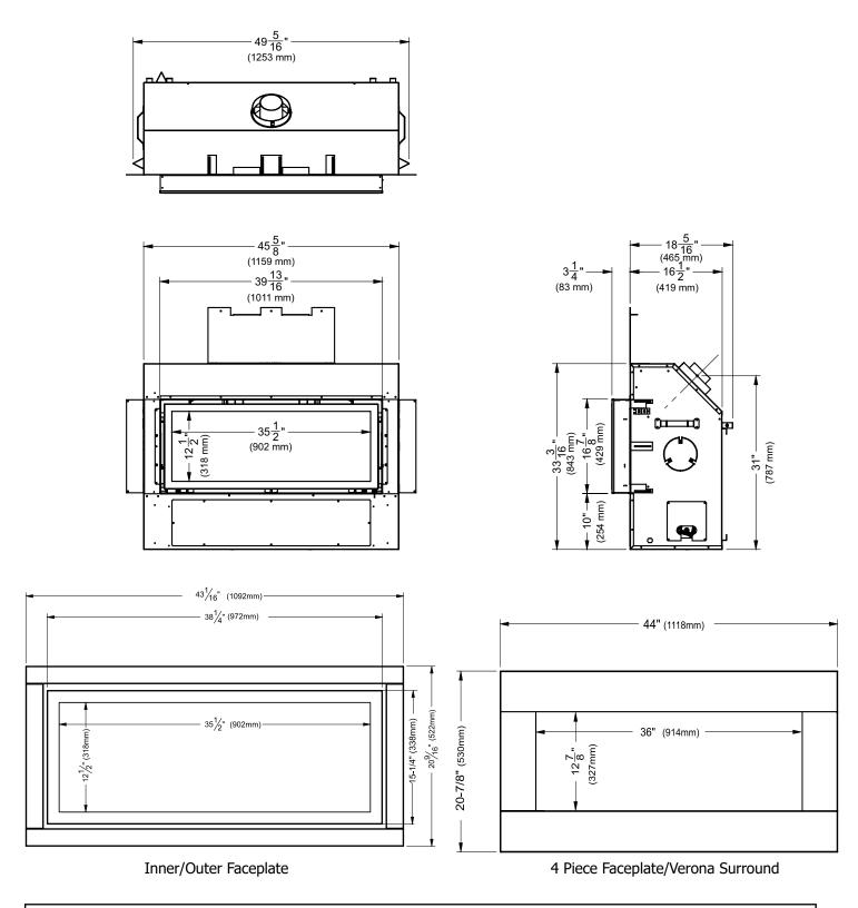
Note: Gas connection is from the right hand side of the appliance & electrical connection on left hand side of the appliance. A metal receptacle box is supplied/installed with the appliance to make all 120 volt electrical connections.
