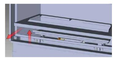
7. Remove 3 screws on the burner to release it - locations shown below.
