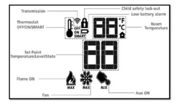
Figure 2: Transmitter LCD Display
