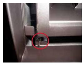
The Surefire switch is discreetly hidden in the bottom right corner of the unit.
