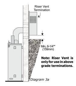
\*Diagrams 3 & 4: As specified in CSA B149.1 Installation Code. Local codes or regulations may require different clearances.
