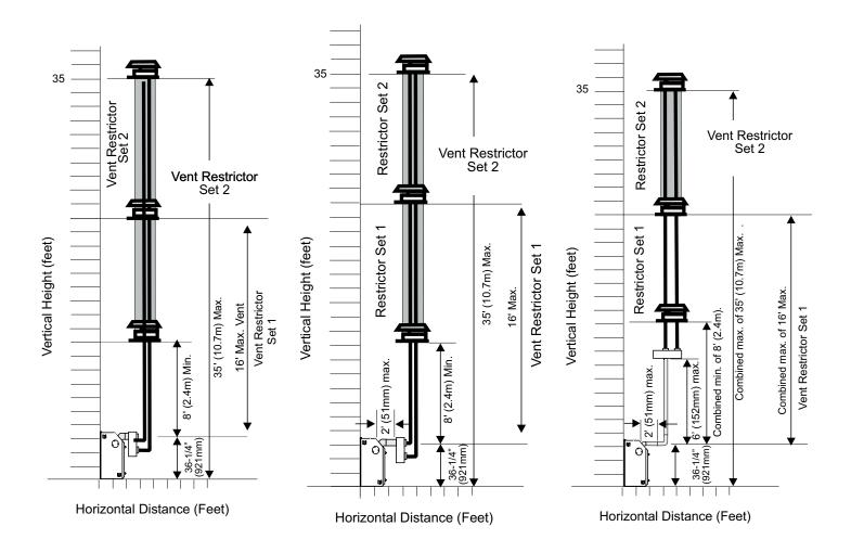
The shaded area in the diagrams show the allowable vertical terminations when using two- 3" co-linear aluminium flex and  $4 \times 6-5/8$ " rigid pipe.
