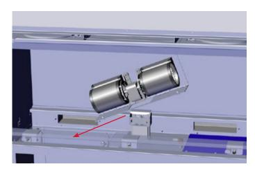
**10.** Secure the fan to the base with 2 screws. Note the right access panel was removed to allow easier access to the right side screw.
