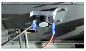
Secure the ground wire from the fan assembly and the power cord to the ground lug located on the back left near the fan.
