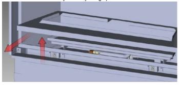
5. Loosen 3 screws at the back of the burner to release it.
