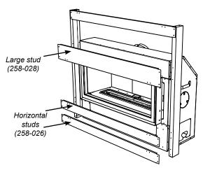
9. Secure 2 vertical studs on either side of the appliance with 4 screws per side stud as shown.
