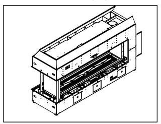
3. Locate the bracket holding the bottom end clamps and loosen the two screws to remove the bracket.
