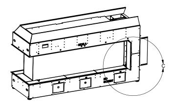
12. Install additional glass stoppers at the end of the unit by sliding the stopper assembly between the unit and panel - the stopper assembly will attach to the unit via a magnet, adjust position of glass stopper if required.
