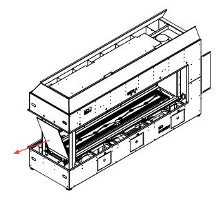
8. Reverse process to reinstall End firebox glass panel.
