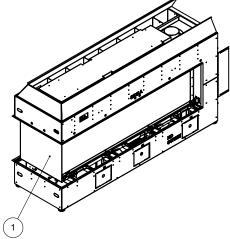
6. Holding the glass barrier in front of the unit, slide it up behind the top lip of the unit. Lift the barrier up as far as it goes, then hook the barrier onto the unit.
