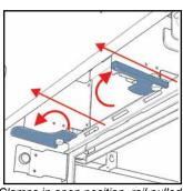
Clamps in open position, rail pulled forward
