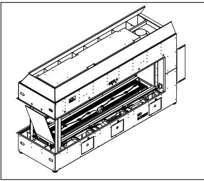
NOTE: UNDER NO CIRCUMSTANCE MAY THE END FIREBOX GLASS BE REMOVED FROM THE FIREPLACE. ONLY REMOVE THIS GLASS PANEL WHEN TRANSPORTATION SUPPORT BRACKETS ARE IN PLACE.
