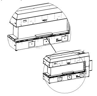
There are 4 optional stoppers included in the manual pack which provide additional support to the glass barrier, if desired - install the stoppers prior to installation of the barrier glass.
