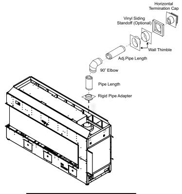
When using rigid vent other than Simpson Dura-Vent, 3 screws must be used to secure rigid pipe to adaptor.
