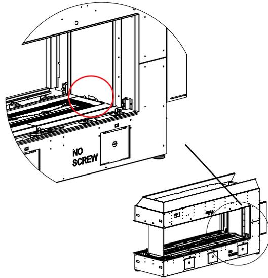
6. Slide the side glass panel #4 into the bottom side bracket.
