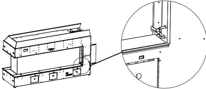
8. Slide the side #5 outer panels between the wall and the barrier stopper bracket. Repeat steps to install the remaining #5 outer panels using a barrier stop where required.
