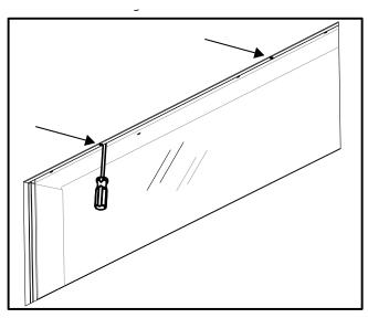
Slide the screwdriver straight up at the two indicator slots.
