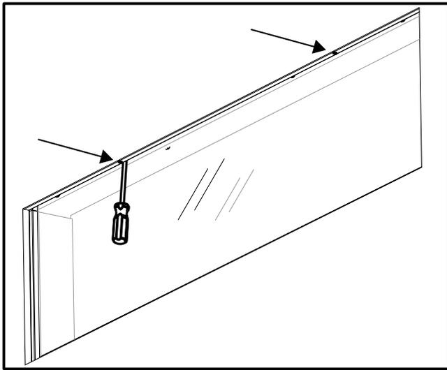
Slide the screwdriver straight up at the two indicator slots.
