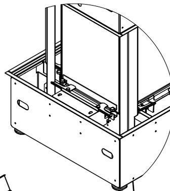
NOTE: UNDER NO CIRCUMSTANCE MAY THE END FIREBOX GLASS BE REMOVED FROM THE FIREPLACE. ONLY REMOVE THIS GLASS PANEL WHEN TRANSPORTATION SUPPORT BRACKETS ARE IN PLACE.
