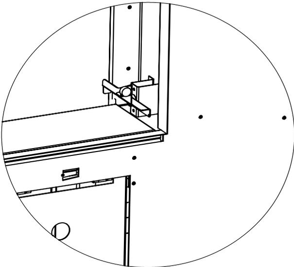
12. Install additional glass stoppers at the end of the unit by sliding the stopper assembly between the unit and panel – the stopper assembly will attach to the unit via a magnet, adjust position of glass stopper if required.
