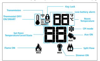
Figure 1: Transmitter LCD Display
