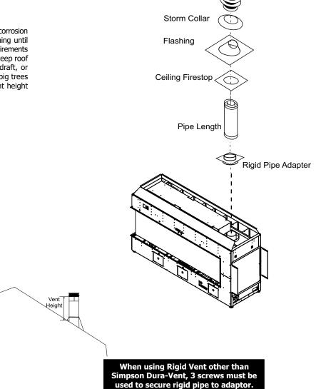
This product was evaluated by Intertek for using a Rigid Pipe Adaptor in conjunction with Duravent Direct-Vent, Selkirk Direct-Temp, Ameri Vent Direct Venting, ICC Excel Direct, Olympia Ventis DV, and Security Secure Vent systems. Use of these systems with the Rigid Pipe adaptor is deemed acceptable and does not affect the Intertek WHI listing of components.
