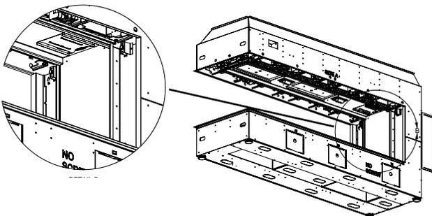
3. Drop the six #3 inner panels into the firebox, then drop the two #2 side covers, as shown below.
