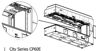
3. Drop the six #3 inner panels into the firebox, then drop the two #2 side covers, as shown below.
