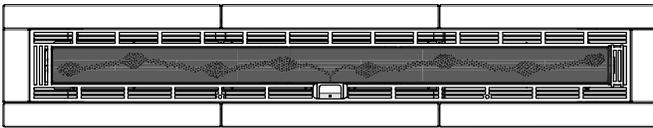
2. Install the 3.5 lb box of black charcoal glass and 1 lb of Andiron embers around the burner. Make sure the burner surround is only 50% covered.
