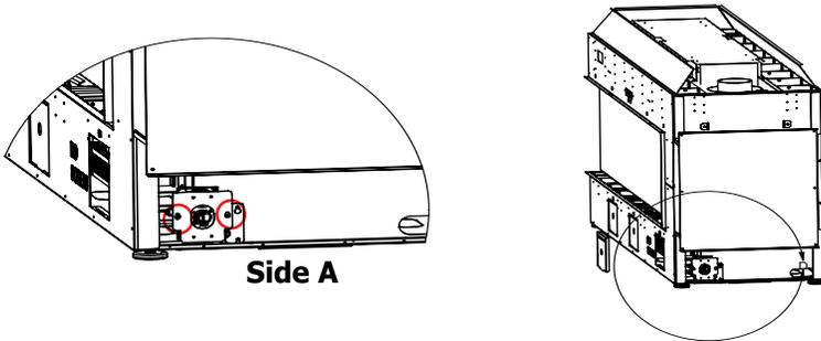
3. Slide electrical box plate towards the back of the unit and then out.
