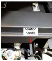
The aeration handle is located near the right side of the gas valve access door, attached by a magnet.
