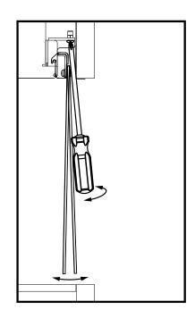
8. Install Side A and Side B barrier glass.
