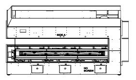
4. Slide in the #6 side panels and secure them by thightening the two screws installed in step 1.
