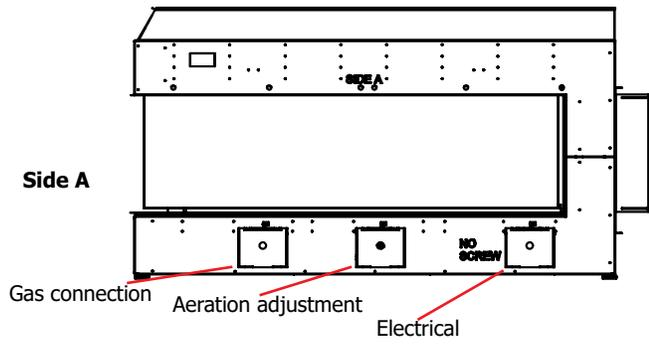
1. Identify the access panel and remove the corresponding outer trim panel by lifting it up and off (centre panel shown opposite).
