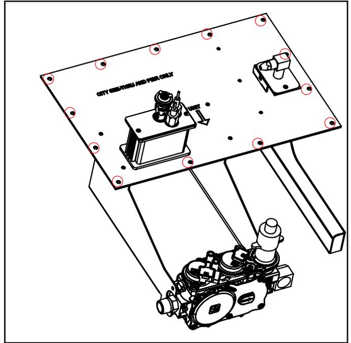
10. Lift valve tray out partially and disconnect flexible gas connection on the valve inlet side. Remove the valve tray and replace it with the new valve tray & valve assembly gasket.
