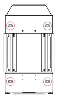
Access holes for removing transportation
