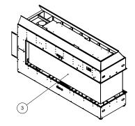
9. Adjust the Side A and Side B barrier glass angle to be parallel with the End barrier glass.
