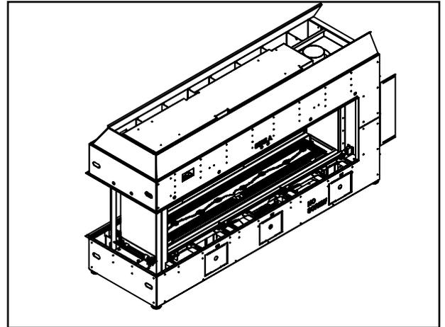
3. Locate the bracket holding the bottom end clamps and loosen the two screws to remove the bracket.
