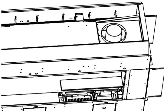
6. Disconnect the cable coming from the pressure regulator motor.
