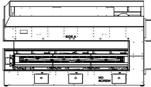
4. Slide in the #6 side panels and secure them by tightening the two screws installed in step 1.
