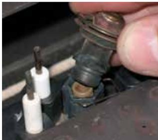
15. Unscrew the pilot orifice with the Allen key, then replace it with the LPG pilot orifice and the pilot cap provided in the kit.
