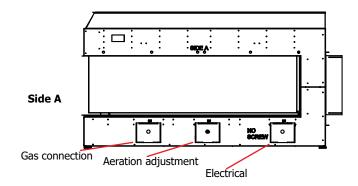
Identify the access panel and remove the corresponding outer trim panel by lifting it up and off (centre panel shown opposite).
