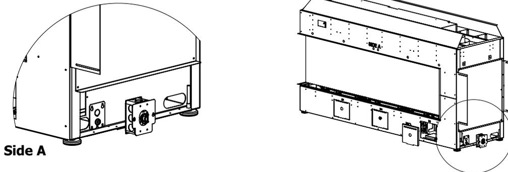
4. Bring the wiring from inside the wall through the opening created when the plate was removed in the previous step.
