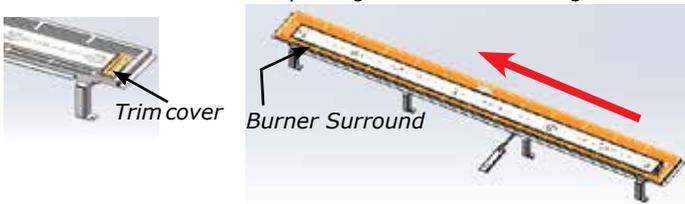
7. Remove eight screws in the locations shown below (four at front and four at rear). Slide the burner to the left, away from the orifice, and lift out.
