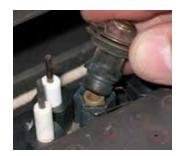
15. Unscrew the pilot orifice with the Allen key, then replace it with the LPG pilot orifice and the pilot cap provided in the kit.
