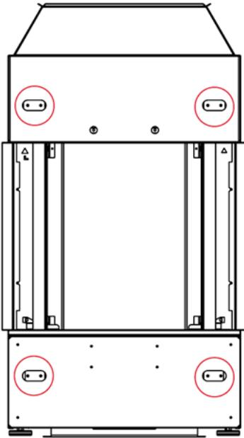
*Access holes for removing transportation*
