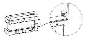
8. Slide the side #5 outer panels between the wall and the barrier stopper bracket. Repeat steps to install the remaining #5 outer panels using a barrier stop where required.
