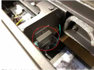
6. Slide the dongle into place with the wires at the top.
