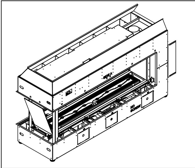
2. Remove Side A and Side B firebox glass panels.
