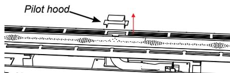
11. Lift off the trim cover on the right side of the burner. Also, remove the burner surround by sliding it to the left and lifting it off.
