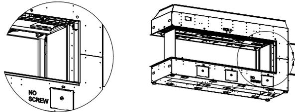
5. Clean panels with a cloth. Add the desired media or logs before installing the inner firebox glass. See this manual for instructions on how to install the firebox glass.
