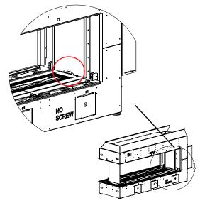
6. Slide the side glass panel #4 into the bottom side bracket.
