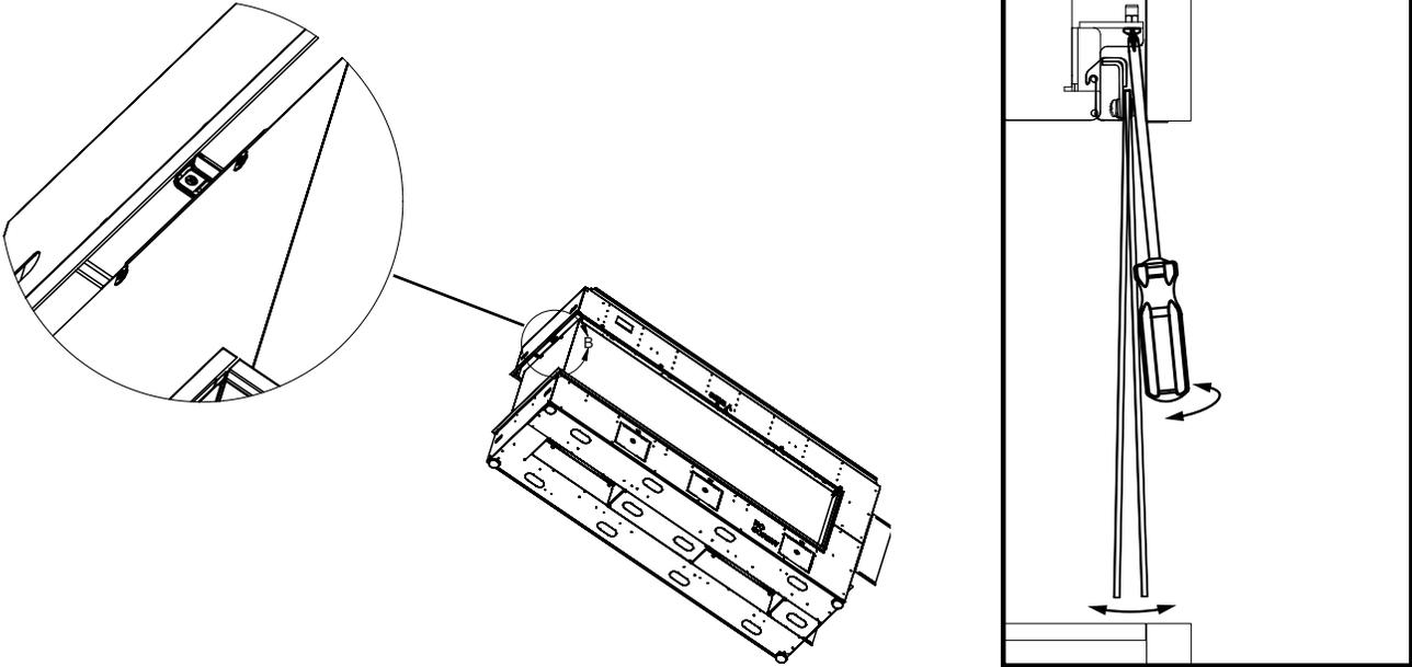
8. Install Side A and Side B barrier glass.
