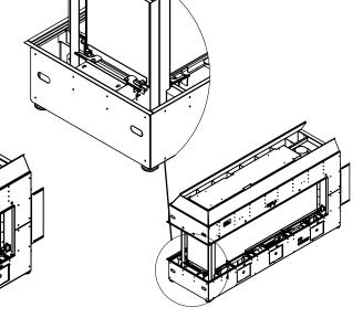
4. Locate the two brackets holding the top end clamps and remove the screws to remove the brackets.
