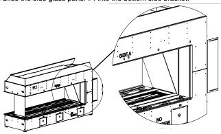
7. Secure side glass by mounting top bracket, then tighten the 2 screws.
