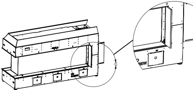
9. Install additional glass stoppers at the end of the unit by sliding the stopper assembly between the unit and panel – the stopper assembly will attach to the unit via a magnet, adjust position of glass stopper if required.
