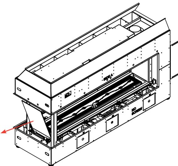
8. Reverse process to reinstall End firebox glass panel.
