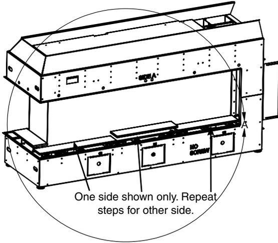
11. Slide the side outer #5 glass panels between the wall and the barrier stopper bracket. If the unit does not have a barrier stopper, stick the side outer panels to the magnets. Repeat steps for the remaining 3 outer sides.
