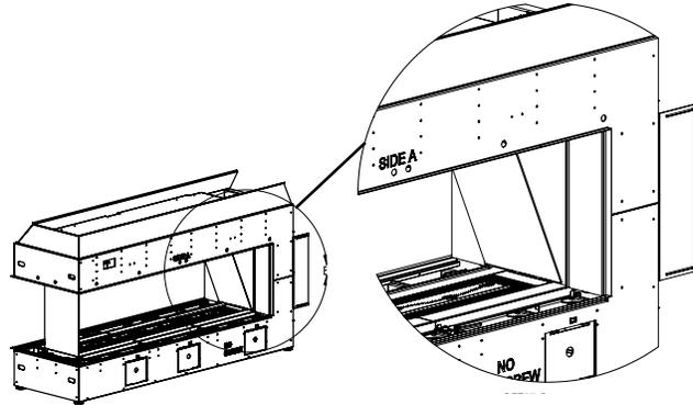
7. Secure side glass by mounting top bracket, then tighten the 2 screws.
