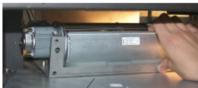
Position Fan B on mounting studs.
