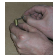
Adjust plunger by turning it to the left or right with a pin.
