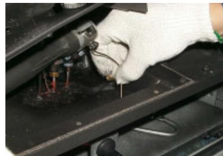
*Note: when installing the burner assembly be sure to slide the aeration adjustment wire through the hole in the base of the burner tray.*
