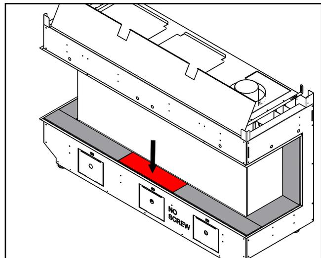
13. Clean the outer panels with a cloth before installing the safety outer barrier glass. To install the safety glass, see this manual for instructions.
