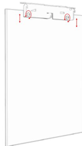
**To adjust the side glass, remove the screws at the top of the panel and move the glass up or down. When the glass is in the correct position, replace and tighten the screws.**
