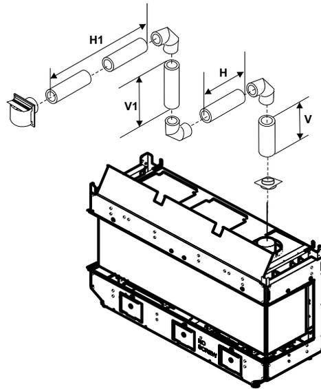
**Vertical Terminations - Rigid Pipe 5" x 8" (Non Power Vent)**
