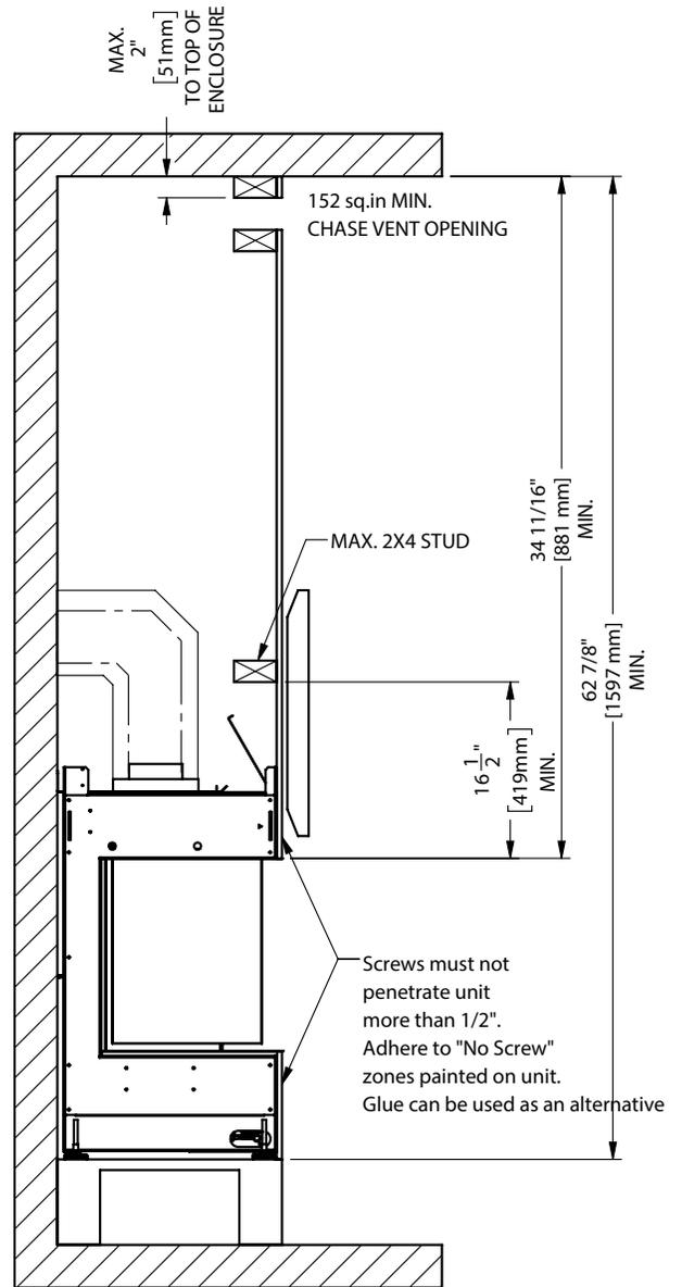
**Note: The TV mounting bracket cannot be secured directly to the appliance. It must be secured to framing. The TV depicted in the picture may need to be higher depending on the style of TV mounting bracket used.**
