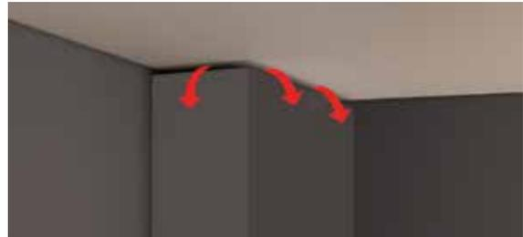
The ventilation opening may be fully open at the top of the enclosure. This type of ventilation opening would be used when the top of the enclosure is not visible from above and where the ceiling within the room is higher than normal. When creating this type of ventilation opening, measures should be in place to avoid having objects of any type falling or be thrown into the ventilation opening. Mesh screen or other preventative measures should be put into place.
