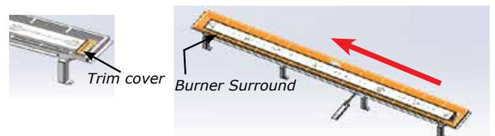
12. Loosen 8 screws in locations shown below (4 at front and 4 at rear)—slide burner to the left away from the orifice and lift out.
