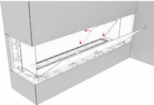
10. Install the inner panel for the corner conversion by wedging it into the inner lower liner panels. **NOTE: The return on the inner panel should be at the top facing inward, and the gasket is facing the side glass.**
