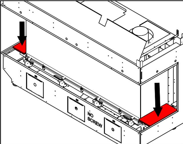
10. Slide the #6 back wall outer panels on both sides as shown below.
