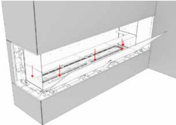
9. Install the back panels by angling the bottom of each panel towards the base of the firebox and then pushing them in.
