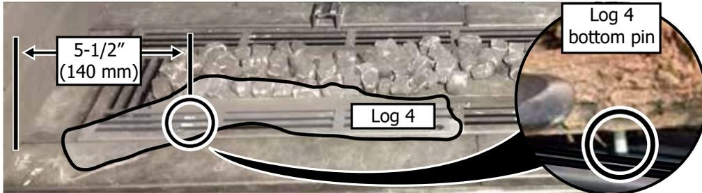
10. Remove the pin on the top of log 4.
