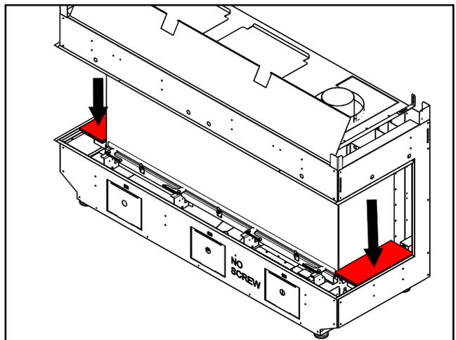
7. Slide the #5 back wall outer panels on both sides as shown below.
