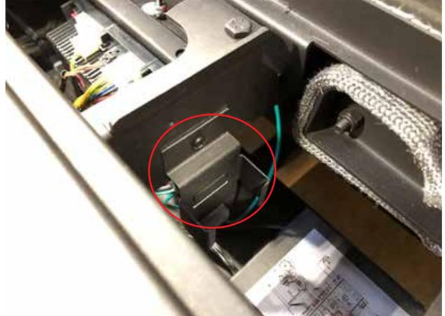
6. Slide the dongle into place with the wires at the top.
