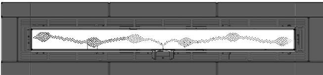
3. Place the various sized fire balls as shown. Ensure the fire balls do not cover any of the burner ports.
