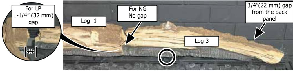
9. Locate the pin on the bottom of log 4. Align the bottom pin of the log 4 onto the burner surround grill using the measurements shown below. Make sure the pin is in the middle slot of the burner surround grill.
