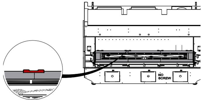
6. Slide the three #4 glass panels into the bottom rear brackets.
