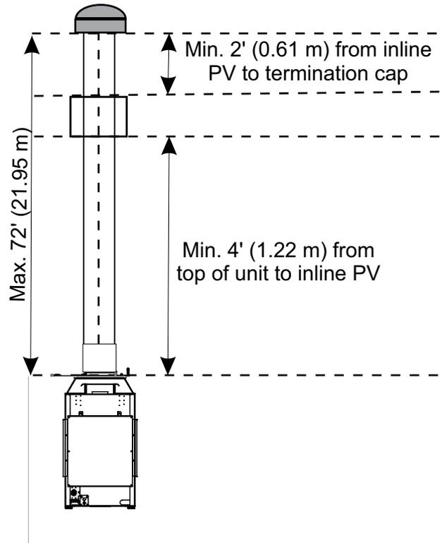
Max. of 72' (21.95 m), using up to six 90° elbows (Note: two 90° elbows shown.)
