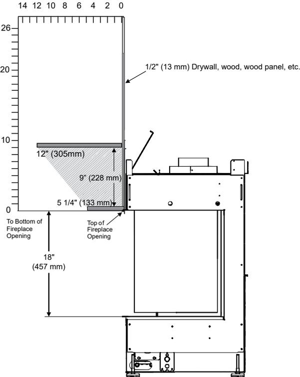
**Mantel Leg Clearances (Non Glass Side When Installed as a Left/Right Corner)**
