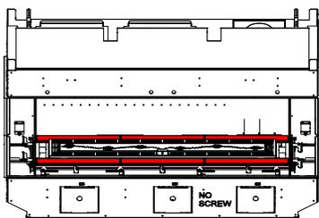
3. Drop the two #2 panels into the firebox on the left and right ends as shown below.
