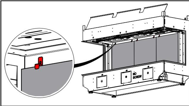
8. Clean panels with a cloth. Add desired media or logs before installing the inner firebox glass. See this manual for instructions on how to install firebox glass.
