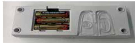
Figure 3: Battery compartment
