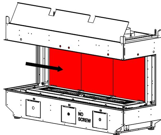
7. Secure the rear glass by mounting top bracket as shown below.
