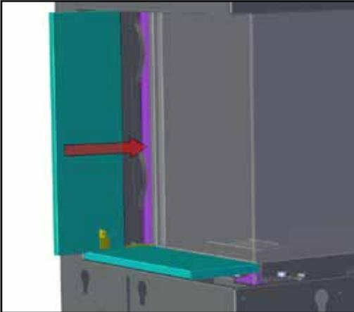
3. Install glass stopper (if desired) by sliding stopper assembly between unit and panel - the stopper assembly will attach to the unit via a magnet, adjust position of glass stopper is required.
