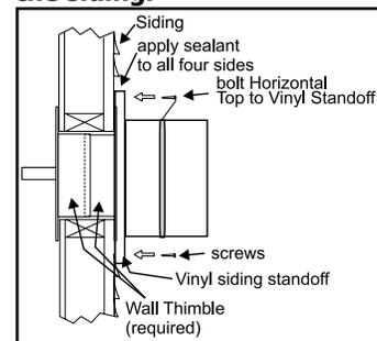
The four wood screws provided should be replaced with appropriate fasteners for stucco, brick, concrete, or other types of sidings.
