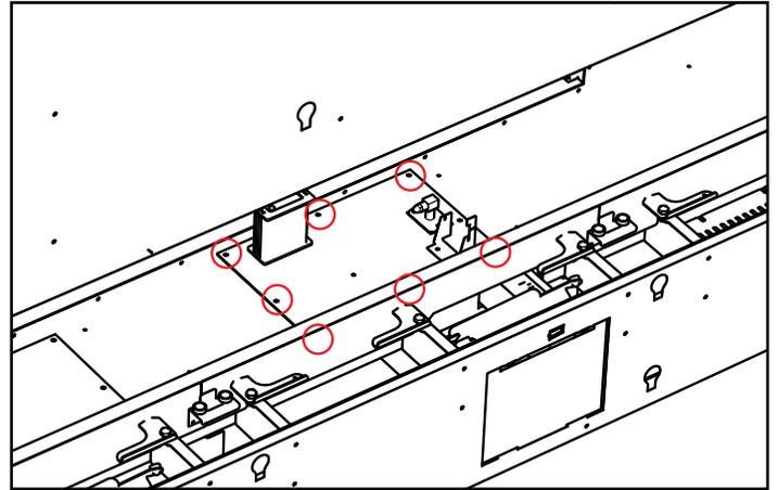
10. Lift valve tray out partially and disconnect flexible gas connection on the valve inlet side, remove valve tray- replace with new valve tray & valve assembly gasket.
