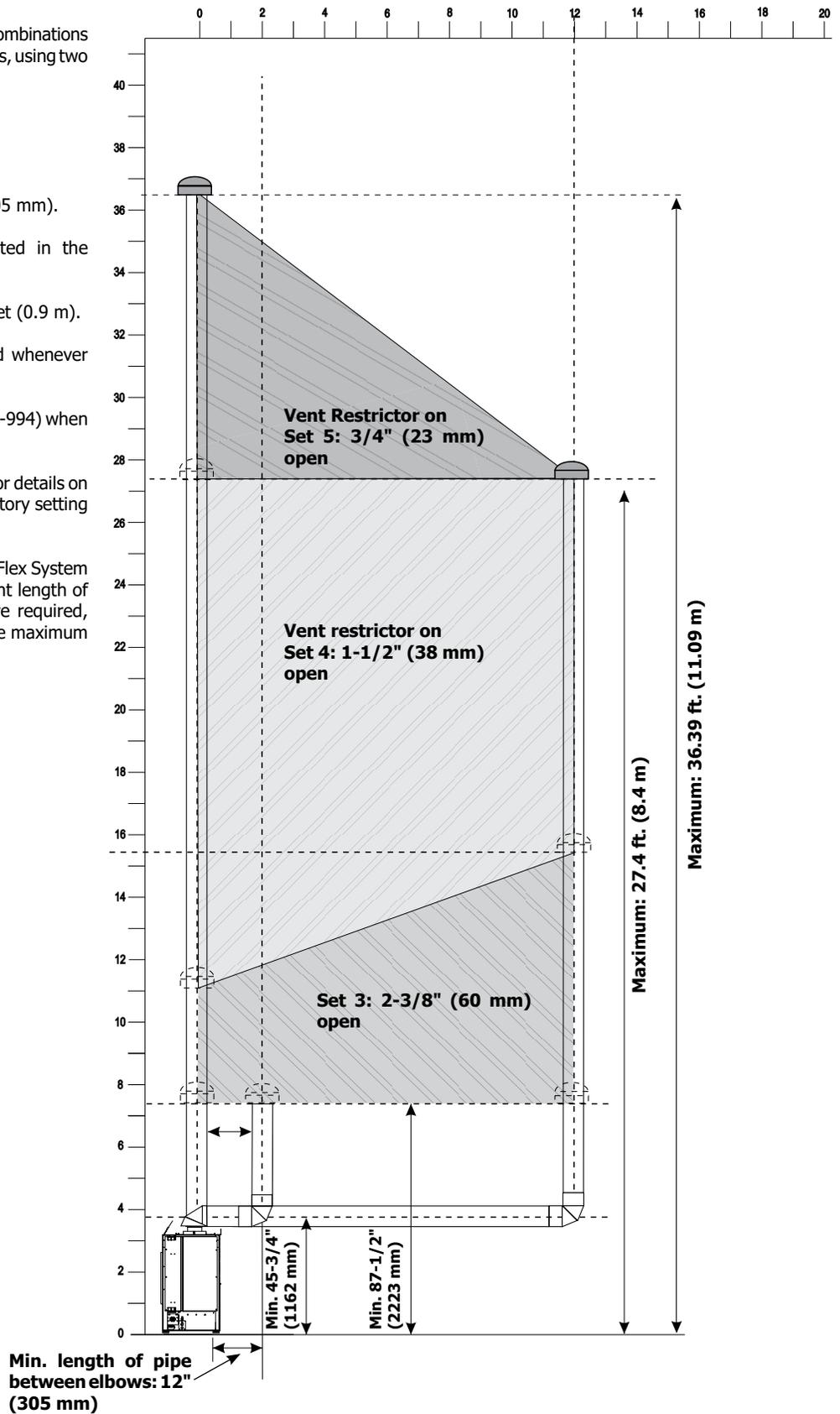
**Vertical Terminations - Rigid/Flex Pipe 5" x 8" (Non Power Vent)**
