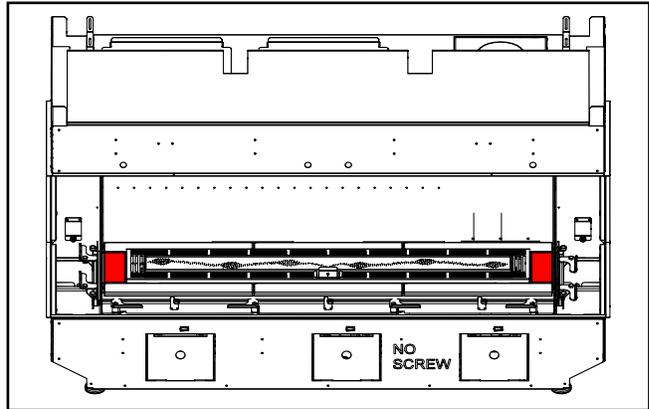
4. Install the 5 screws loosely and install the three #3 panels in the rear of the firebox.
