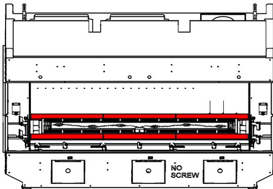
4. Drop the 6 #2 inner glass panels in. The glass panels should be on top of the steel panels. Install the 2 #3 inner side steel panels to the ends of the burner.
