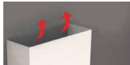
The ventilation opening may be placed on top ensuring it meets the 152 square inch opening. This type of ventilation opening would be used when the top of the enclosure is visible from above and where the ceiling within the room is higher than normal.
