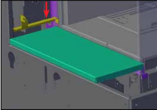
2. Slide backwall outer panel behind glass stopper bracket (if installed).
