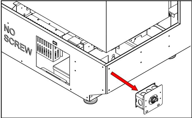
3. Slide electrical box plate towards the back of the unit and then out.
