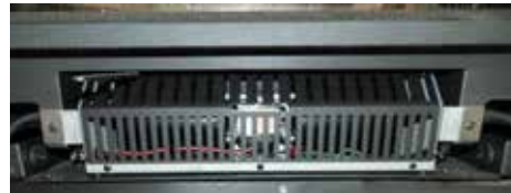
Secure fan with 2 screws removed in Step 1
