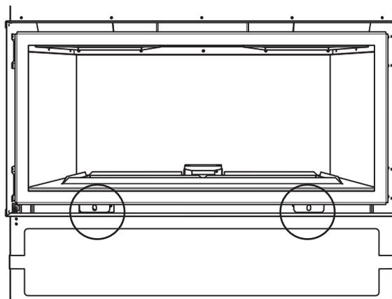
3) Install cover plates over each screw with 2 magnets each as shown below.
