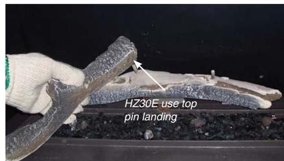
*HZ30E shown - installing Log 2*
