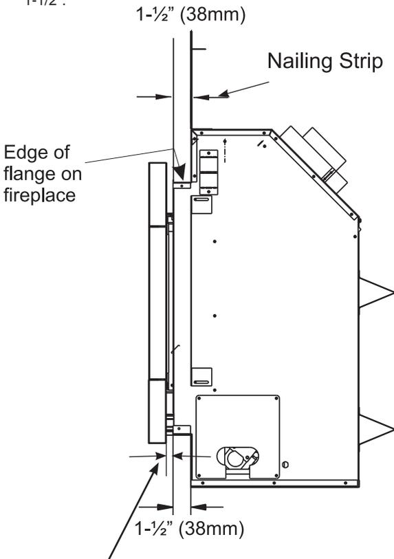
**Important:** 1/2" gap required between faceplate and finished wall when using part #316-924, 316-926, 316-927 (4 pc. faceplate).
