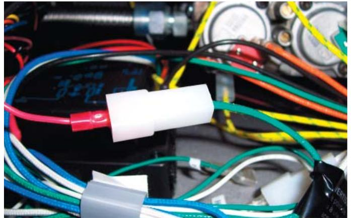
3) Connect one thermostat lead to female connector, using male spade connector - see pic below.
