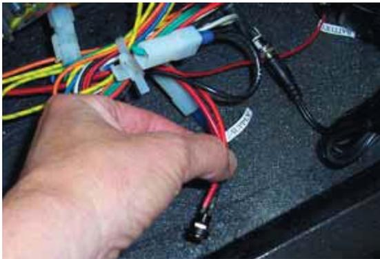
2) Connect the male end from AC adaptor to the female end tagged "DC Supply" on wiring harness in unit.
