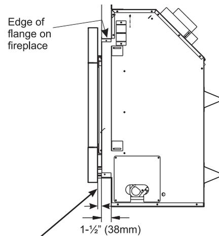
**Important:** 1/2" gap required between faceplate and finished wall when using part #316-924, 316-926, 316-927 (4 pc. faceplate).
