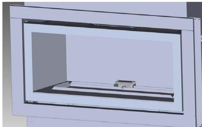
*Completed inner door frame and faceplate installation*
