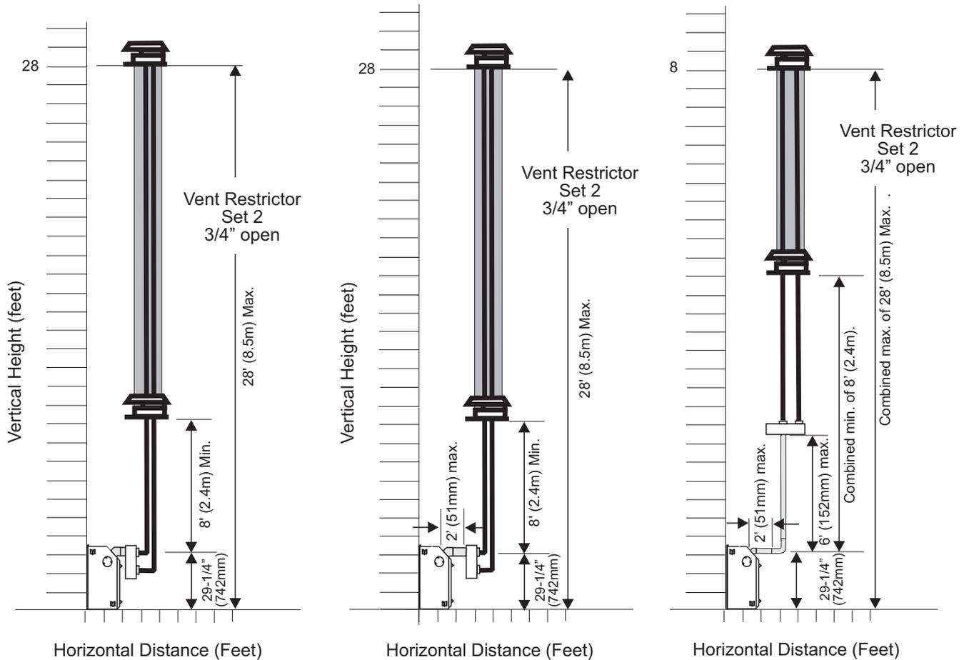
The shaded area in the diagrams show the allowable vertical terminations when using two- 3" co-linear aluminium flex and 4 x 6-5/8" rigid pipe.
