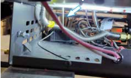
Location of the Aeration Adjustment wire
