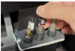
Remove the 2 screws, push Burner Assembly to the left and lift out.
