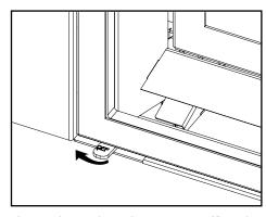
The switch must be in the ON position (flipped to the right) for the remote to turn the unit on. Moving the switch to the left will turn the burner off.
