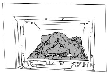
12. Fill the media tray with the 3/4" crushed glass, then scatter the vermiculite, black seawool on top. The glass can cover parts of the front black ember panel (Log #4).
