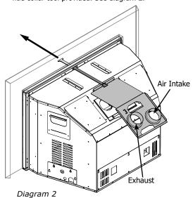
Ensure the draft hood is properly secured and screws tight to create proper seal.
