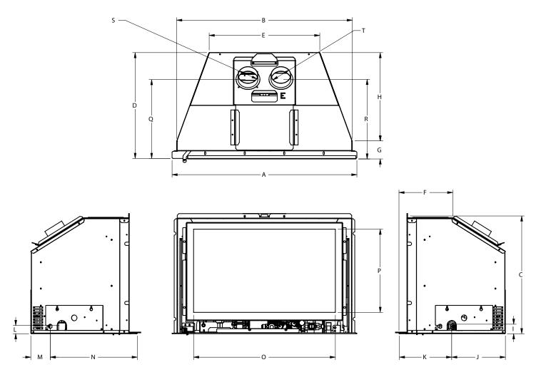
Note: Gas Located on right side of appliance and electrical located on the left hand side of appliance.
