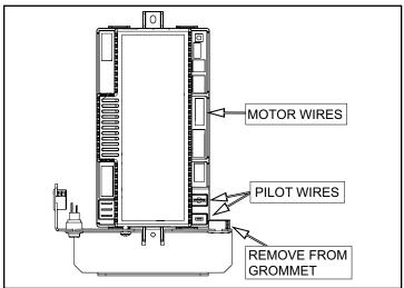
11. Remove the final 7 screws securing the valve tray to the unit and lift the valve tray out. The Valve can then be replaced by removing the 4 screws securing it to the Valve Tray.
