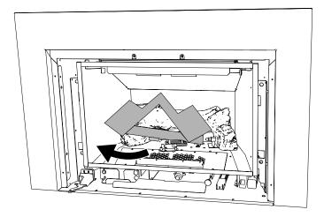
3. Install the rear log #1 and rear brick panel/rear glass panel as shown. The brick & glass panels are not required as this is optional. Only install the rear brick panel if the optional panel set is being installed.
