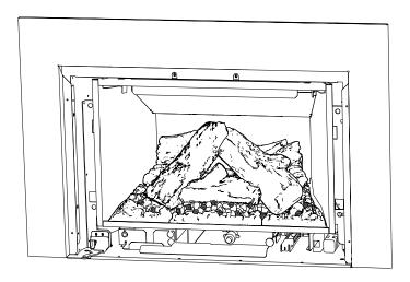
14. Complete the full installation of the logs and media.
