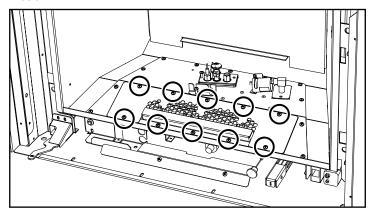
3. Lift the light assembly cover out of the way.
