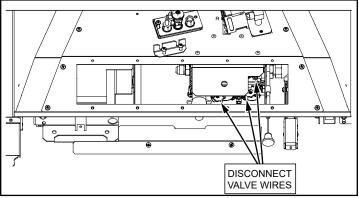
7. Remove the 2 Phillips screws securing the Wire Cover and place in a safe area.
