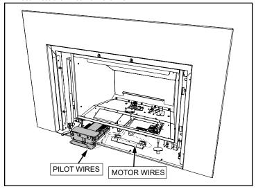
10. Slide the wires through the grommet to remove.
