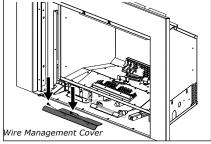
Remove the screw securing the IFC tray and then slid it out to access the motor cable
