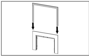
2. If using a Gi25/27 3-Sided Flush Faceplate (262/550-912), place the magnet on face A. One magnet per bracket.
