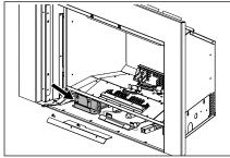
Disconnect the cable coming from the pressure regulator motor at the IFC board (marked X6 on the IFC).
