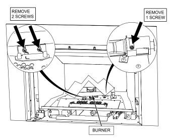
2b. Remove the screw securing the aeration cap and lift burner from the unit.
