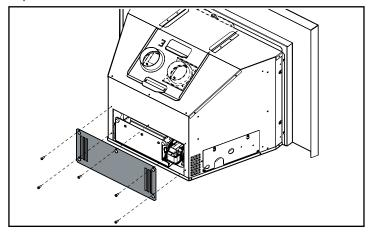
3. Disconnect the fan wire harness through the rear panel. Disconnect 2 x 1/4" spade connectors to the fan terminals. Disconnect the ground lug to the fan using the screw provided.
