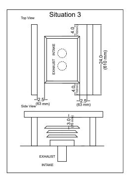
Note: Restrictor must be set to 5" (127 mm) open, see Restrictor Adjustment.
