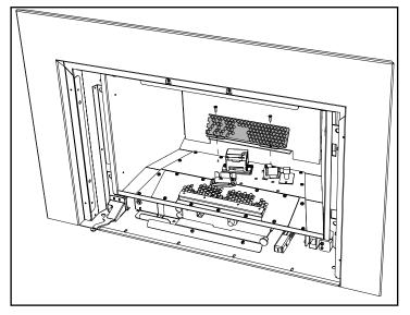
4. Using a Phillips head screwdriver, remove screws securing Pilot Shield in the shown sequence and thenr remove the pilot shield.
