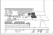
Remove the wire management cover (secured by 2 screws). Remove the wire management straps to access the cables.
