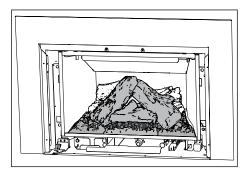
6. Loosen the 2 screws securing the burner to the mount. Remove the 1 screw securing the aeration cap and lift the burner out from the unit.
