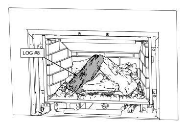
10. If you are using the optional Embaglow (purchased separately) to enhance the flame, sandwich thin, flat layer between the burner and logs #7 and #8. Do not allow the Embaglow fibers to overhang more than 0.25" from the log inner edge.
