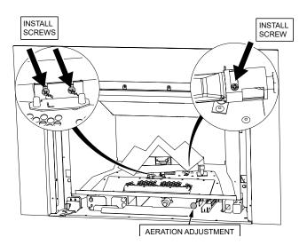
5. Install Log #2, Pilot Log onto the top of the Pilot Shield.
