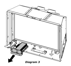
3. Unplug the main power harness (X1) at the PF11 IFC Control Board and disconnect the ground wire from the ground stud.
