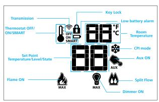
Figure 2: Transmitter LCD Display
