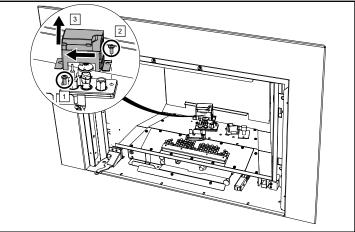
5. Remove the 10 screws securing the light tray and light cover. Disconnect the light wires and then lift and remove the light tray and cover.
