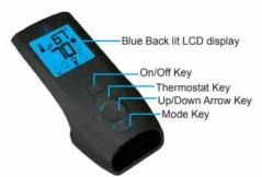
Figure 1: Proflame Transmitter
