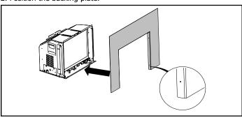
3. Fasten four screws on both sides to attach the backing plate, ensuring they sit at the front of the slots.
