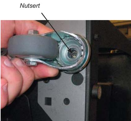
4. Retrofit - Thread bolt into nutsert, hand tighten and finish tightening bolt with supplied allen key.
