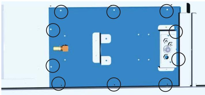
8) Manuover valve assembly up and out.
