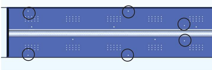
2) Slide the burner to the left and lift out.
