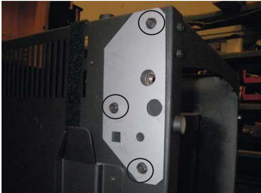
3. Line up caster with existing nutsert (retrofit) or corresponding hole ( see above diagrams) on plate.
