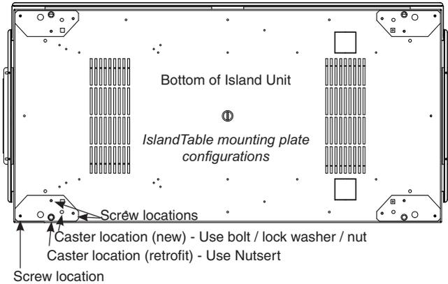
2. Line up mounting plate at each corner on bottom of unit.
