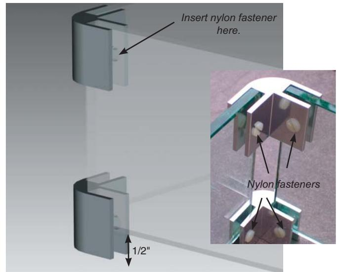
7. Place assembled glass surround on table top - ensure glass is centered on the table top. Once in correct position, lift up one end, apply double sided tape that has been cut to size, to the bottom of the brackets. Repeat process on other end. Press down firmly from to secure glass surround in position. Use care not to scratch surfaces.
