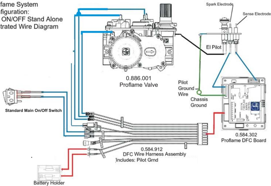
**Important:** The AA batteries in the battery pack operate the burner switch. If the batteries become weak they will need to be replaced with quality alkaline batteries. This unit will not operate without AA batteries.
