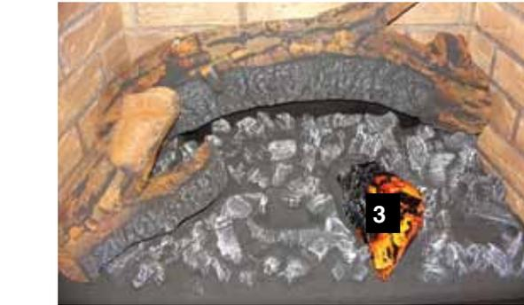
8) Locate provision in the bottom of Log 4 (see highlighted areas below) and place provision on the burner.
