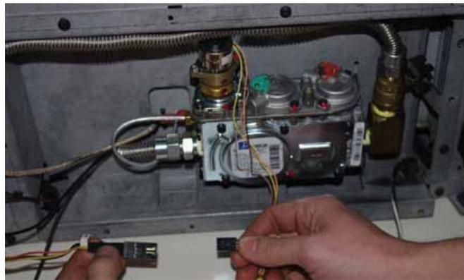
4) Remove and discard 2 Pressure regulator screws A (T20 or slot), Pressure Regulator B, Spring and Diaphragm C.
