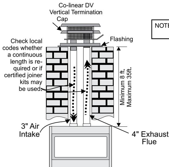
**NOTE:** Flashing should be securely fastened to the chimney.
