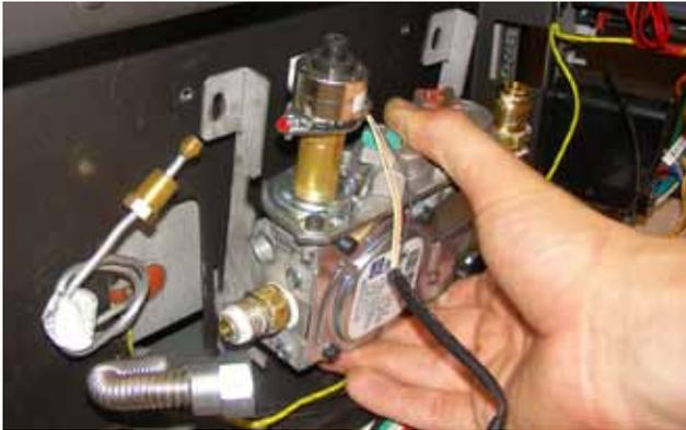
9) Secure the Valve Assembly by the 90 Elbow Fitting in a sturdy table vice. Using a crescent wrench, loosen the valve from the Elbow fitting.
