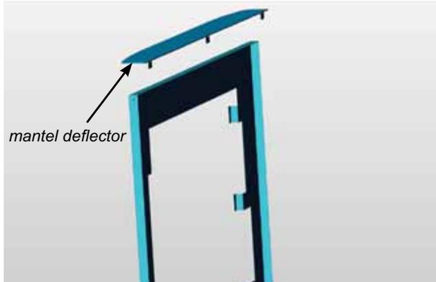
Flip all 3 tabs 90° to secure the deflector to the top of the backing plate. The tabs should be flush with the underside of the top lip of the back plate.
