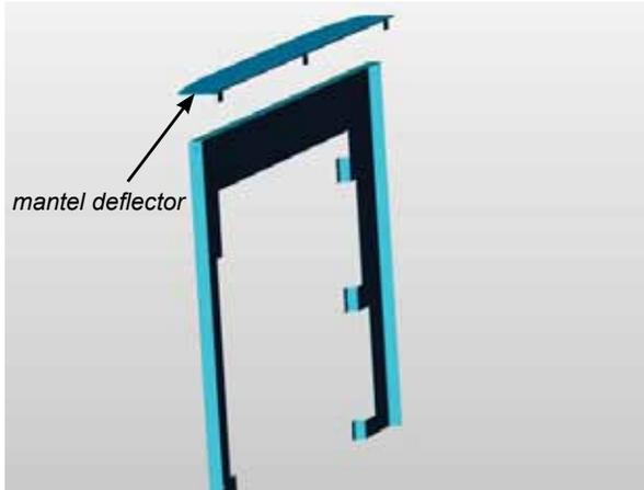
Bend all 3 tabs 90° to secure the deflector to the top of the backing plate. The tabs should be flush with the underside of the top lip of the back plate.
