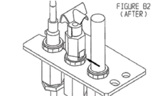
11) Re-tighten the pilot target hex fitting until the pilot target aligns with the flame sensing rod.
