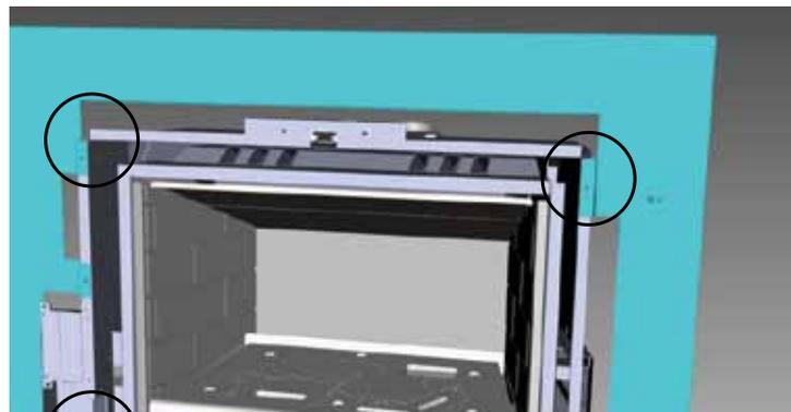
4) Install front faceplate and secure to the unit with 4 screws in locations shown below.
