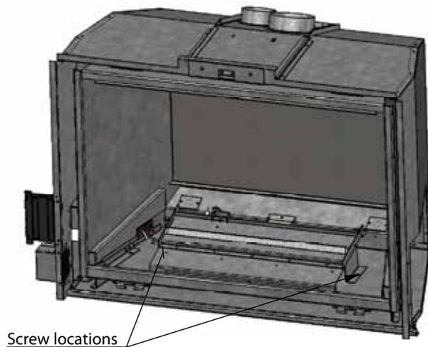
**L540EB CERAMIC BURNER REMOVAL / INSTALLATION**
