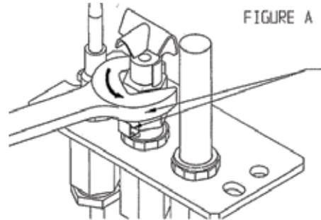
10) Push the Orifice strip tab all the way against the hex fitting as shown on the right.
