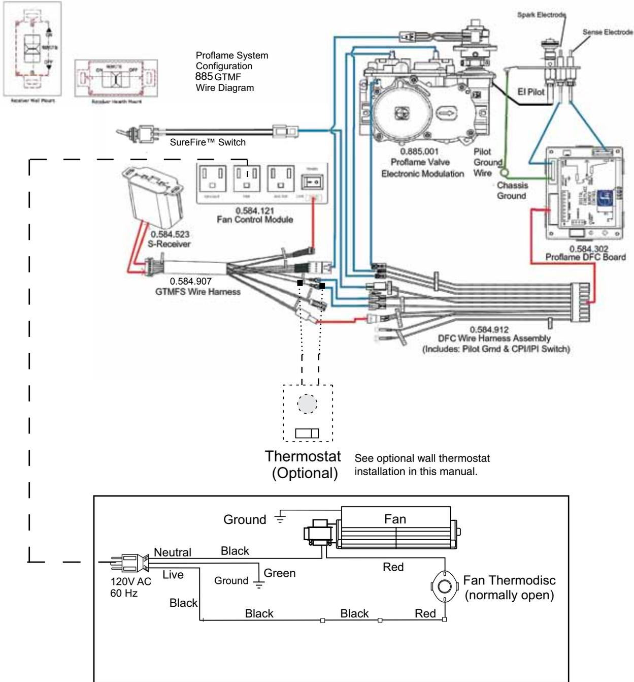
**GTMF REMOTE SYSTEM - IMPORTANT:** The 120V fan control module serves as the power source for this unit. The AA batteries in the receiver only serve as a backup in case 120 volt power lost within the home.
