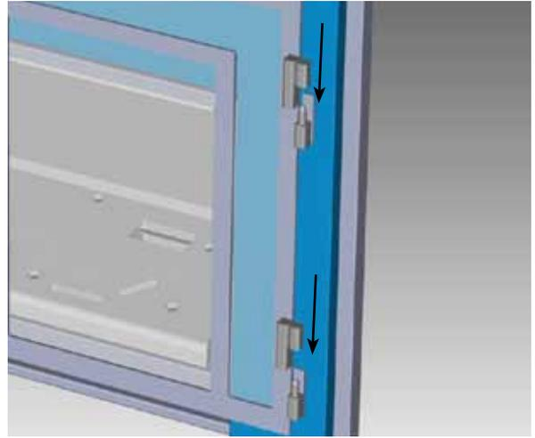
5) Install the supplied bracket in the center of the low lip on the unit base - secure with 2 clips as shown below.
