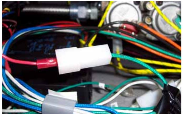
3) Connect one thermostat lead to female connector, using male spade connector - see pic below.
