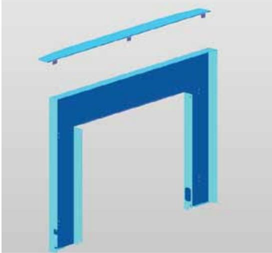
2) Bend all 3 tabs 90° to secure the deflector to the top of the frame. The tabs should be flush with the underside of the top lip of the back plate.
