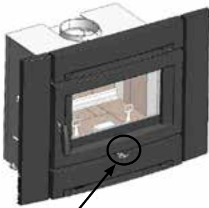
Primary Air Damper Left - Open Right - Closed
