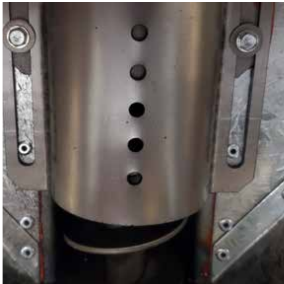
Hopper Auger Cover. Factory setting two closed holes and 3 open
