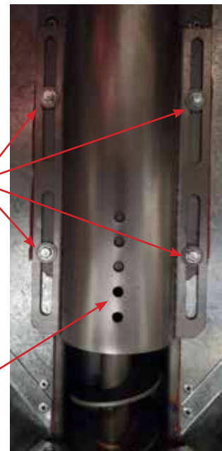
Hopper Auger Cover. Adjusted to accommodate larger pellets.
