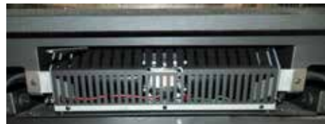
Secure fan with 2 screws removed in Step 1
