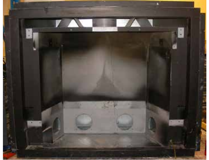
Diagram 8.12 Modified edges must be flush to allow proper seating of the E18E outerbox.
