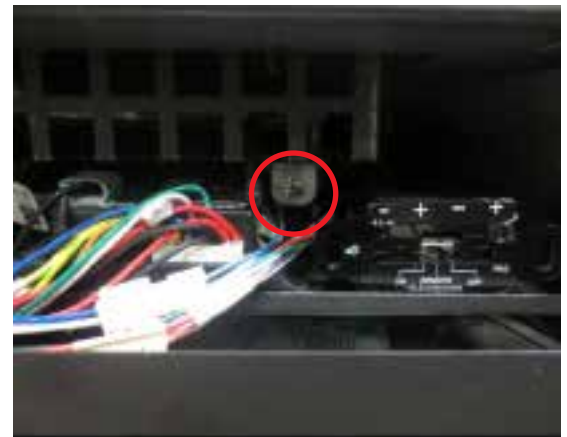
The Surefire switch is located at the bottom right above the DFC board.
