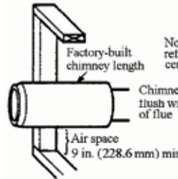
Minimum chimney clearance from masonry to sheet steel supports and combustibles 2 in. (50.8 mm)
