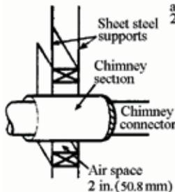
Minimum chimney clearance to sheet steel supports and combustibles 2 in. (50.8 mm)
