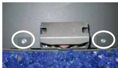
Burner screws on E33S
