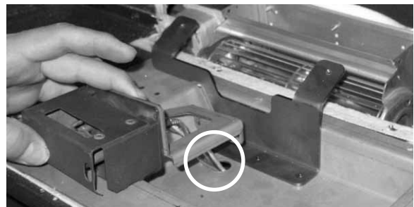
Pilot assembly wires
