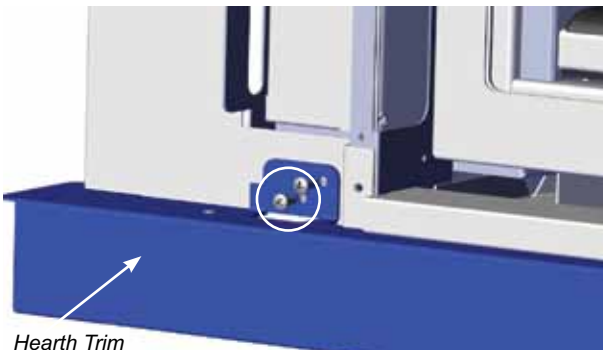
Diagram 3—Hearth Trim Secured to Backing Plate
