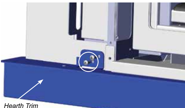
Diagram 3—Hearth Trim Secured to Backing Plate
