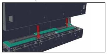
2. On back of firebox wall--install 6 screws (loosely) in locations shown below. Install 3 back panels--hang panels on installed screws through keyhole opening.
