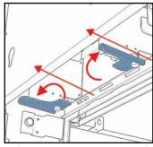
Clamps in open position, rail pulled forward
