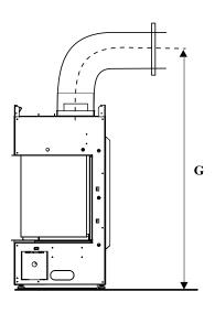
Note: Unit must be installed onto a solid back wall - do not install directly onto studs.
