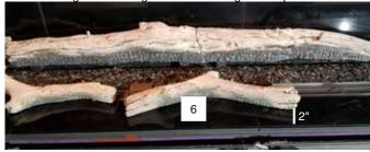
12. Insert the pin of Log 7 into the hole on the right-most side. Position the left end of the log 1-1/8" from edge of panel, as shown below.
