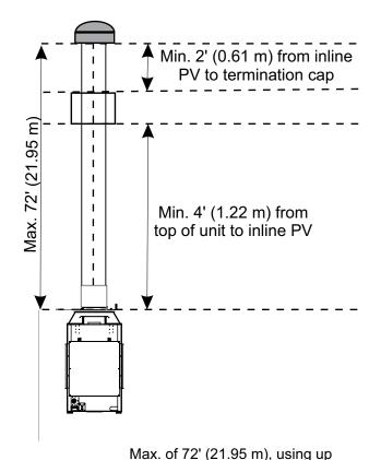
to six 90° elbows (Note: two 90° elbows shown.) 1/4" Flex Vent " to C/L Rigid Vent Min. 2' (0,61 m) from inline I to termination cap Min. 4' (1.22 m) from top of unit 55' 1/4" to inline PV Min. 59'
