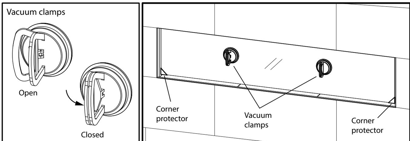
4. Using the vacuum clamps, lift the barrier straight up, pull it toward you, then gently lower it straight down (see below).
