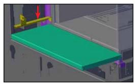
2. Slide backwall outer panel behind glass stopper bracket (if installed).
