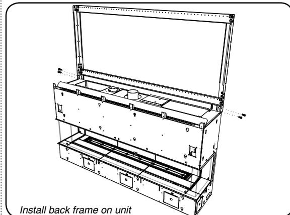
2. Install the frame assembled in Step 1, onto the back of the unit as shown above with 2 screws on each side.
