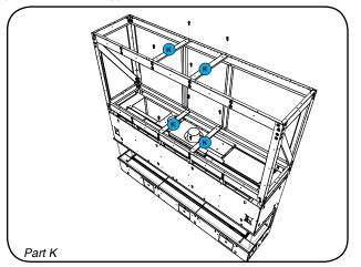
12. Install 4 front supports (Part C) to upper and lower Part A with 2 screws on each end. Before installing Part C, turn it so that the screw holes are at the top.
