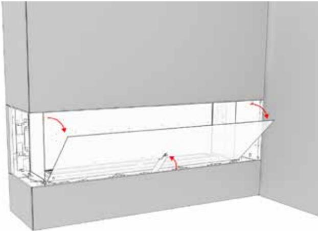
8. Install lower inner liner panels.
