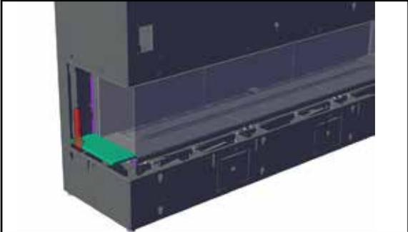
12. Install glass stopper (if desired) by sliding down the outside of the outer side panel.
