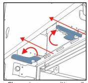
Clamps in open position, rail pulled forward
