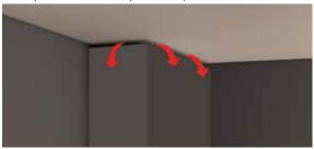
The ventilation opening may be fully open at the top of the enclosure. This type of ventilation opening would be used when the top of the enclosure is not visible from above and where the ceiling within the room is higher than normal. When creating this type of ventilation opening, measures should be into place to avoid having objects of any type falling or be thrown into the ventilation opening. Mesh screen or other preventative measures should be put into place.
