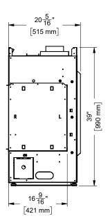
Note: Height Dimension is taken with leveling legs fully inserted and may vary depending on the height of the leveling legs, when unscrewed or extended.
