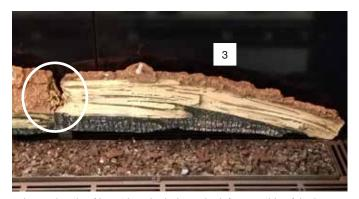
9. Insert the pin of Log 4 into the hole on the left-most side of the burner. The right end of Log 4 should sit 1-1/4" from the edge of the panel,
