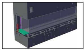
12. Install glass stopper (if desired) by sliding down the outside of the outer side panel.
