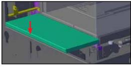
13. Slide backwall outer panel (13) behind glass stopper bracket (if installed).
