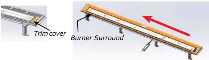
7. Remove 8 screws in locations shown below (4 at front and 4 at rear)—slide burner to the left away from the orifice and lift out.
