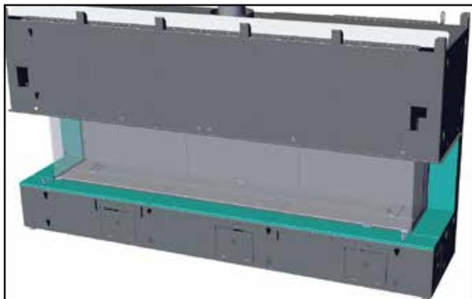
8. With panel set installed -- complete by installing barrier glass.
