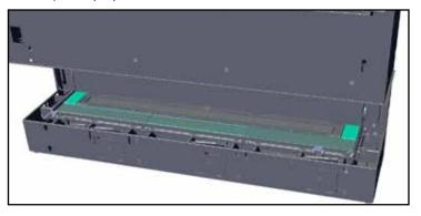
Install four back panel brackets in between the back wall and the burner tray. Line up the center of the middle brackets with the base panels installed in the previous step as shown below.
