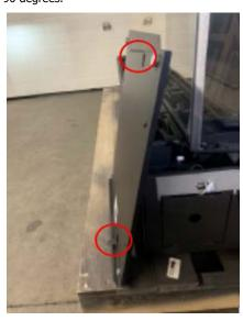
Tighten screws with screwdriver.
