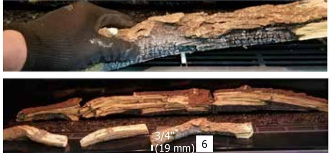
12. Insert the pin of Log 7 into the hole on the right-most side of the burner. Position the left end of Log 7 1-5/8" from edge of panel, as shown below.
