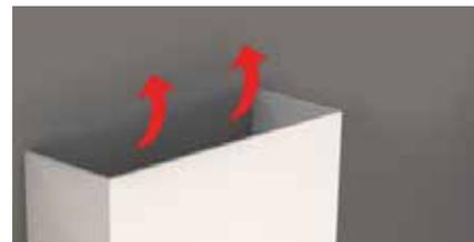
The ventilation opening may be placed on top ensuring it meets the 180 square inch opening. This type of ventilation opening would be used when the top of the enclosure is visible from above and where the ceiling within the room is higher than normal.
