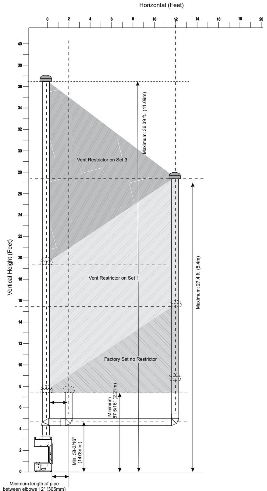
**Vertical Terminations - Rigid/Flex Pipe 5" x 8" (Non Power Vent)**
