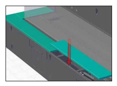
6. Install glass stopper (if desired) by sliding stopper assembly between unit and panel - the stopper assembly will attach to the unit via a magnet, adjust position of glass stopper is required.
