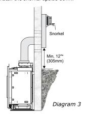
\*As specified in CSA B149.1 Installation Code. Local codes or regulations may require different clearances.
