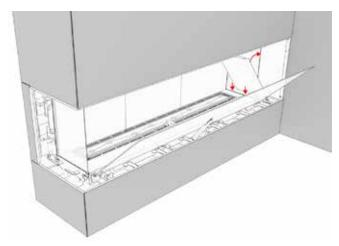
11. Slide the inner side panel in by wedging it between the side glass and the back liner panels.
