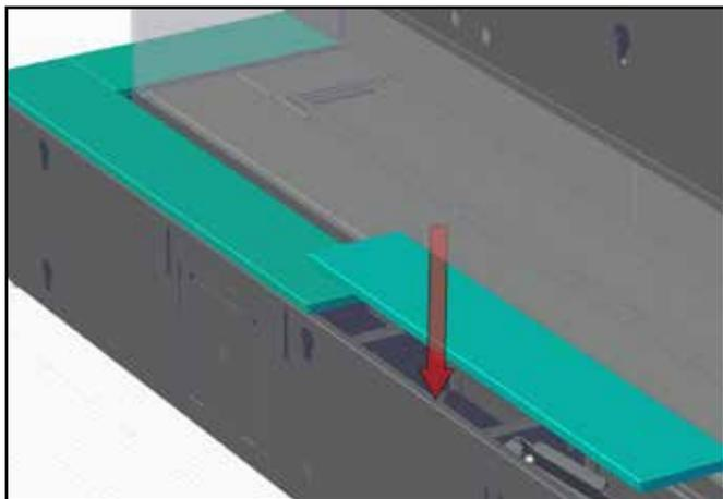
6. Install glass stopper (if desired) by sliding stopper assembly between unit and panel - the stopper assembly will attach to the unit via a magnet. Adjust position of glass stopper as required.
