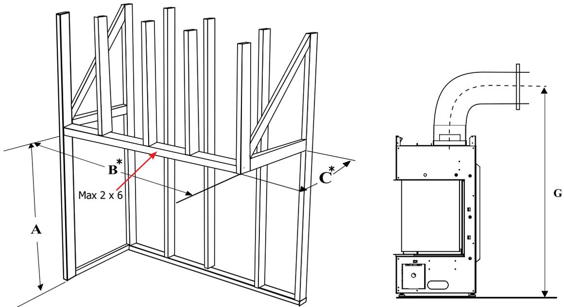
Note: This appliance must be installed on a level and solid surface such as a plywood floor which must be the full width and depth of the appliance.
