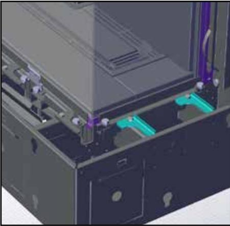
2. Pull glass gasket pad forward to release glass.
