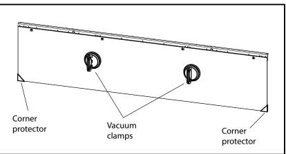
5. Holding the glass barrier in front of the unit, slide it up behind the top lip of the unit. Lift the barrier up as far as it goes, then hook the barrier onto the unit.
