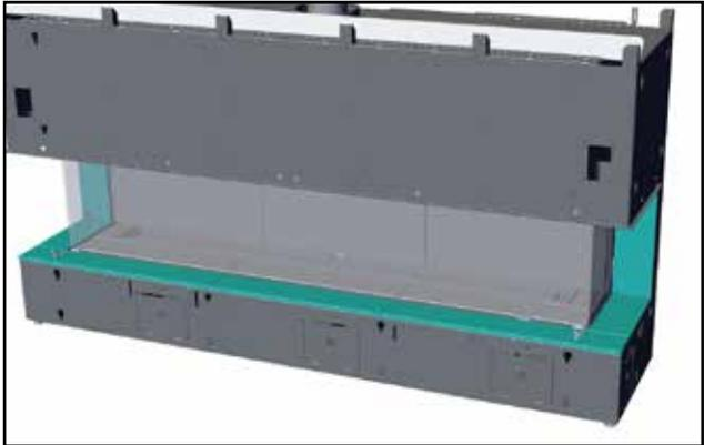
18. After complete panel set installed -- complete by installing barrier glass.
