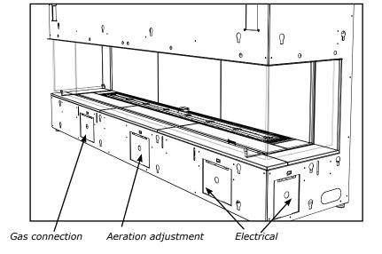
Identify access panel to be removed, remove corresponding outer trim panel by lifting up and off (centre panel shown below).
