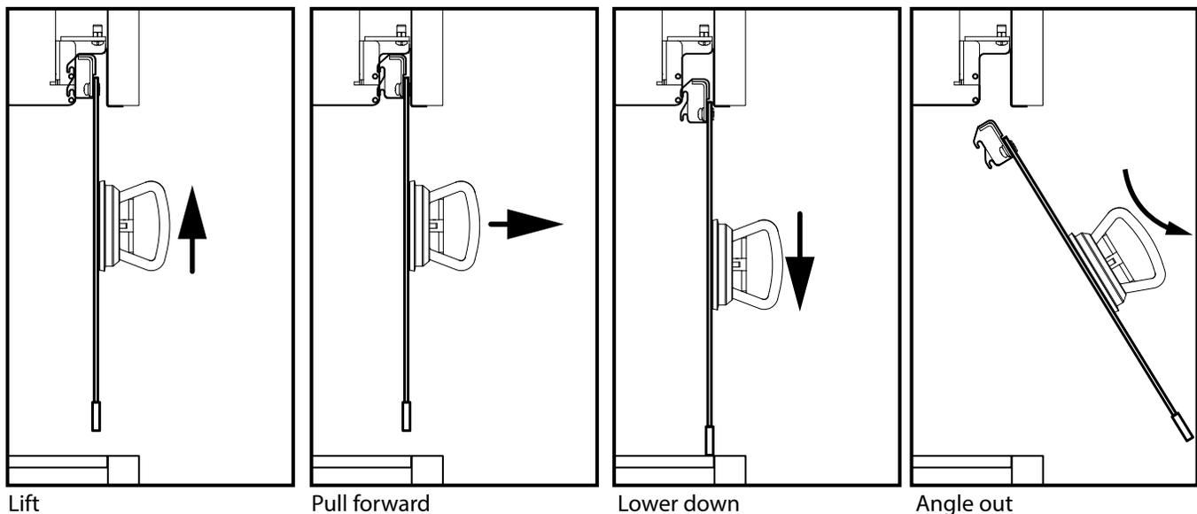
5. Angle the bottom edge toward you and carefully lift the glass barrier out, placing it on your prepared soft, scratch resistant surface (i.e. drop cloth).
