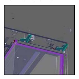
4. Gently move bottom of side glass panel into the support channel as shown in diagram below.
