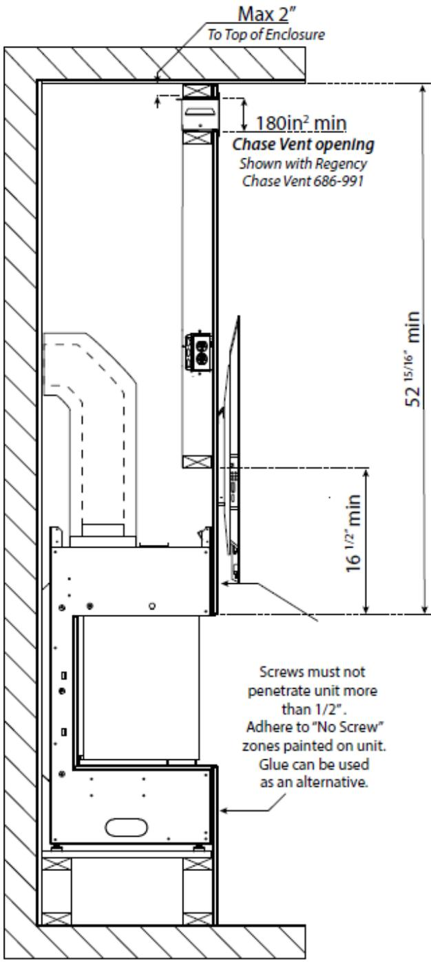
Note: The TV mounting bracket cannot be secured directly to the appliance. It must be secured to framing. The TV depicted in the picture may need to be higher depending on the style of TV mounting bracket used.
