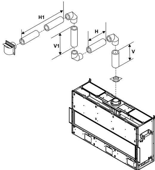
**Vertical Terminations - Rigid Pipe 5" x 8" (Non Power Vent)**
