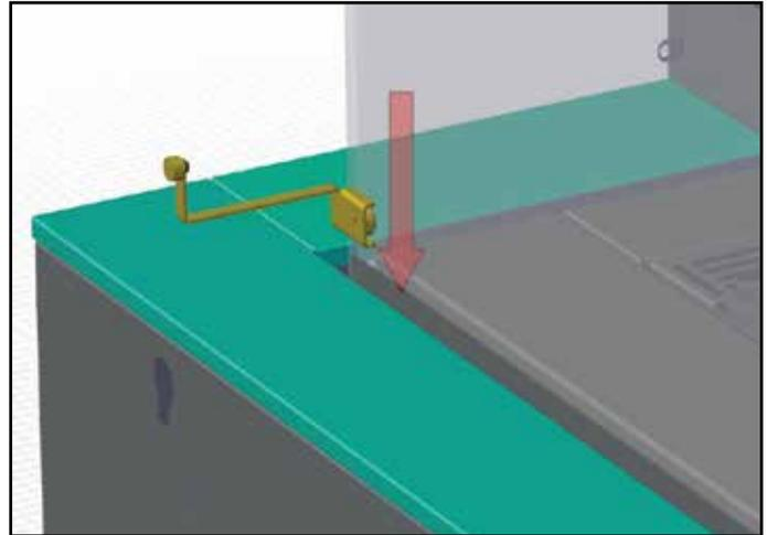
4. Install front end panel-place on unit as shown below.
