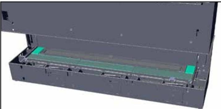
6. Install four back panel brackets in between the back wall and the burner tray. Line up the center of the middle brackets with the base panels installed in the previous step as shown below.
