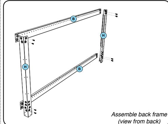
1. Assemble the back frame as shown above by assembling 2x Part B with 2x Part H with 8 screws installed from back of frame.
