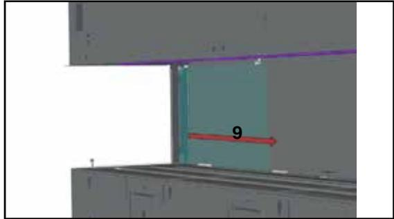
8. Secure the top of the panel brackets with 2 screws into 2 brackets (each panel has 2 brackets).
