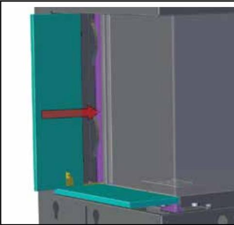
6. Install glass stopper (if desired) by sliding stopper assembly between unit and panel - the stopper assembly will attach to the unit via a magnet, adjust position of glass stopper is required.
