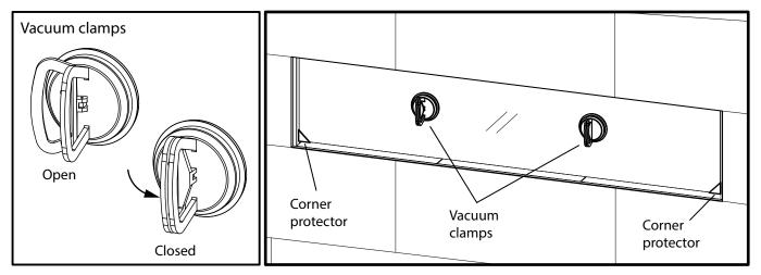
4. Using the vacuum clamps, lift the barrier straight up, pull it toward you, then gently lower it straight down (see below).
