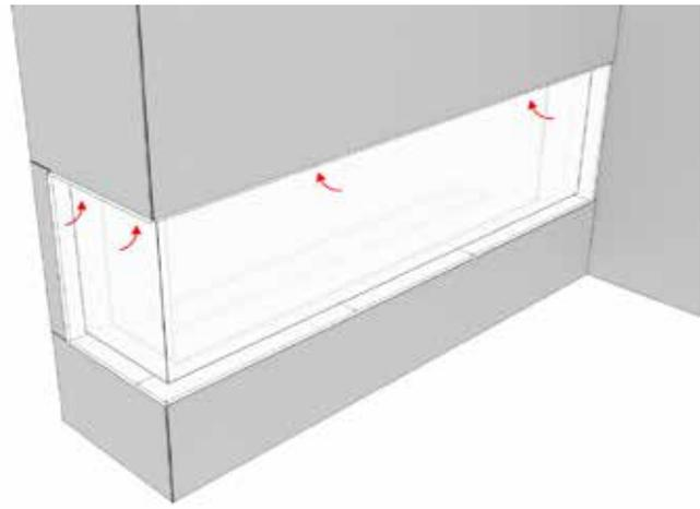
15. Slide the corner panel up and in to secure it.
