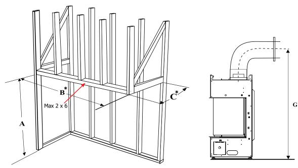
Note: This appliance must be installed on a level and solid surface such as a plywood floor which must be the full width and depth of the appliance.
