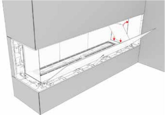
11. Slide the inner side panel in by wedging it between the side glass and the back liner panels.
