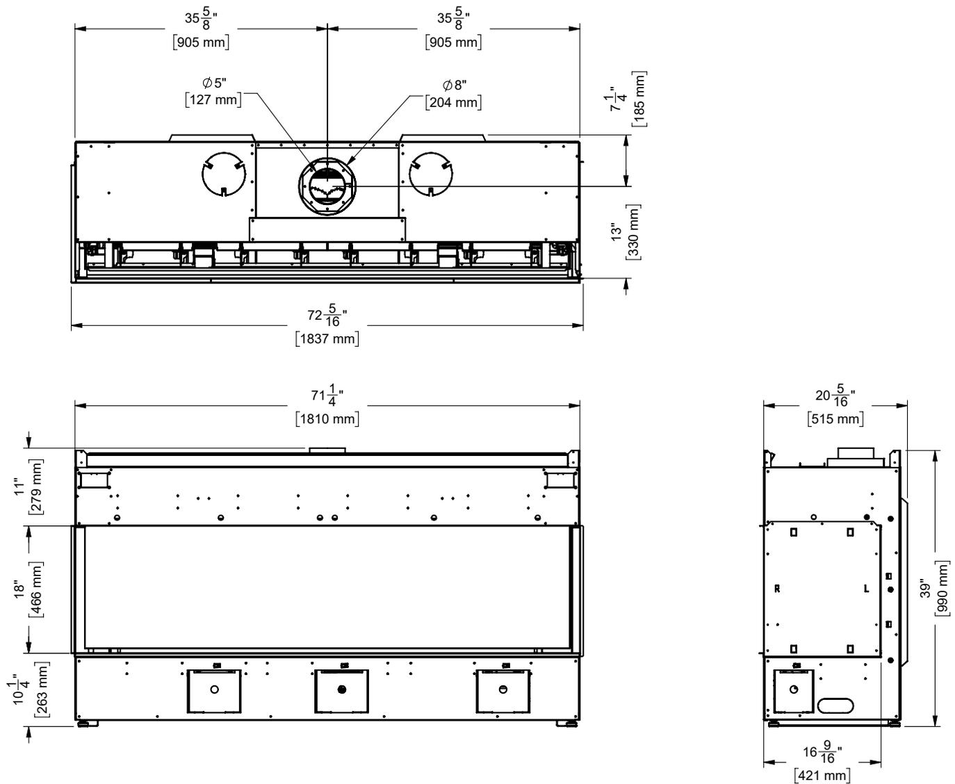
Note: Height Dimension is taken with leveling legs fully inserted and may vary depending on the height of the leveling legs, when unscrewed or extended.
