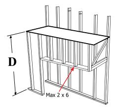
Note: Unit must be installed onto a solid back wall - do not install directly onto studs.
