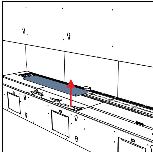
2. From inside the unit—push in tab to release the access panel at the top.
