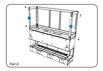
9. Attach end cross braces (Parts E + F) with 2 screws at each end as shown below.
