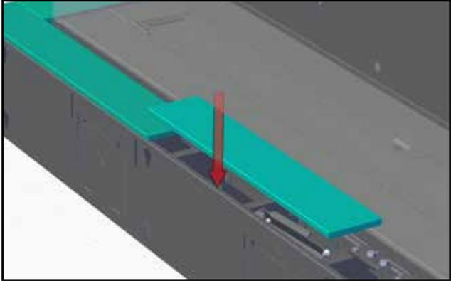
16. Install glass stopper (if desired) by sliding stopper assembly between unit and panel - the stopper assembly will attach to the unit via a magnet, adjust position of glass stopper is required.
