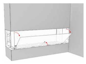
8. Install lower inner liner panels.
