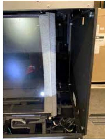
2. Install trim guide for left or right install to the outer side panel.
