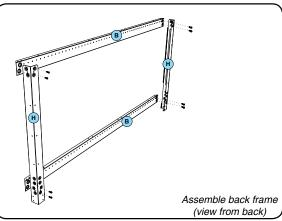
1. Assemble the back frame as shown above by assembling 2x Part B with 2x Part H with 8 screws installed from back of frame.
