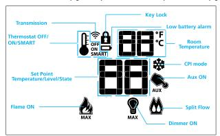
Figure 1: Transmitter LCD Display
