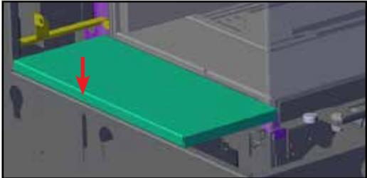
13. Slide backwall outer panel (13) behind glass stopper bracket (if installed).
