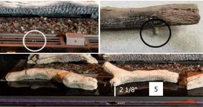
11. Insert the pin of Log 6 into the hole on the right side of the pilot. Position the right end of Log 6 2" from the edge of the panel.
