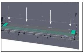
7. Carefully manoeuvre the back glass panels (9,10,11) to the back wall of the firebox. Start with back panel 9 -- place two panel brackets on each panel and manoeuvre into position, sliding the bottom into the corner and back brackets.
