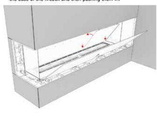
10. Install the inner panel for the corner conversion by wedging it into the inner lower liner panels. NOTE: The return on the inner panel should be at the top facing inward, and the gasket is facing the side glass.
