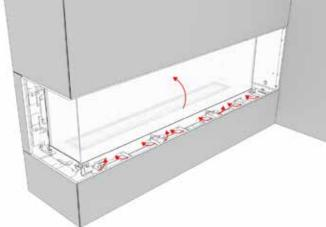
14. Install outer liner panels - there will be two left over.
