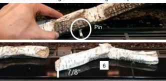
12. Insert the pin of Log 7 into the hole on the right-most side of the burner. Position the left end of Log 7 1/2" from edge of panel, as shown below.
