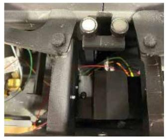
2. Remove the screw and pull the cover off.
