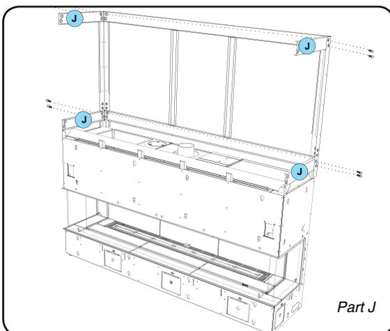
8. Attach 2 x Part G to the previously installed Part J parts with 2 screws at each end.
