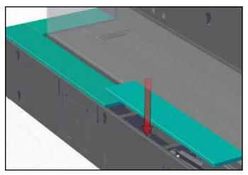
6. Install glass stopper (if desired) by sliding stopper assembly between unit and panel - the stopper assembly will attach to the unit via a magnet, adjust position of glass stopper is required.
