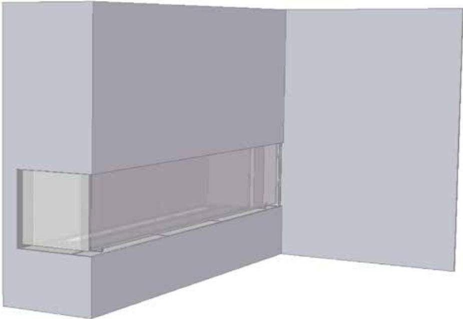
1. Decide on Left or Right install - Install outer panel of corner conversion before placing unit in framing.
