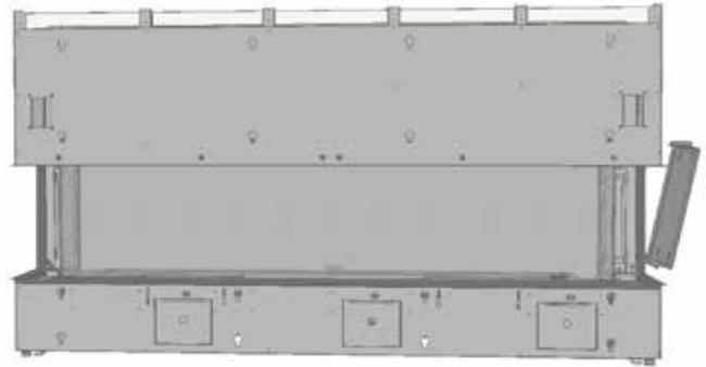
6. Screw in the two self-tapping screws to the top of the outer side panel. Unit can be placed in framing at this point.
