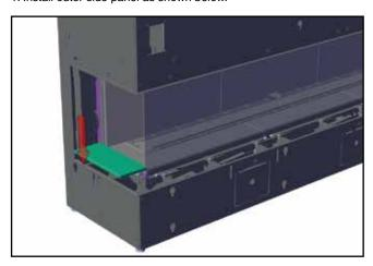
2. Install glass stopper (if desired) by sliding down the outside of the outer side panel.
