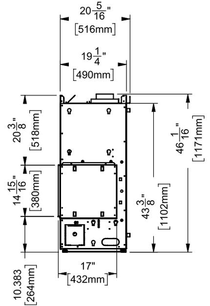
Note: Height Dimension is taken with leveling legs fully inserted and may vary depending on the height of the leveling legs, when unscrewed or extended.
