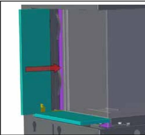
3. Install glass stopper (if desired) by sliding stopper assembly between unit and panel - the stopper assembly will attach to the unit via a magnet, adjust position of glass stopper is required.
