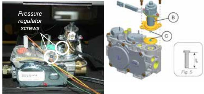
9. Re-attach the Pressure Regulator wire (disconnected in Step 6), and re-situate the IFC, secure the screws that fasten the IFC Mounting Brackets.
