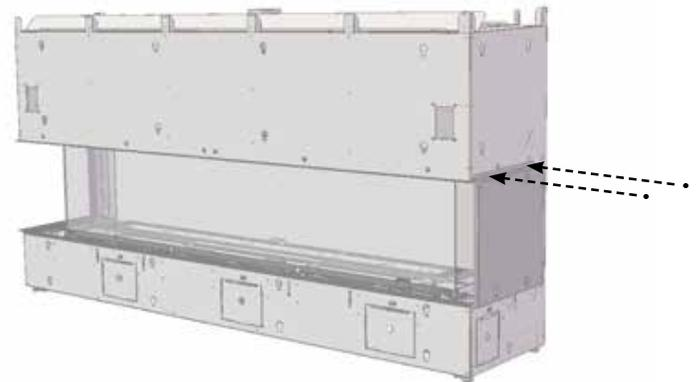
7. See inner panel install section. Once firebox panels are installed, then install corner conversion liner panel inside of side barrier glass. Note: Gasket side of panel sits against the glass and the flange sits at top.
