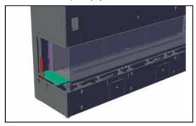
12. Install glass stopper (if desired) by sliding down the outside of the outer side panel.
