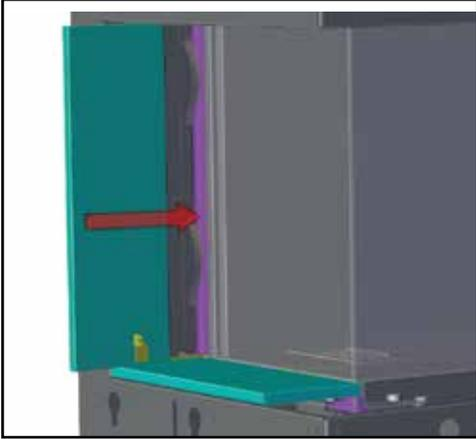
4. Install front end panel-place on unit as shown below.
