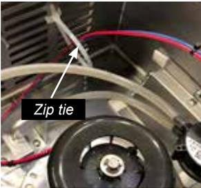
4. Install the second zip tie loosely on the bracket behind the pressure switch. Run the motor wires through the zip tie.
