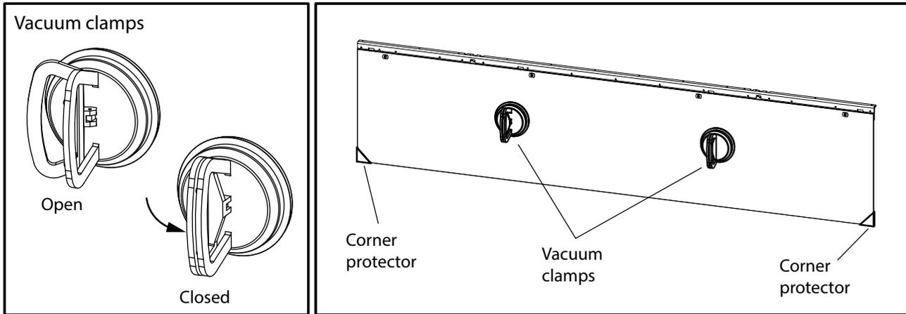
5. Holding the glass barrier in front of the unit, slide it up behind the top lip of the unit. Lift the barrier up as far as it goes, then hook the barrier onto the unit.
