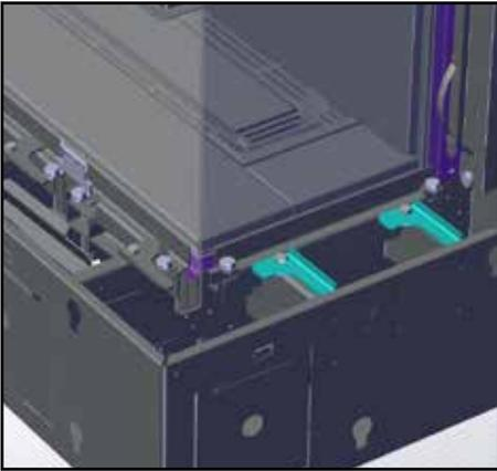
2. Pull glass gasket pad forward to release glass.
