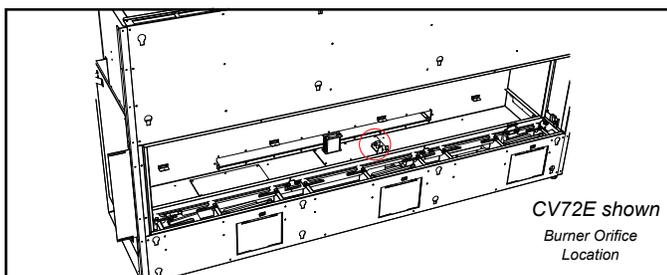
15. Remove pilot retainer clip with pliers and pull off the pilot cap to expose the pilot orifice.
