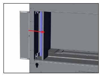
2. Slide the stopper bracket in between the front panel and the unit wall as shown.
