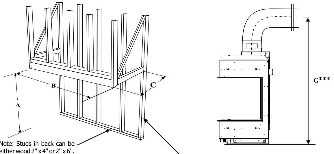
Note: Studs in back can be either wood 2" x 4" or 2" x 6".
