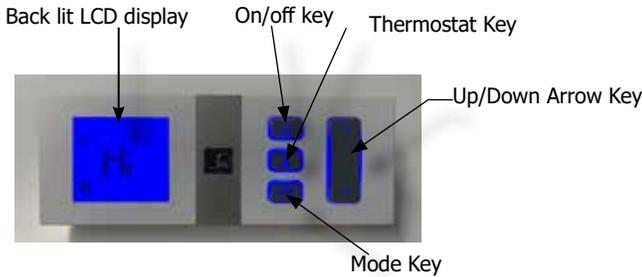
Figure 2: Proflame Transmitter
