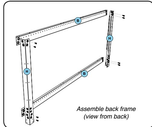
2. Install the frame assembled in Step 1, onto the back of the unit as shown with 2 screws on each side.
