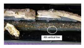
14. Install Log 8 - the left end of the log should sit 1" from the edge of the panel. The right end of Log 8 should be 2-1/2" from the right edge of the burner.
