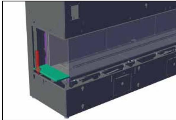
2. Install glass stopper (if desired) by sliding down the outside of the outer side panel.
