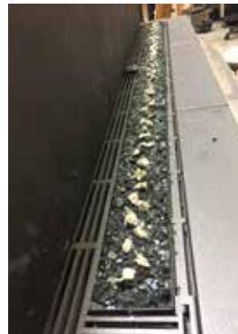
Burner covered with Fireglass and glowing wool
