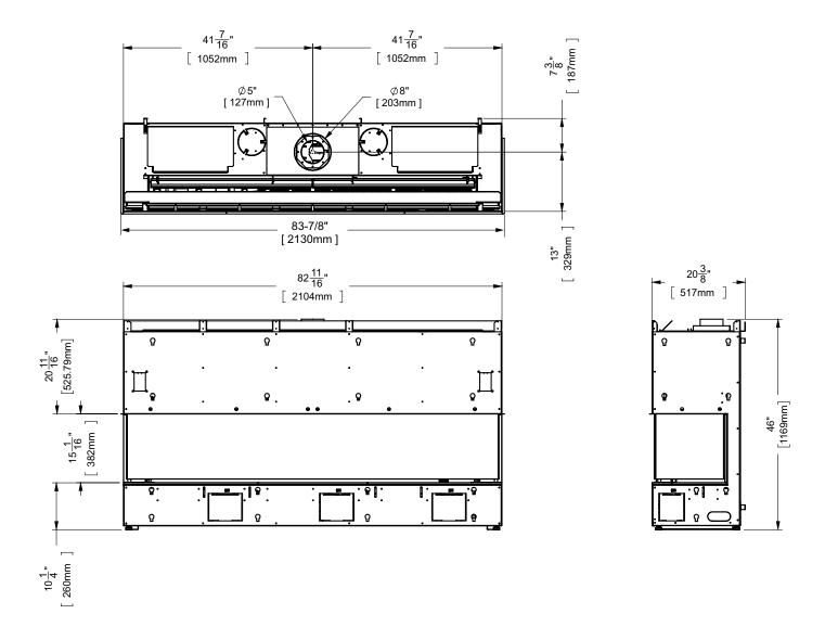
Note: Height Dimension is taken with leveling legs fully inserted and may vary depending on the height of the leveling legs, when unscrewed or extended.
