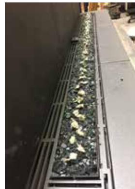
Burner covered with Fireglass and glowing wool
