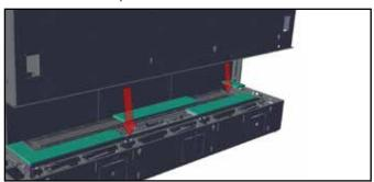
On back of firebox wall--install 6 screws (loosely) in locations shown below. Install 3 back panels--hang panels on installed screws through keyhole opening.
