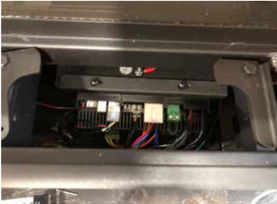
3. Locate the WiFi dongle connection (X0A) on the left side of the IFC.
