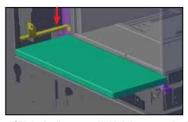
3. Slide backwall outer panel behind glass stopper bracket (if installed).
