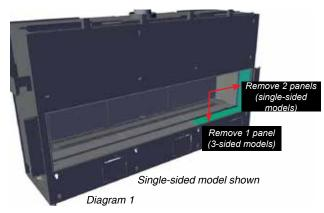
Remove access panel by lifting panel up and out (Diagram 2). Unscrew
