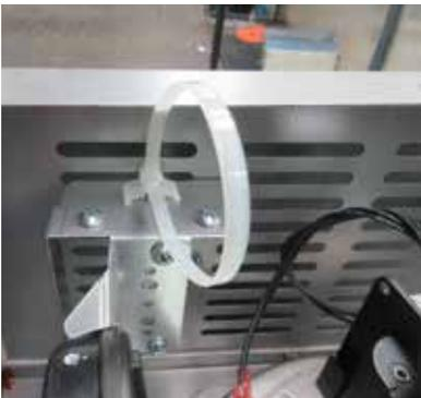
5. Connect ground wire to ground lug located on the side wall of the power vent box.
