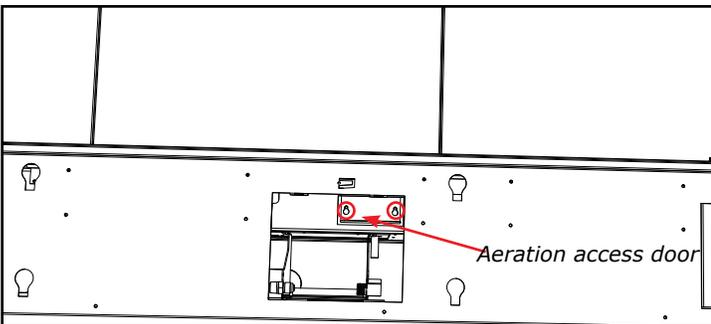
3. Attach the handle to the aeration lever through the access opening--handle will slide into position on the lever.
