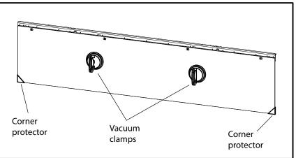
5. Holding the glass barrier in front of the unit, slide it up behind the top lip of the unit. Lift the barrier up as far as it goes, then hook the barrier onto the unit.
