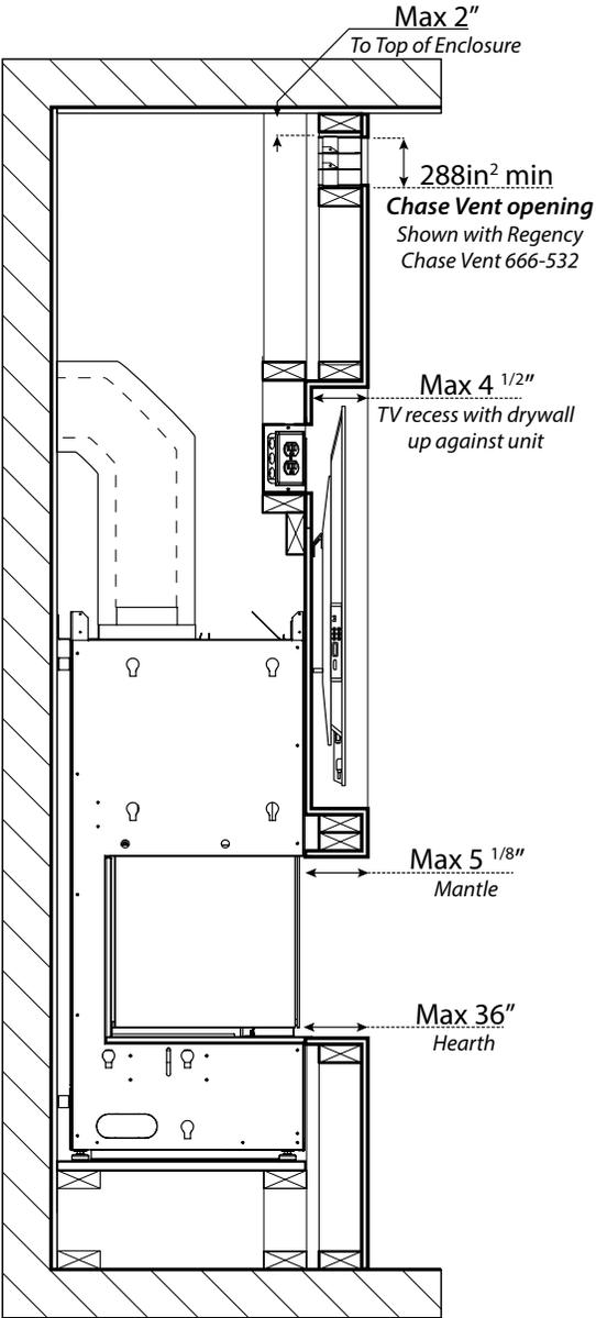
4 5/8" maximum TV recess using 1/2" drywall
