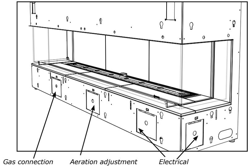
1. Identify access panel to be removed, remove corresponding outer trim panel by lifting up and off (centre panel shown below).
