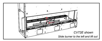
14. Remove burner orifice with a 3/8" wrench. Use another wrench to hold on to the elbow behind the orifice. Discard orifice. Reinstall new burner orifice LPG stamped #47 and tighten.
