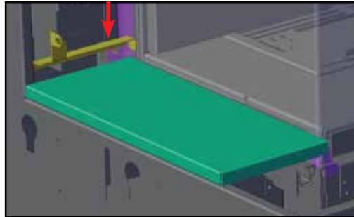
3. Slide backwall outer panel behind glass stopper bracket (if installed).
