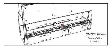
Remove pilot retainer clip with pliers and pull off the pilot cap to expose the pilot orifice.
