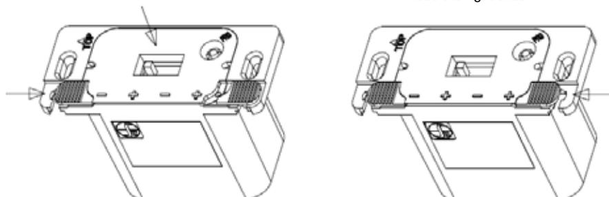
**STEP 4** Reinstall wall cover plate with 2 Phillips head screws.
