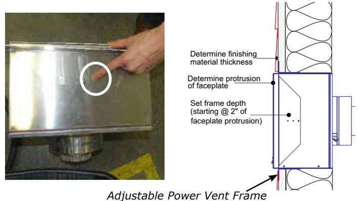
8. Install Power Vent unit into framed opening using 4 screws as shown below.
