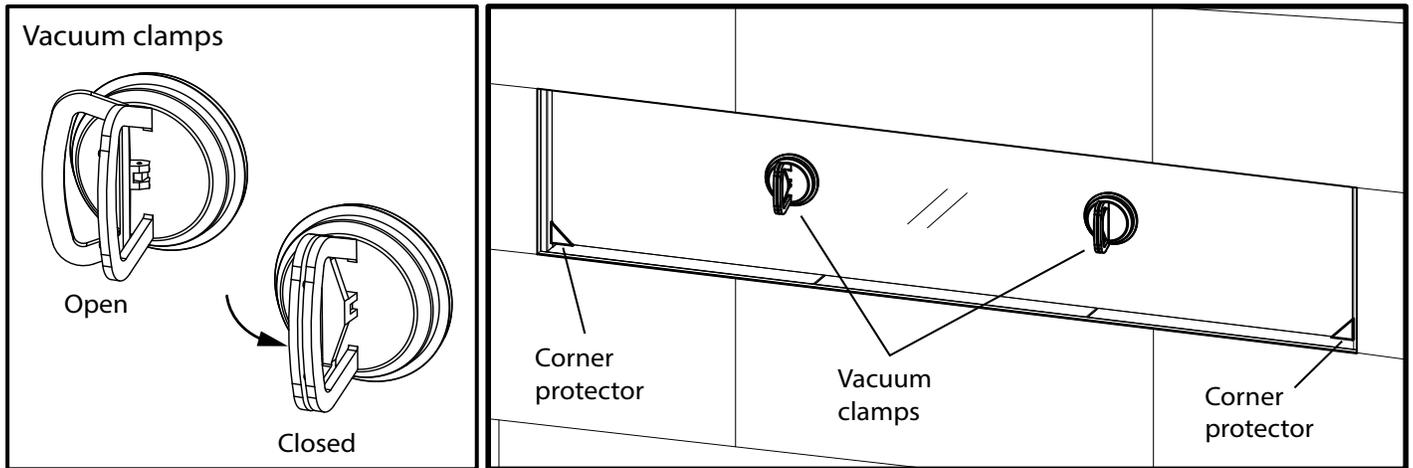
4. Using the vacuum clamps, lift the barrier straight up, pull it toward you, then gently lower it straight down (see below).
