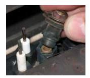
Unscrew the pilot orifice with the Allen key; then replace with the LPG pilot orifice and the pilot cap, provided in the kit.
