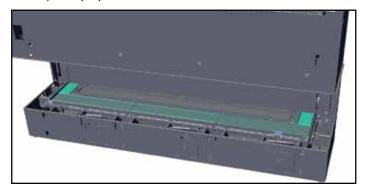
6. Install four back panel brackets in between the back wall and the burner tray. Line up the center of the middle brackets with the base panels installed in the previous step as shown below.
