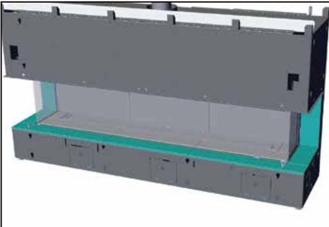
8. With panel set installed -- complete by installing barrier glass.
