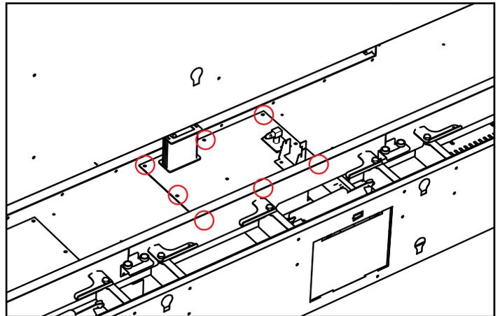
10. Lift valve tray out partially and disconnect flexible gas connection on the valve inlet side, remove valve tray- replace with new valve tray.
