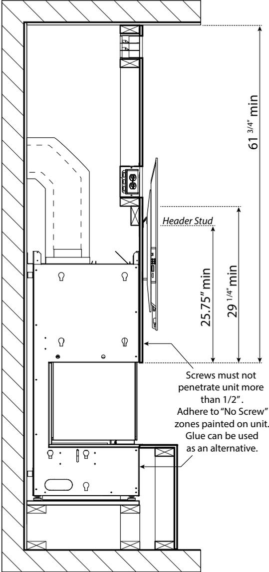
Flush wall TV install using 1/2" (13 mm) drywall.
