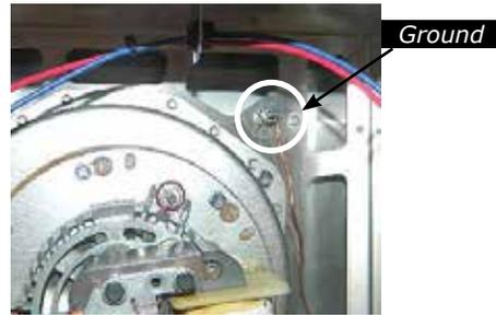
16. Connect wires from pressure switch to wires from BX cable--red to red and blue to blue. Cap paired wires with supplied marrette.
