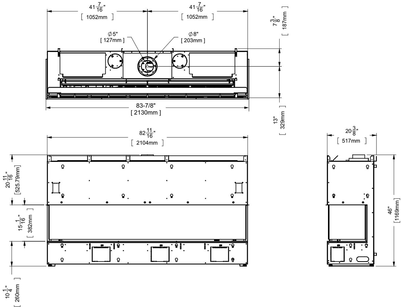
Note: Height Dimension is taken with leveling legs fully inserted and may vary depending on the height of the leveling legs, when unscrewed or extended.
