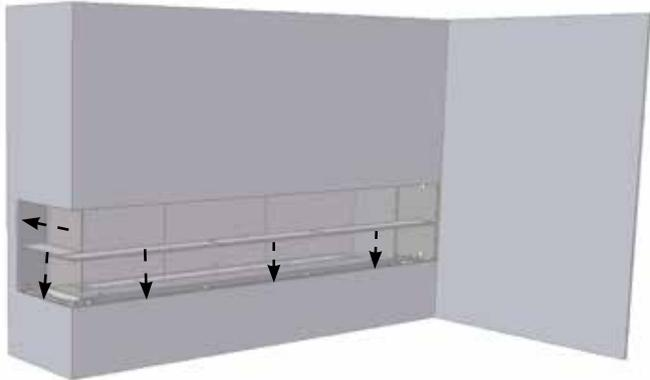
12. Once corner conversion is installed, continue regular install of barrier glass. Discard unused side glass barrier.
