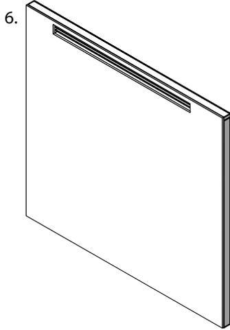
6. Cut hole in finishing material around inside of chase vent. Finish edges around opening
