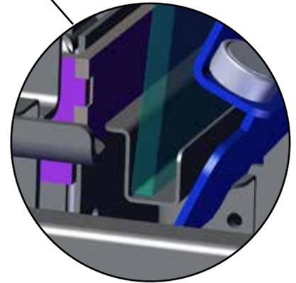
5. Tilt top of glass side panel outward to create clearance.
