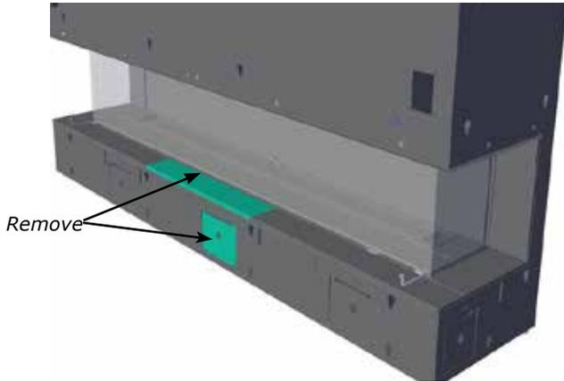
2. Loosen 2 screws on the aeration lever access door. Lift the door up and out to remove.
