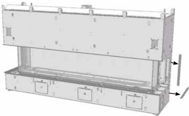
5. Slide outer side panel down onto screws that remain from removable trim. Tighten screws with offset screwdriver.
