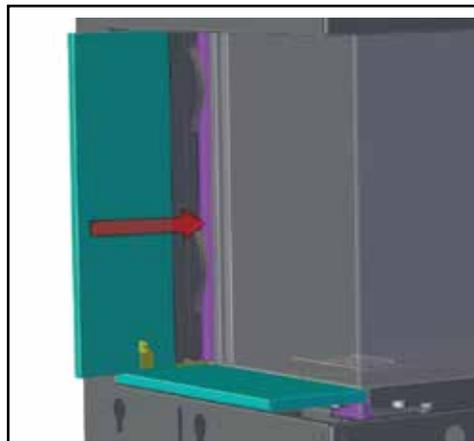
4. Install front end panel--place on unit as shown below.
