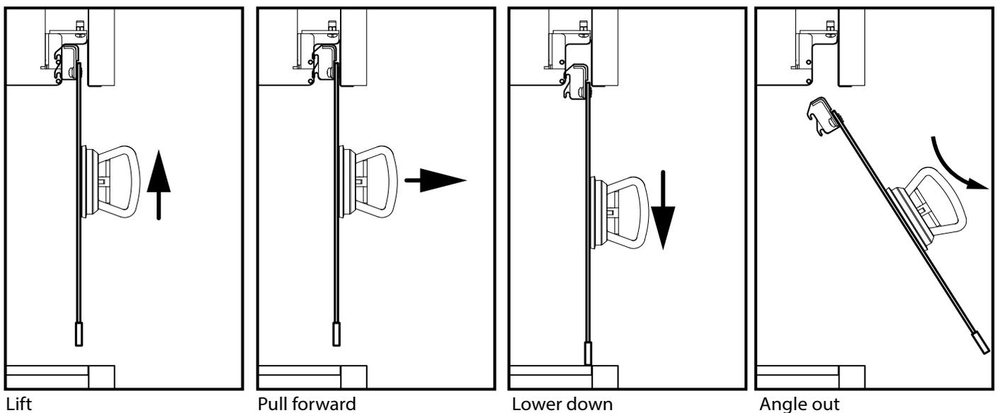
5. Angle the bottom edge toward you and carefully lift the glass barrier out, placing it on your prepared soft, scratch resistant surface (i.e. drop cloth).
