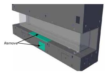
2. Loosen 2 screws on the aeration lever access door. Lift the door up and out to remove.
