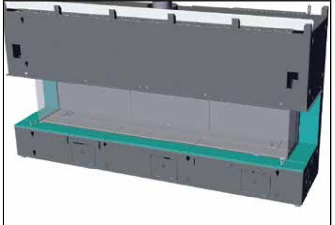
8. With panel set installed -- complete by installing barrier glass.
