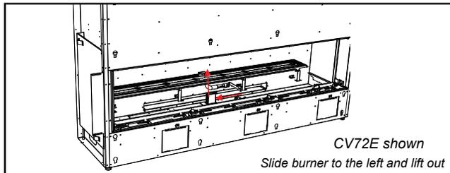
14. Remove burner orifice with a 3/8" wrench. Use another wrench to hold on to the elbow behind the orifice. Discard orifice. Reinstall new burner orifice LPG stamped #47 and tighten.
