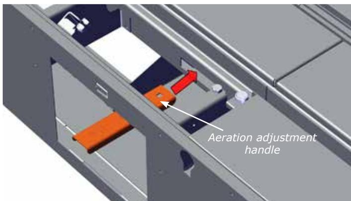
**NOTE:** The aeration handle is located near the right hand side of the gas valve access door -- attached by a magnet.
