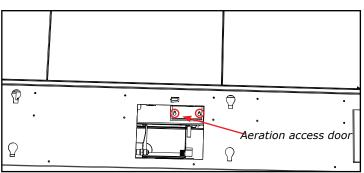
3. Attach the handle to the aeration lever through the access opening--handle will slide into position on the lever.
