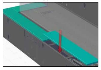
16. Install glass stopper (if desired) by sliding stopper assembly between unit and panel - the stopper assembly will attach to the unit via a magnet, adjust position of glass stopper is required.
