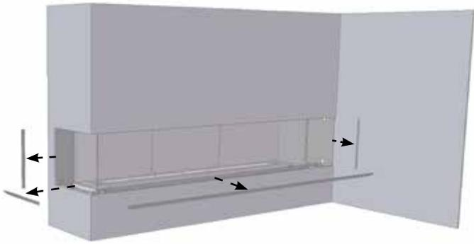
11. Slide corner piece up to outer side panel until contact with magnet is made.
