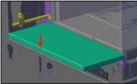
13. Slide backwall outer panel (13) behind glass stopper bracket (if installed).
