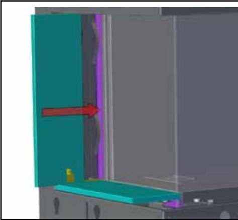
3. Install glass stopper (if desired) by sliding stopper assembly between unit and panel - the stopper assembly will attach to the unit via a magnet, adjust position of glass stopper is required.
