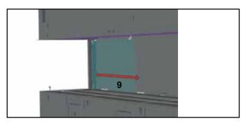
Secure the top of the panel brackets with 2 screws into 2 brackets (each panel has 2 brackets).
