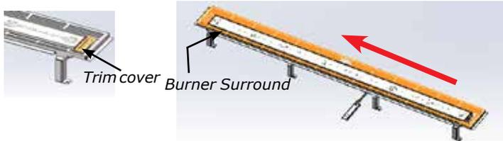
8. Loosen 8 screws in locations shown below (2 at front and 2 at rear)—slide burner to the left away from the orifice and lift out.
