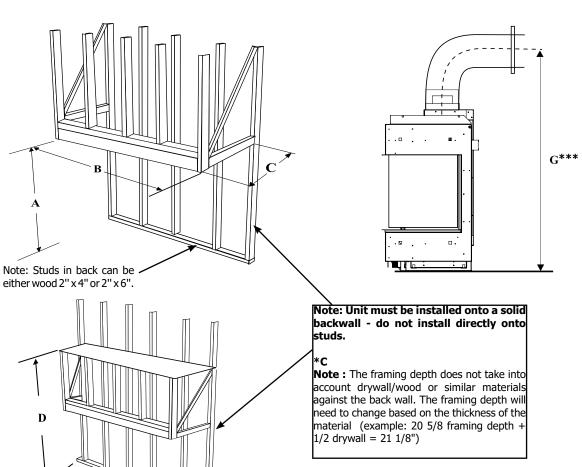
Note: This appliance must be installed on a solid surface such as a plywood floor which must be the full width and depth of the appliance.
