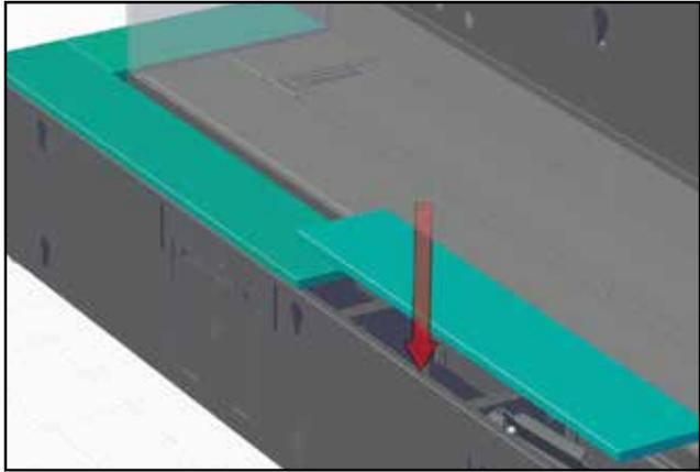
16. Install glass stopper (if desired) by sliding stopper assembly between unit and panel - the stopper assembly will attach to the unit via a magnet, adjust position of glass stopper is required.
