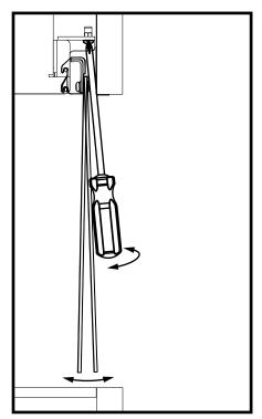
Slide the screwdriver straight up at the two indicator slots.
