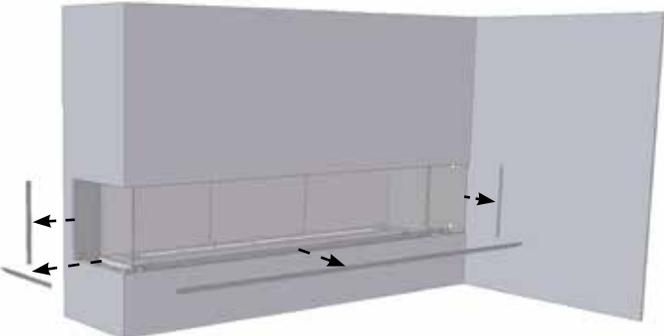
11. Slide corner piece up to outer side panel until contact with magnet is made.
