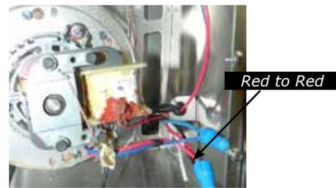
17. Connect remaining wires from the power vent motor to the BX cable- black to black and black to white. Cap paired wires with supplied marrette.
