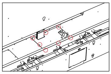
10. Lift valve tray out partially and disconnect flexible gas connection on the valve inlet side, remove valve tray- replace with new valve tray.
