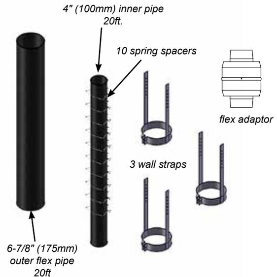
**NOTE** Power vent model only - the flex adaptor included with this kit is only required when joining two 946-756 flue extension kits to a maximum of 40 feet (12.9 m). If only one 946-756 20 foot (6.1 m) kit is used, the flex adaptor is not required.
