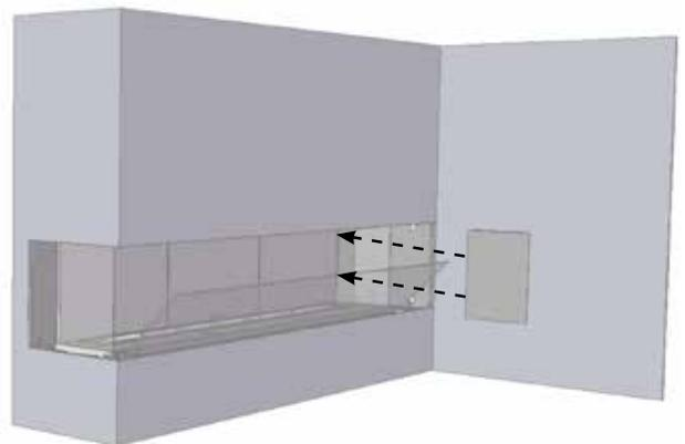
8. Once all framing and wall finishing is complete, use offset screwdriver and remove finishing trim guides.
