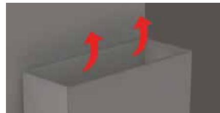
The ventilation opening may be placed on top ensuring it meets the 288 square inch opening. This type of ventilation opening would be used when the top of the enclosure is visible from above and where the ceiling within the room is higher than normal.
