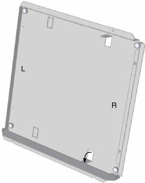
4. Loosen screws using offset screwdriver and remove trim guides from side of unit and recycle them.
