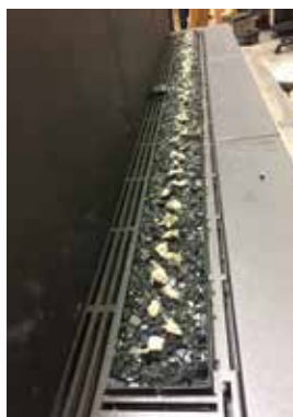
Burner covered with Fireglass and glowing wool
