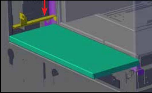
2. Slide backwall outer panel behind glass stopper bracket (if installed).
