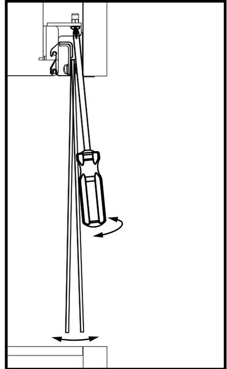
Slide the screwdriver straight up at the two indicator slots.
