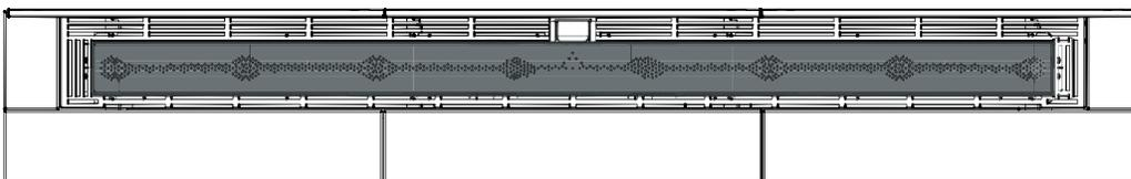
2. Install the 3.5 lb box of black charcoal glass and 1 lb of Andiron embers around the burner. Make sure the burner surround is only 50% covered.
