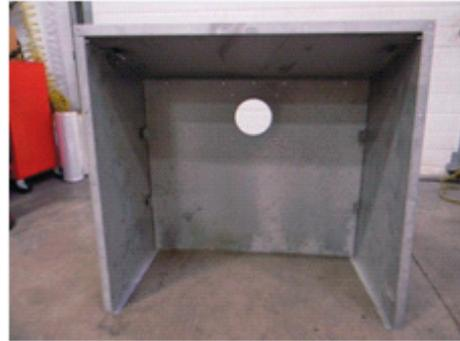
3. Attach the bottom to the sides with 3 screws on each side. Ensure return edge is on the inside.
