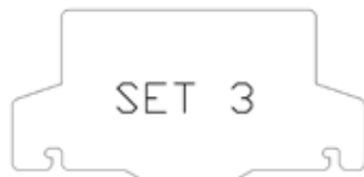
Restrictor plate for Set 3 (Part # 761-143F)
