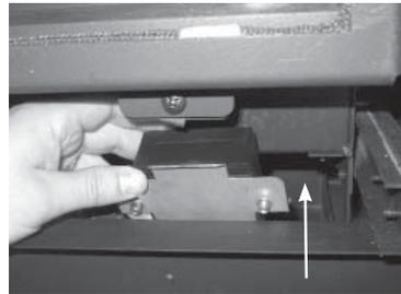
DC Spark Box mounting plate partially removed.
