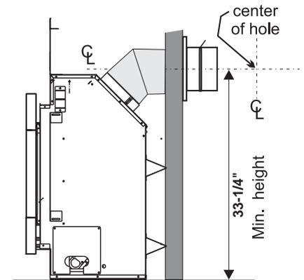
**IMPORTANT:** Do not locate termination hood where excessive snow or ice buildup may occur. Be sure to check vent termination area after snow falls, and clear to prevent accidental blockage of venting system. When using snow blowers, make sure snow is not directed towards vent termination area.
