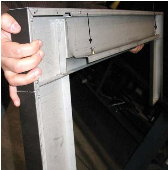
The bottom panel of the faceplate installs on the unit with 2 slides. These slides are located in the bottom of the unit - already installed within the outer slide. The inner slides need to be removed to install them on the brackets.
