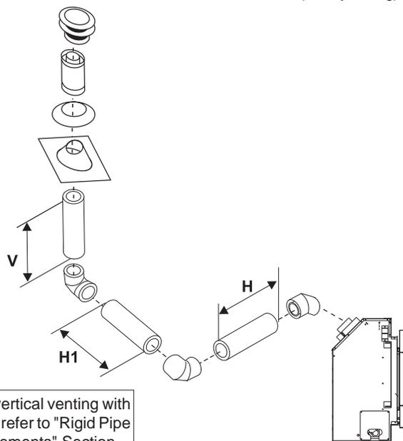
For additional vertical venting with 2 x 90° elbows, refer to "Rigid Pipe Venting Arrangements" Section.
