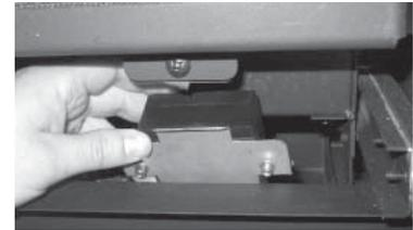
DC Spark Box mounting plate partially removed.
