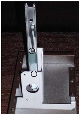
**HZ42ST** - install slider on this side of the bracket.
