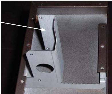
**HZ42** - Install slider with flat side facing outward -secure with 2 screws in locations shown.
