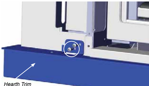
Diagram 3—Hearth Trim Secured to Backing Plate
