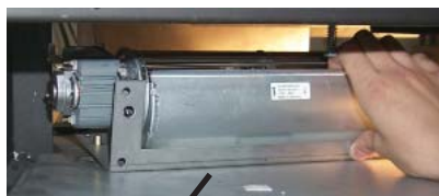
Position Fan B on mounting studs.
