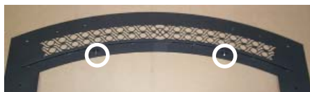
Remove screws from the mounting tabs.
