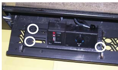
Secure left side with 2 screws and right side with one screw.
