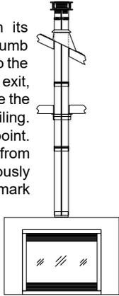
3. A Firestop spacer must be installed in the floor or ceiling of every level. To install the Firestop spacer in a flat ceiling or wall, cut a 10 inch square hole. Frame the hole as shown in Diagram 2 and install the firestop.
