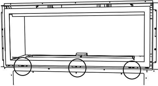
5. Remove the inner panels - reverse of "Inner panel Installation" in this manual.
