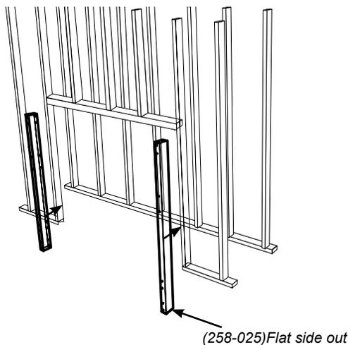
5. Secure horizontal steel header stud with 2 screws per side as per diagram.
