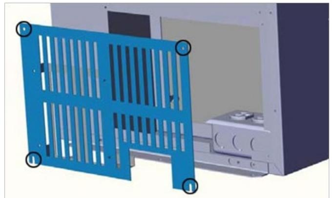
11. Install the fan control module (FCM) into the bracket on the side access panel. Plug in the power cord to the outlet in the unit. Reinstall the panel with the 4 screws from step 10.
