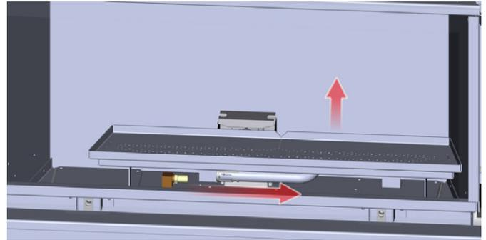
9. Remove the valve access plate by undoing the 8 screws - see locations below.
