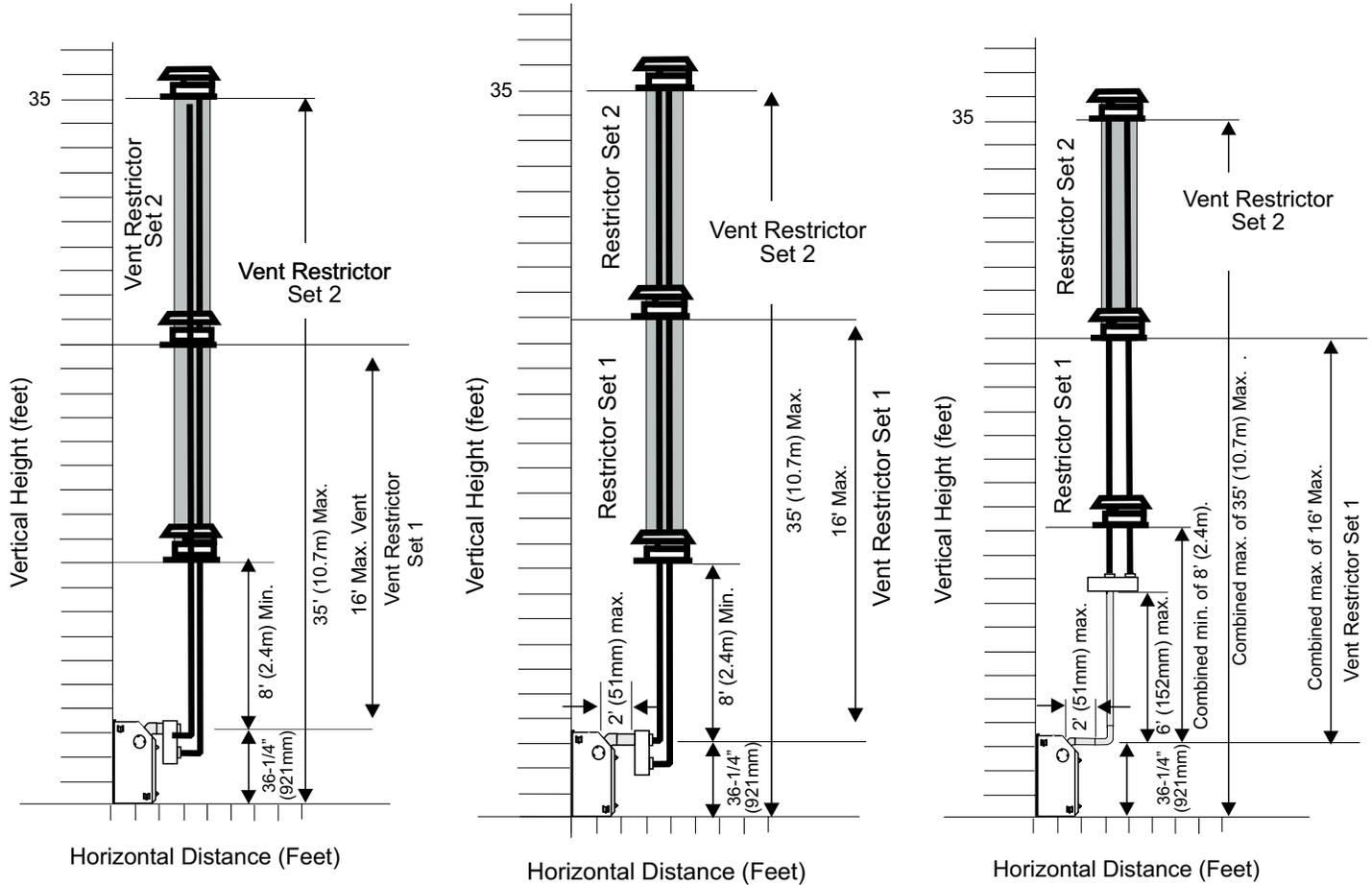
The shaded area in the diagrams show the allowable vertical terminations when using two-3" co-linear aluminium flex and 4 x 6-5/8" rigid pipe.
