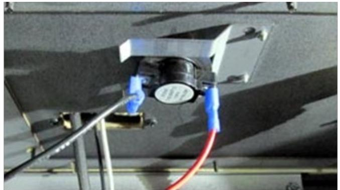
9. Secure the ground wire from the fan assembly and the power cord to the ground lug located on the back left near the fan.
