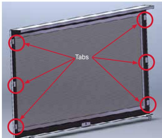
4. Hook the inner door frame (3) and safety screen assembly (2) over the inner door trim.
