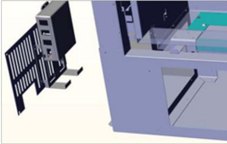
12. Plug in the fan power cord to the Fan Control Module into the outlet marked "Fan". Plug the FCM-COM wire from the remote control wiring harness into the location on the Fan Control Module marked "COM". Turn the switch on the Fan Control Module to the ON position. ON is to the left. The "O" is the off position
