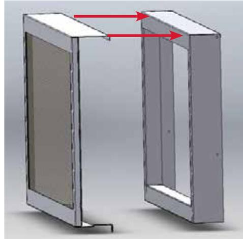
5. Bend the center tab up and secure with a screw to attach the inner door frame/safety screen assembly to the inner door trim
