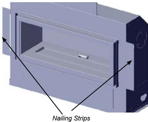
3. Adjust the nailing strips by loosening 2 screws on each nailing strip - adjust and retighten screws.
