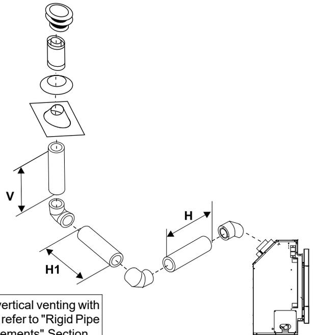
For additional vertical venting with 2 x 90° elbows, refer to "Rigid Pipe Venting Arrangements" Section.
