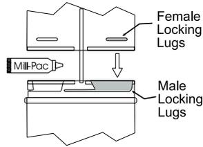
**NOTE: For best results and optimum performance with each approved venting system, it is highly recommended to apply "Mill-Pac" sealant (supplied) to every inner pipe connection. Failure to do so may result in drafting or performance issues not covered under warranty.**
