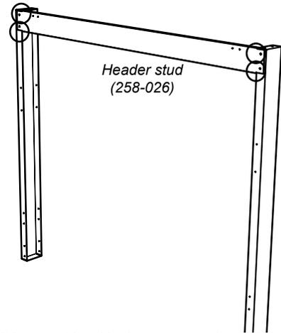
6. Slide the unit into position. Hook up gas, venting, electrical and fan (if purchased) prior to installing the remaining steel studs.
