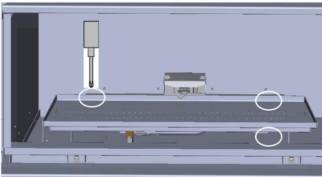
8. Remove the burner by sliding it to the right - then lift out.
