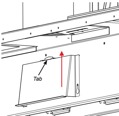
5. Loosen 2 screws on each side of individual inner light cover and remove.
