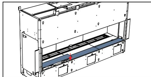
8. Slide the glass barrier stopper bracket in between the front panel and the unit wall as shown.
