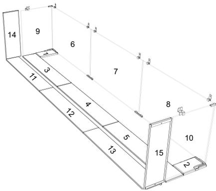
3. Install back corner panels (1, 2) - seat smallest panel in back left corner, repeat on other side.
