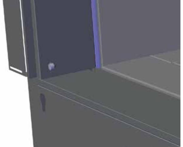
2. Slide the stopper bracket in between the front panel and the unit wall as shown.
