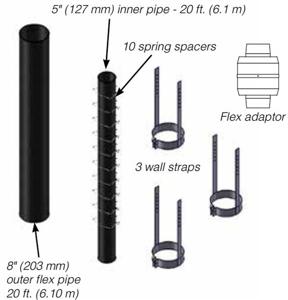
**NOTE** If an offset is necessary in the attic or floor joists it is important to support the vent pipe every 3 ft. (0.91 m) to avoid excessive stress and sagging of the vent pipe. Wall straps are provided (3 in total) for this purpose.
