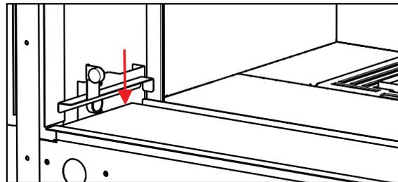
9. Install side outer panels by manoeuvring the bracket between the wall and the barrier stopper bracket as shown below. The panels are held in place by magnets.
