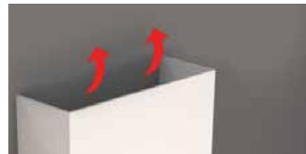
The ventilation opening may be placed on top ensuring it meets the 288 square inch opening. This type of ventilation opening would be used when the top of the enclosure is visible from above and where the ceiling within the room is higher than normal.
