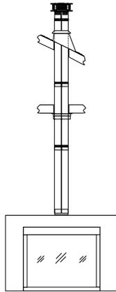
**2)** Set the gas appliance in its desired location. Drop a plumb bob down from the ceiling to the position of the appliance flue exit, and mark the location where the vent will penetrate the ceiling. Drill a small hole at this point. Next, drop a plumb bob from the roof to the hole previously drilled in the ceiling, and mark the spot where the vent will penetrate the roof.
