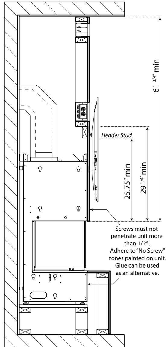
Flush wall TV install using 1/2" (13 mm) drywall.
