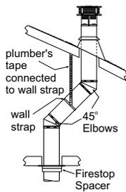
Determine if ceiling joists, roof rafters or other framing will obstruct the venting system. You may wish to relocate the appliance or to offset, as shown in Diagram 2 to avoid cutting load bearing members.
