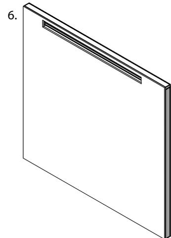
Cut hole in finishing material
