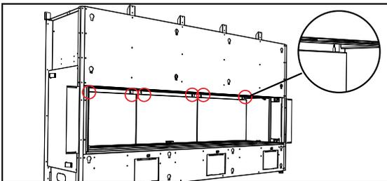
3. Install panel bracket into the slot in the panel.
