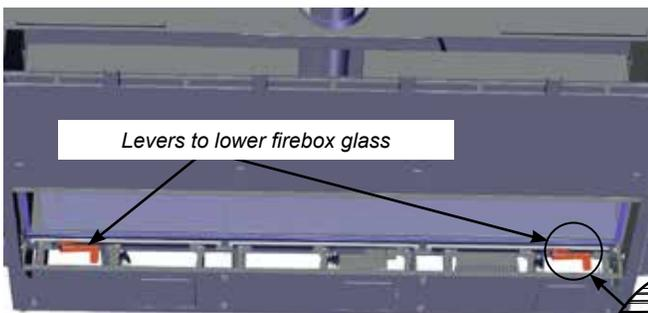
9. **To remove the firebox glass panel from the unit:** tilt the glass forward gently onto the glass supports, grip both suction clamps and lift the glass up and out of the unit.
