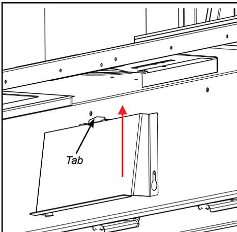
5. Loosen 2 screws on each side of individual inner light cover and remove.
