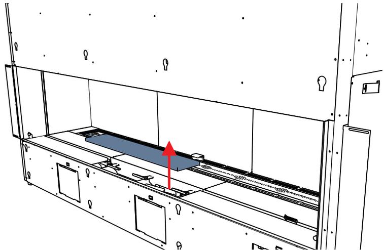
2. From inside the unit--push in tab to release the access panel at the top.
