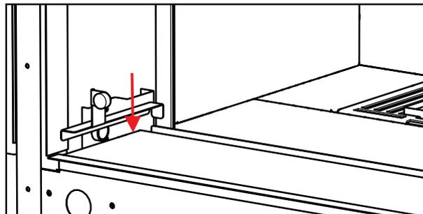
3. Install side outer panels by manoeuvring the panel between the wall and the barrier stopper bracket as shown below. The panels are held in place by magnets.
