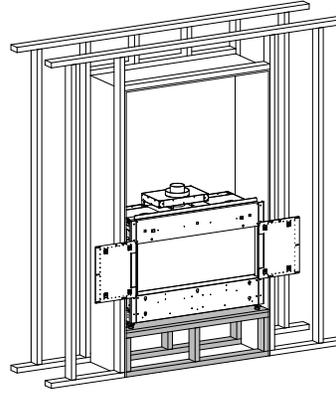
2. Locate mounting holes in locations shown below and remove nailing strips (if already installed). Remove drywall finishing edge from right and left side of window opening, using supplied right-angle screwdriver.
