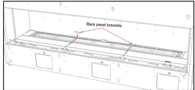
7. Carefully manoeuvre the back glass panels (6,7,8) to the back wall of the firebox. Start with back panel 6 -- place two panel brackets on each panel and manoeuvre into position, sliding the bottom into the corner and back brackets.
