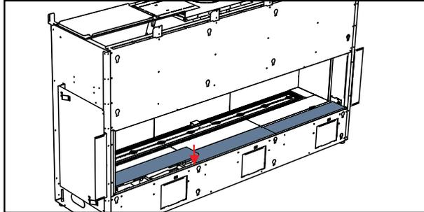
2. Slide the glass barrier stopper bracket in between the front panel and the unit wall as shown.
