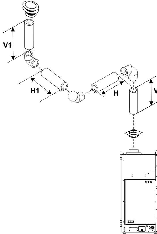
**Venting Arrangement for Vertical Terminations - Straight Vertical Venting and/or with a Max. of Two (2) 90° Elbows (1 - 90° = 2 - 45°)**
