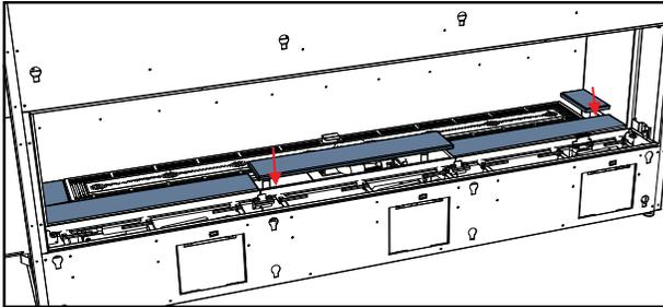
2. On back of firebox wall--install 6 screws (loosely) in locations shown below. Install 3 back panels--hang panels on installed screws through keyhole opening.
