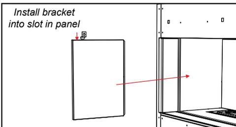
5. Secure panel in position with one screw.
