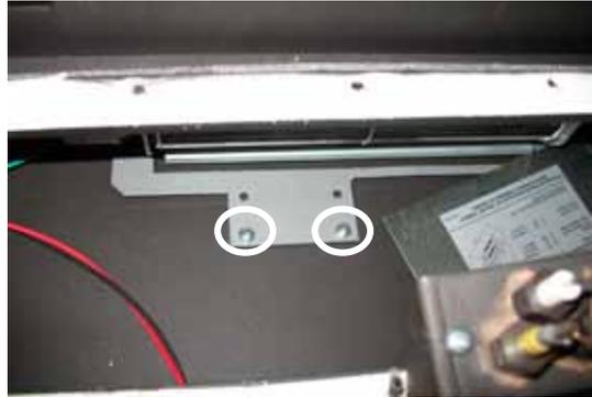
10) Remove the 2 screws that hold the pilot assembly in place and lift forward as shown below.
