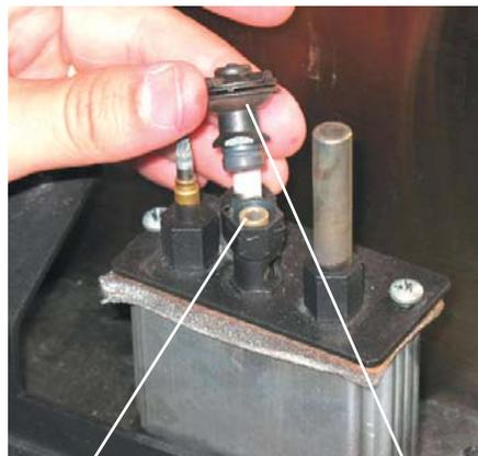
Pilot Orifice Schéma 5 Pilot Cap
