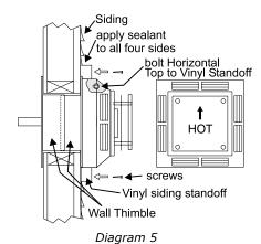
Note: If installing termination on a siding covered wall, a vinyl siding standoff or furring strips must be used to ensure that the termination is not recessed into the siding. The four wood screws provided should be replaced with appropriate fasteners for stucco, brick, concrete, or other types of sidings.
