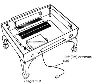
Run the extension cord through the largest opening at the back when using the Bottom Heat Shield with Legs option-no strain relief grommet required.
