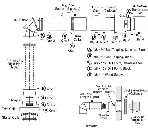
Note: The four screws provided for the vent cap should be replaced with appropriate fasteners for stucco, brick, concrete, or other types of sidings.
