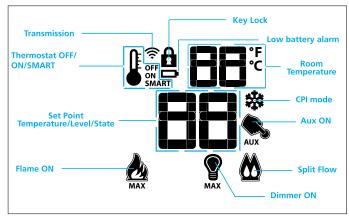
Figure 2: Transmitter LCD Display
