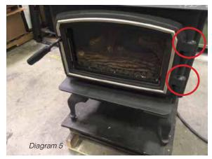
Note: The bottom of the door may scrape the ash lip. In this case place the spacers provided on the door hinges of the unit before placing the door.
