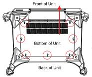
Diagram 2 Loosen 6 screws-slide access panel to the front of unit to remove
