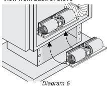
9. Slide thermodisc under the thermodisc bracket.
