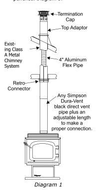
7. The connection between the appliance and the Retro Connector may be completed with sections of black direct vent pipe, together with an adjustable length.
