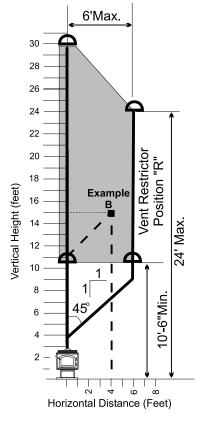
Straight Vertical and Offset to Vertical Terminations use Vent Restrictor Position "R" (Right)
