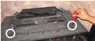
Diagram 1: Remove the left and right screws.
