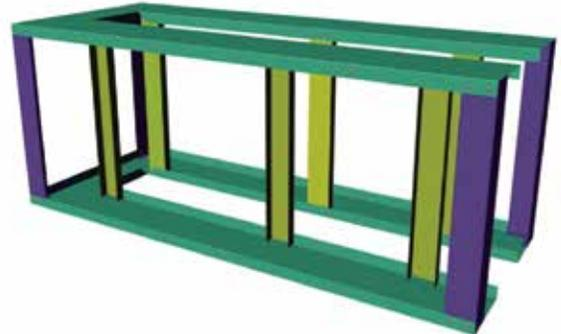
Diagram 5 - Install Inside vertical supports
