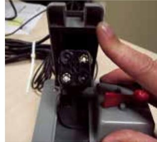
7. Using silicone, completely seal strain relief to protect from water or moisture.
