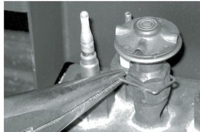
6. Pull off the pilot cap to expose the pilot orifice. Using a 5/32" allen key, remove pilot orifice and replace with LP pilot orifice.
