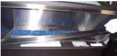
10. HZO42/HZO60--Remove the burner tray by lifting up and out.
