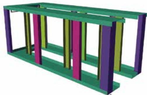
Diagram 7 - Install outside vertical supports (B1) with 4 screws each
