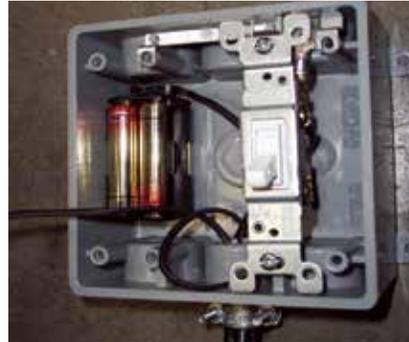
7. Install 4- AA batteries into each battery terminal. Ensure correct polarity. Slide the first battery terminal all the way to the right - until it is next to the switch. The 2nd battery terminal can be attached to the battery cover with the supplied velcro.
