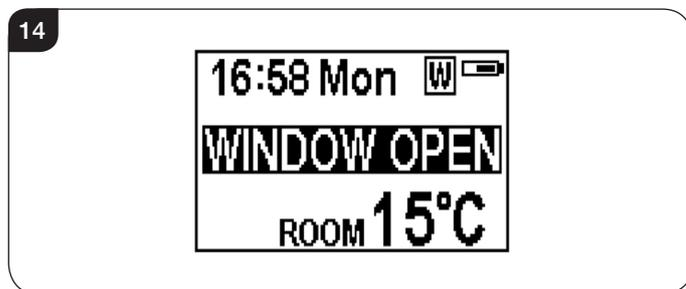
2b.45 After indoor temperature rise or manual intervention (by operating remote control), it will return to normal working state.
