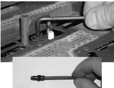
12. Remove burner orifice with a 1/2" wrench while using a 9/16" wrench to hold onto the elbow behind the orifice, then discard the orifice.
