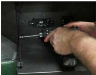
6. Remove four screws to remove the access panel (in locations shown below) and the chain attached to the front door and the unit.
