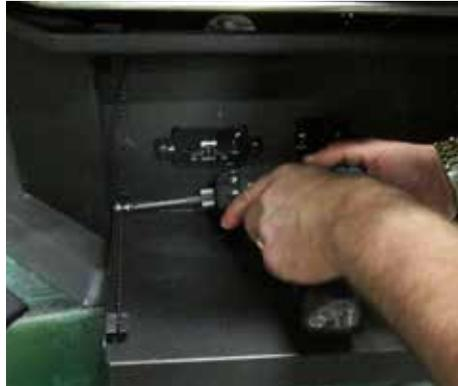
3. Remove four screws and the chain attached to the front door and the unit.
