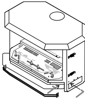
To adjust the aeration: use the allen key to turn the turning gear which will adjust the air shutter. Open the air shutter for a blue flame or close it for a yellow flame.
