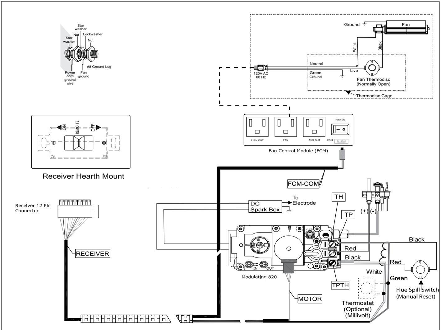
**CAUTION:** Label all wires prior to disconnection when servicing controls. Wiring errors can cause improper and dangerous operation.
