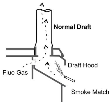
The smoke should be drawn into the draft hood. If the smoke is not drawn into the draft hood, turn the unit off and check for the cause of lack of draft.
